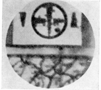
Fig. 57—Enlargement of 1/2-millimeter test-pattern circle at corner of plate (Figure 55) at 0 = 19 degrees.
