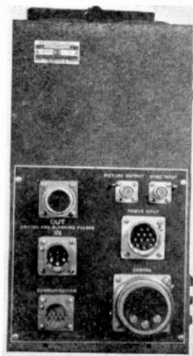
Fig. 11 — Rear of camera control.
