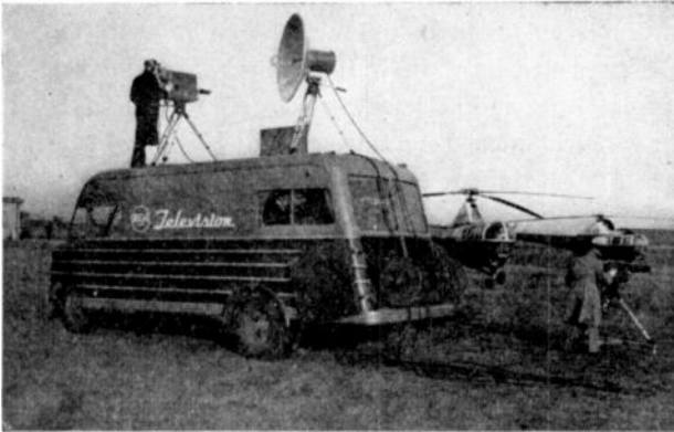
Fig. 4 — Mobile unit in operation, with camera and relay transmitter on the roof.
