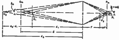
Fig. 64—Relations between lens diameter, circle of confusion, and depth of field for finite distances d_1 and d_2 .
