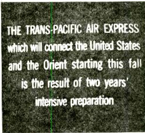
Fig. 10—Television picture transmitted by an Orthicon.
