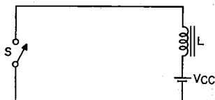
Fig. 85—Simplest form of deflection circuit.
