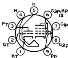
Miniature type used in color and black-and-white television receivers employing series-connected heater strings. The pentode unit is used as a video output amplifier; the triode unit is used in sync-separator, sync-clipper, and phase-inverter circuits. Outline 14, OUTLINES SECTION. Heater volts (ac/dc), 8; amperes, 0.6; warm-up time (average), 11 seconds. Except for heater rating, this type is identical with miniature type 6EB8.
