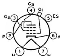
Glass type used as detector or amplifier in radio receivers. Outline 45, OUTLINES SECTION. Heater volts (ac/dc), 6.3; amperes, 0.3. For electrical characteristics, refer to type 6J7. Type 6D7 is a DISCONTINUED type listed for reference only.
