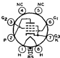
Glass lock-in type used in output stage of ac/dc receivers. Outline 20, OUTLINES SECTION. Tube requires lock-in socket. Heater volts (ac/dc), 35; amperes, 0.15. For maximum ratings and typical operation, refer to glass octal type 35L6-GT. Type 35A5 is used principally for renewal purposes.
