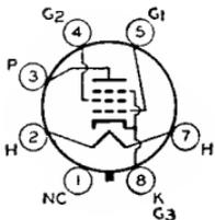
Glass octal type used in output stage of ac/dc receivers. Outline 42, OUTLINES SECTION. Heater volts (ac/dc), 25; amperes, 0.3. Typical operation as class A<sub>1</sub> amplifier: plate volts, 200 max; grid-No.2 volts, 135 max; grid-No.1 volts, -23; plate ma., 62; grid-No.2 ma., 1.8; plate resistance, 18000 ohms; transconductance, 5000 μmhos; load resistance, 2500 ohms; output watts, 7.1. This is a DISCONTINUED type listed for reference only.
