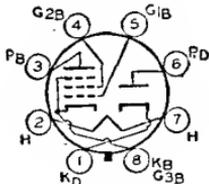
Glass octal type used as combined half-wave rectifier and output amplifier in ac/dc receivers. Outline 23, OUTLINES SECTION. Tube requires octal socket. Heater volts (ac/dc), 32.5; amperes, 0.3. Maximum ratings for rectifier unit: ac plate volts (rms), 125; dc output ma., 60. Typical operation of beam power unit as class A<sub>1</sub> amplifier: plate and grid-No.2 volts,
