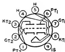
driver for the other unit. Outline 12, OUTLINES SECTION. Tube requires nine-contact socket and may be mounted in any position.
