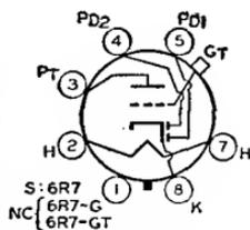
watts. For typical operation as a resistance-coupled amplifier, refer to Chart 7, RESISTANCE-COUPLED AMPLIFIER SECTION. Types 6R7-G and 6R7-GT are DISCONTINUED types listed for reference only. Type 6R7 is used principally for renewal purposes.
