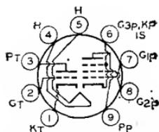
Miniature type used in a wide variety of applications in television receivers. This type has a controlled heater warm-up time for use in receivers employing series-connected
