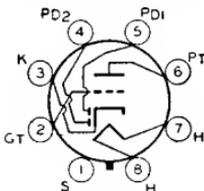
Metal type used as combined detector, amplifier, and avc tube in radio receivers. Except for heater-current rating and interelectrode capacitances, this type is essentially the same electrically as type 6AT6. Outline 3, OUTLINES SECTION. Tube requires octal socket. Heater volts (ac/dc), 6.3; amperes, 0.15. For diode operation curves, refer to type 6AV6. Type 6SZ7 is a DISCONTINUED type listed for reference only.
