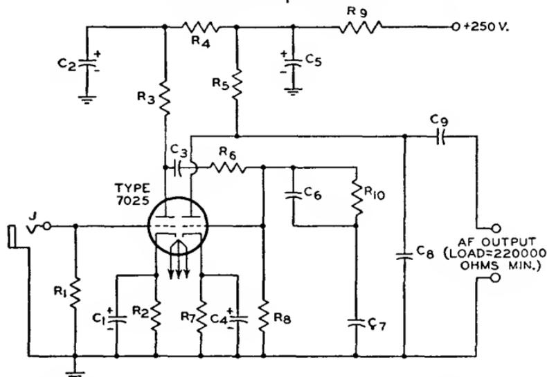
$C_1 C_4=25 \mu\text{f}$ , electrolytic, 25 v.
