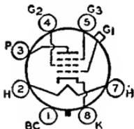
Glass octal type used as biased detector or high-gain audio amplifier in ac/dc radio receivers. Outline 23, OUTLINES SECTION. Heater volts (ac/dc), 12.6; amperes, 0.15. Except for heater rating, this type is identical with glass-octal type 6J7-GT. Type 12J7-GT is used principally for renewal purposes.
