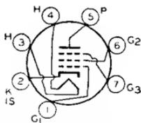
warm-up time (average), 11 seconds. Except for heater rating, this type is identical with miniature type 6DT6.
