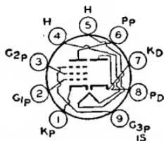
detector or dc restorer. Outline 12, OUTLINES SECTION. Heater volts (ac/dc), 4.7; amperes, 0.6; warm-up time (average), 11 seconds. Except for heater rating, this type is identical with miniature type 6AM8-A.
