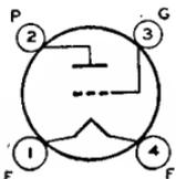
Glass type used as output amplifier in dry-battery-operated receivers. Filament volts (dc), 3.3; amperes, 0.132. Characteristics as class A<sub>1</sub> amplifier: plate volts, 135 max; grid volts, -22.5; plate ma., 6.5; plate resistance, 6300 ohms; amplification factor, 3.3; transconductance, 525 μmhos; load resistance, 6500 ohms; output mw., 110. This is a DISCONTINUED type listed for reference only.
