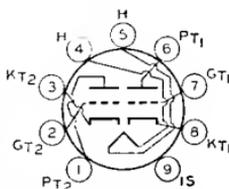
Heater volts (ac/dc), 4.2; amperes, 0.6; warm-up time (average), 11 seconds. Except for heater rating, this type is identical with miniature type 6BC8.
