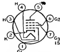
OUTLINES SECTION. Heater volts (ac/dc), 4.2; amperes, 0.6; warm-up time (average), 11 seconds. Except for heater rating, this type is identical with miniature type 6EW6.
