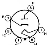
Glass octal type used as damper tube in horizontal-deflection circuits of television receivers. Outline 22, OUTLINES SECTION. Tube requires octal socket and may be mounted in any position. May be supplied with pin No.1 omitted. Socket terminals 1, 2, 4, and 6 should not be used as tie points. It is important that this tube, like other power-handling tubes, be adequately ventilated.
