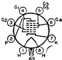
Glass lock-in type used as frequency converter in superheterodyne circuits. Outline 15, OUTLINES SECTION. Tube requires lock-in socket. Heater volts (ac/dc), 6.3; amperes, 0.3. Except for interelectrode capacitances, this type is the same electrically as metal type 6A8. Type 7B8 is used principally for renewal purposes.
