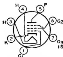
in vhf television tuners. Outline 11, OUTLINES SECTION. Heater volts (ac/dc), 4.2; amperes, 0.45; warm-up time (average), 11 seconds. Except for heater rating, this tube is identical with miniature type 6DE6.
