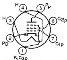
Miniature type used as combined detector and audio amplifier in automobile and ac-operated radio receivers. The diode unit is used as an AM detector, and the pentode unit as an
