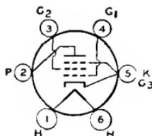
Glass type used in audio output stage of ac receivers. Outline 43, OUTLINES SECTION. Tube requires six-contact socket. Heater volts (ac/dc), 6.3; amperes, 0.7. This type is electrically identical with type 6F6. Type 42 is used principally for renewal purposes.
