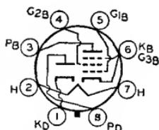
plate-supply impedance, 15 ohms. Typical operation and maximum ratings of beam power unit as class A<sub>1</sub> amplifier: plate and grid-No.2 volts, 110 (117 *max*); grid-No.1 volts, -7.5; plate ma., 40; grid-No.2 ma., 3; plate resistance, 15000 ohms; transconductance, 7500  $\mu$ mhos; load resistance, 2000 ohms; output watts, 1.8; plate dissipation, 5 *max* watts; grid-No.2 input, 1 *max* watt. This type is used principally for renewal purposes.
