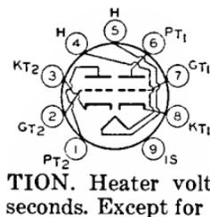
Miniature type used as combined vertical deflection and horizontal deflection oscillator in television receivers employing series-connected heater strings. Outline 14, OUTLINES SECTION. Heater volts (ac/dc), 8.4; amperes, 0.45; warm-up time (average), 11 seconds. Except for heater rating, this type is identical with miniature type 6CG7.
