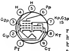
Miniature type used in television receivers employing series-connected heater strings. Tube is used as combined oscillator and mixer tube in vhf tuners of television receivers utilizing
