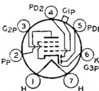
Glass types used as combined detector, amplifier, and avc tubes. Outline 40, OUTLINES SECTION. These types fit the small seven-contact (0.75-inch, pin-circle diameter) socket. Except for interelectrode capacitances, the electrical characteristics of the 6B7 are identical with those of type 6B8-G. Type 6B7S has the external shield connected to the cathode. In
