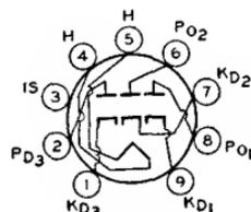
Tube requires miniature nine-contact socket and may be mounted in any position.
