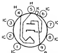
Miniature type used as a damper tube in horizontal deflection circuits of television receivers. Outline 17, OUTLINES SECTION, except all vertical dimensions of this type are 1/8 inch greater. Tube requires miniature nine-contact socket and may be mounted in any position. Socket terminals 1, 2, 3, 6, 7, and 8 should not be used as tie points. It is especially important that this tube, like other power-handling tubes, be adequately ventilated.
