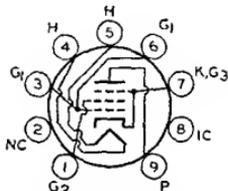
and operating at ulior voltages up to 18 kilovolts. Also used in the audio output stage of television and radio receivers. This type has a controlled heater warm-up time for use in receivers employing series-connected heater strings. Outline 18, OUTLINES SECTION. Tube requires miniature nine-contact socket and may be mounted in any position.
