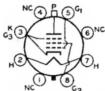
Glass octal types used as output amplifier in horizontal-deflection circuits of television equipment and other applications where high pulse voltages occur during short duty cycles. Out-
