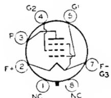
Glass octal type used in output stage of battery-operated receivers. Outline 42, OUTLINES SECTION. Tube requires octal socket. Filament volts (dc), 2.0; amperes, 0.12. Typical operation as class A<sub>1</sub> amplifier: plate and grid-No.2 (screen-grid) volts, 135 (180 *max*); grid-No.1 volts, -4.5; plate ma., 8; grid-No.2 ma., 2.4; cathode resistor, 432 ohms; output watts, 0.31. This is a DISCONTINUED type listed for reference only.
