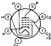
Heater volts (ac/dc), 3.15; amperes, 0.6; warm-up time (average), 11 seconds. Peak heater-cathode volts when heater is negative with respect to cathode, 300 max (the dc component must not exceed 200 volts). Except for heater and heater-cathode ratings, this type is identical with miniature type 6BZ6.
