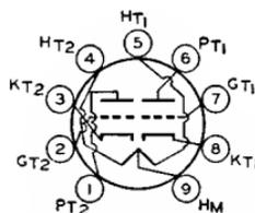
heater warm-up time for use in series-connected heater strings. These types are also used in other applications including phase-inverter circuits and multivibrator circuits. Outline 14, OUTLINES SECTION. Tubes require miniature nine-contact socket and may be mounted in any position. Each triode unit is independent of the other except for the common heater. Type 12BH7 is a DISCONTINUED type listed for reference only.
