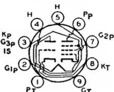
a reactance tube. The triode unit is used in sweep-oscillator, sync-separator, sync-clipper, and phase-splitter circuits. Outline 12, OUTLINES SECTION. Heater volts (ac/dc), 4.7; amperes, 0.6. Except for heater rating, this type is identical with miniature type 6CM8.
