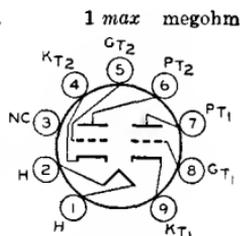
in microphone amplifiers and in preamplifiers for mono- and stereophonic phonographs. Outline 12, **OUTLINES SECTION**. Tube requires miniature nine-contact socket and may be mounted in any position. For typical operation as a resistance-coupled amplifier, refer to Chart 7, **RESISTANCE-COUPLED AMPLIFIER SECTION**.
