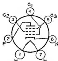
plate resistance, 2300 ohms; amplification factor, 6; transconductance, 2600; load resistance for maximum undistorted power output, 5000 ohms; undistorted output watts, 1.25. For typical operation as class A<sub>1</sub> amplifier (pentode connection; grid No.3 tied to cathode at socket), refer to type 6F6 with plate voltage of 250 volts. Type 59 is a DISCONTINUED type listed for reference only.
