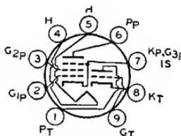
SECTION. Tube requires miniature nine-contact socket and may be mounted in any position.
