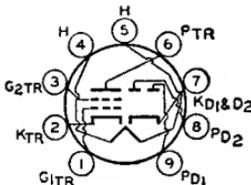
Miniature type used as combined detector and audio driver in automobile radio receivers operating from a 12-volt storage battery. Outline 12, OUTLINES SECTION. Tube requires miniature nine-contact socket and may be mounted in any position.
