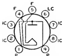
Miniature type used in high-voltage, low-current applications such as the rectifier in high-voltage, pulse-operated voltage-doubling power supplies for kinescopes. The very low power
