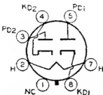
Glass octal type used as half-wave rectifier or voltage doubler in ac/dc receivers. This type is used particularly in "transformerless" receivers of either the ac/dc type or the voltage-doubler type. Outline 22, OUTLINES
