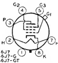
SECTION. Type 6J7-GT is used principally for renewal purposes. Type 6J7-G is a DISCONTINUED type listed for reference only. All types require octal socket and may be mounted in any position.
