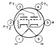
Glass type used as class A<sub>1</sub> power amplifier. One triode, the driver, is directly connected within the tube to the second, or output, triode. Outline 43, OUTLINES SECTION. Tube requires six-contact socket. Heater volts (ac/dc), 6.3; amperes, 0.8. Characteristics of input and output triodes as class A<sub>1</sub> amplifier follow. Input triode: plate volts, 300 *max*; grid volts, 0; plate
