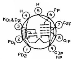
or reactance tube. The diode unit is used in automatic-frequency-control and detector circuits. Outline 12, OUTLINES SECTION. Tube requires miniature nine-contact socket and may be mounted in any position.
