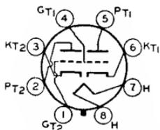
Glass octal type containing high-mu triode and high-perveance, low-mu triode in same envelope. Used as combined vertical-deflection amplifier and vertical-deflection oscillator in television receivers employing picture tubes having 110-degree deflection angles and high ultor voltages. Outline 19, OUTLINES SECTION. Tube requires octal socket and may be mounted in any position.
