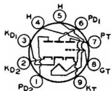
ploying series-connected heater strings. The triode unit is used in burst-amplifier, af amplifier, and low-frequency oscillator applications. The diode units are used in phase-detector, ratio-detector or discriminator, and horizontal AFC discriminator circuits. Outline 14, OUTLINES SECTION. Tube requires miniature nine-contact socket and may be mounted in any position.
