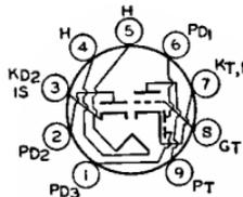
Miniature type used as combined AM detector, FM detector, and af voltage amplifier in radio and television receivers employing series-connected heater strings. Outline 12,
