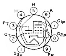
Heater volts (ac/dc), 4.7; amperes, 0.6; warm-up time (average), 11 seconds. Except for heater rating, this type is identical with miniature type 6X8.
