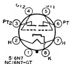
as a class B amplifier. Outlines 6 and 22, respectively, OUTLINES SECTION. Tubes require octal socket and may be mounted in any position. For class B amplifier considerations, refer to ELECTRON TUBE APPLICATIONS SECTION. Type 6N7 is used principally for renewal purposes.
