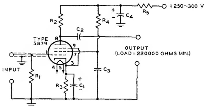
$C_1=25 \mu\text{f}$ , electrolytic, 25 v.
