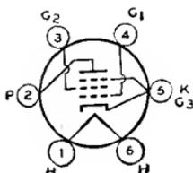
Glass type used in audio output stage of ac/dc receivers. Outline 43, OUTLINES SECTION. Tube requires six-contact socket. Heater volts (ac/dc), 25; amperes, 0.3. This type is electrically identical with type 25A6. Type 43 is used principally for renewal purposes.
