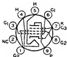
Miniature type used as power amplifier in compact high-fidelity audio equipment. Tube features linear operation over a wide range of power, high power sensitivity, high stability, and
