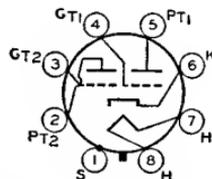
line 3, OUTLINES SECTION. Tube requires octal socket and may be mounted in any position.
