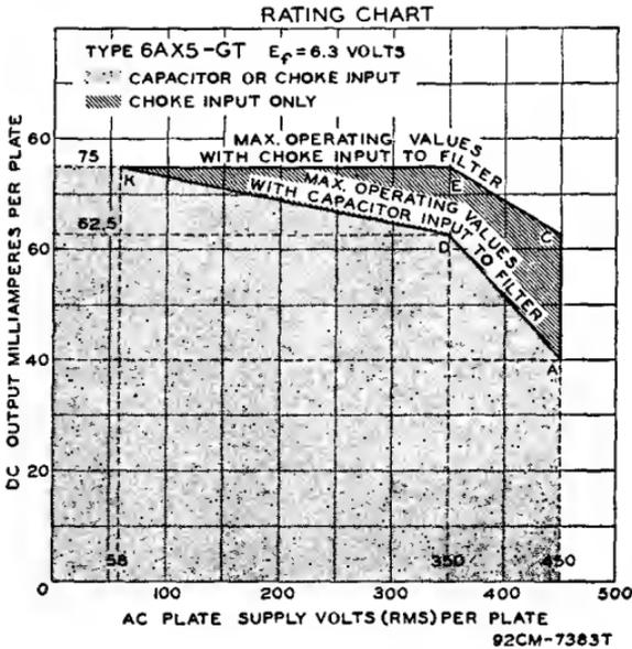
\* Higher values of capacitance than indicated may be used but the effective plate-supply impedance may have to be increased to prevent exceeding the maximum rating for hot-switching transient plate current.
