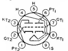
Miniature type used in direct-coupled cathode-drive rf amplifier circuits of vhf television tuners employing series-connected heater strings. Outline 12, OUTLINES SECTION.
