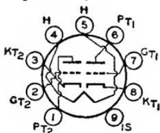
Miniature type used in direct-coupled cathode-drive rf amplifier circuits of vhf television tuners. In such circuits, one triode unit is used as the direct-coupled grounded-cathode driv-
