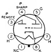
Glass octal type used as a control tube for twin-indicator type electron-ray tubes. Outline 36, OUTLINES SECTION. Contains two triodes with different cutoff characteristics. If a dc voltage is applied to the common control grid in suitable circuit, one triode section operates on weak signals while the other operates on strong signals. Heater voltage (ac/dc), 6.3; amperes, 0.15. This is a DISCONTINUED type listed for reference only.
