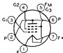
and may be mounted in any position. Types 3S4 and 1S4 are identical except for filament arrangement. Type 3S4 features a filament mid-tap so that tube may be used either with a 1.4-volt battery supply or in series with other miniature tubes having 0.050-ampere filaments.
