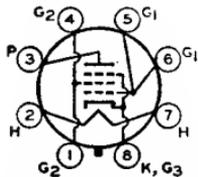
Glass octal types used in push-pull power amplifier circuits of high-fidelity audio equipment. Tubes provide high powersensitivity and high stability and are capable of delivering high power
