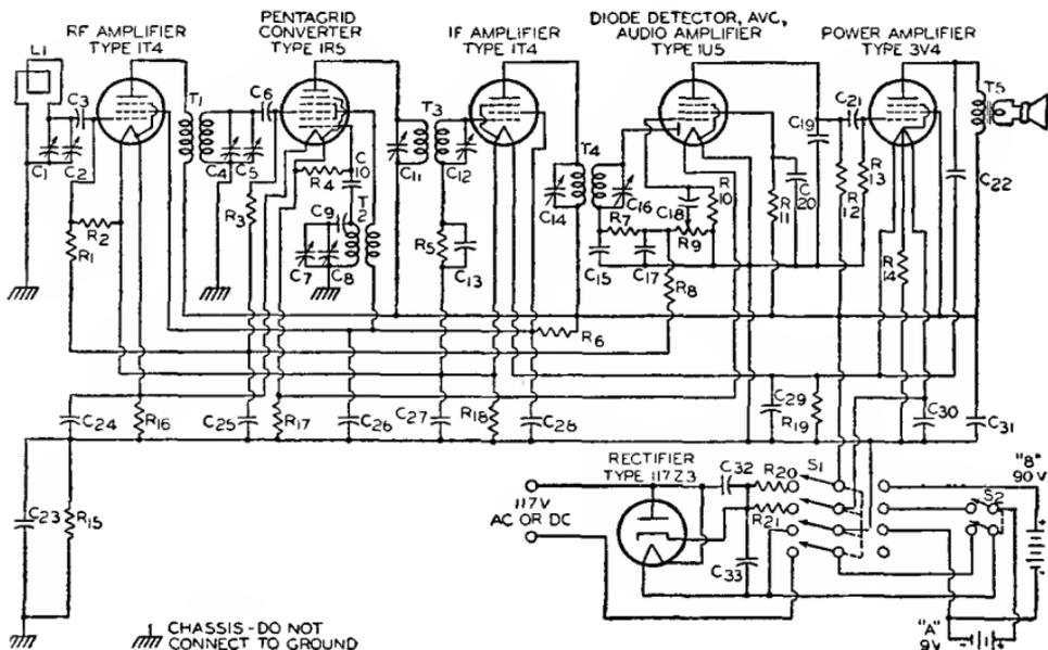
C<sub>1</sub> C<sub>4</sub> C<sub>5</sub> = Ganged tuning capacitors, 20-450  $\mu\mu\text{f}$
