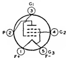
Glass type used in output stage of battery-operated receivers. Outline 42, OUTLINES SECTION. Tube requires five-contact socket. Filament volts (dc), 2.0; amperes, 0.26. Typical operation as class A<sub>1</sub> amplifier: plate and grid-No.2 volts, 180 max; grid-No.1 volts, -18; plate ma., 22; grid-No.2 ma., 5; plate resistance, 55000 ohms; transconductance, 1750  $\mu$ mhos;
