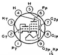
used in oscillator or sync circuits. Outline 12, OUTLINES SECTION. Heater volts (ac/dc), 4.7; amperes, 0.6; warm-up time (average), 11 seconds. Except for heater rating, this type is identical with miniature type 6AN8.
