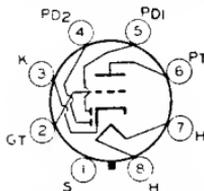
Metal type used as combined detector, amplifier, and avc tube. Within maximum ratings this type is electrically identical to type 6BF6 except for interelectrode capacitances and heater current. Outline 3, OUTLINES SECTION. Tube requires octal socket and may be mounted in any position. Heater volts (ac/dc), 6.3; amperes, 0.15. Maximum ratings of triode
