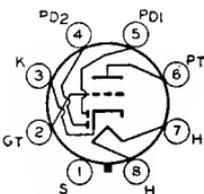
Metal type used as combined detector, amplifier, and avc tube. It is equivalent in performance to miniature type 6BF6. Outline 3, OUTLINES SECTION. Tube requires octal socket and may be mounted in any position. Heater volts (ac/dc), 6.3; amperes, 0.3. Maximum ratings and typical operation of triode unit as class A<sub>1</sub> amplifier: plate volts, 250 *max*;
