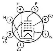
warm-up time (average), 11 seconds. Peak heater-cathode volts: heater negative with respect to cathode, 200 *max*; heater positive with respect to cathode, 200 *max* (the dc component must not exceed 100 volts). Except for heater and heater-cathode ratings, this type is identical with miniature type 6AU6.
