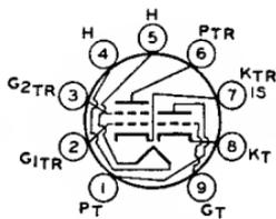
mixer or amplifier and the triode unit is used in oscillator and rf amplifier circuits. Outline 12, OUTLINES SECTION. Heater volts (ac/dc), 4.7; amperes, 0.6; warm-up time (average), 11 seconds. Except for heater rating, this type is identical with miniature type 6CQ8.
