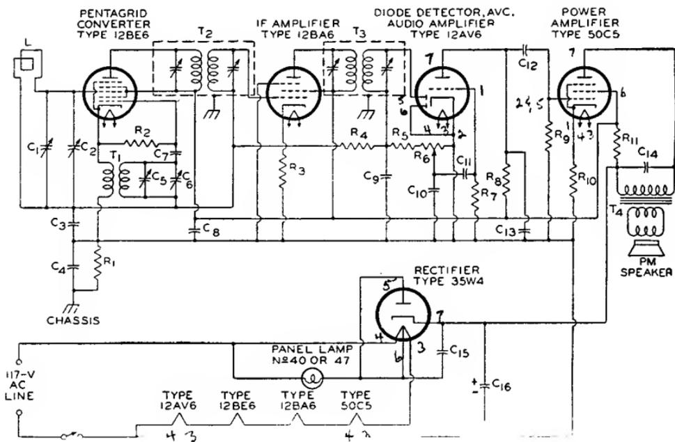
C<sub>1</sub> C<sub>3</sub>=Ganged tuning capacitors; C<sub>1</sub>, 10-365  $\mu$ f; C<sub>3</sub>, 7-115  $\mu$ f
