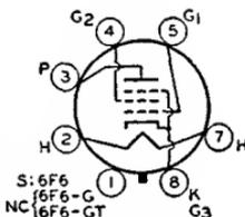
Outlines 6, 42 and 26, respectively, **OUTLINES SECTION**. Type 6F6-GT may be supplied with pin No.1 omitted. Tubes require octal socket and may be mounted in any position. It is especially important that these tubes, like other power-handling tubes, be adequately ventilated. Types 6F6-G and 6F6-GT are used principally for renewal purposes.
