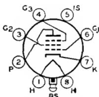
watts; grid-No.2 input, for grid-No.2 voltages up to 150 volts, 0.7 *max* watt (for grid-No.2 voltages from 150 to 300 volts, see curve page 66); cathode-bias resistor, 250 ohms; grid No.3 and internal shield connected to cathode at socket; plate resistance (approx.), 1 megohm; transconductance, 3300  $\mu$ mhos; plate ma., 6.8; grid-No.2 ma., 1.9; peak heater-cathode volts, 90 *max*. Type 7AH7 is used principally for renewal purposes.
