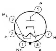
Glass octal type used in power supply of ac/dc receivers. The heater is provided with a tap for operation of a panel lamp. Outline 22, OUTLINES SECTION. Tube requires
