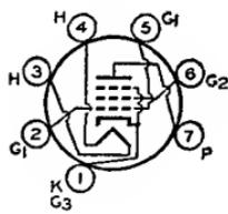
Miniature type used as a vertical deflection amplifier in television receivers employing series-connected heater strings. Outline 13, OUTLINES SECTION. Tube requires miniature seven-contact socket and may be mounted in any position.
