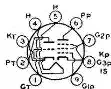
Heater volts (ac/dc), 4.7; amperes, 0.6; warm-up time (average), 11 seconds. Except for heater rating, this type is identical with miniature type 6BR8-A.
