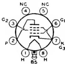
Glass lock-in type used in output stage of radio receivers. Outline 20, OUTLINES SECTION. Tube requires lock-in socket. Heater volts (ac/dc), 6.3; amperes, 0.4. Except for interelectrode capacitances, this type is the same electrically as glass-octal type 6K6-GT. Type 7B5 is used principally for renewal purposes.
