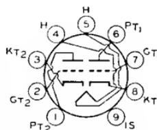
Heater volts (ac/dc), 4.2; amperes, 0.6; warm-up time (average), 11 seconds. Except for heater rating, this type is identical with miniature type 6BQ7-A.
