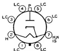
Glass octal type used as rectifier of high-voltage pulses produced in the scanning systems of television receivers. Outline 47, OUTLINES SECTION. Tube requires octal socket and may be mounted in any position. Low-potential circuits should not be connected to any of the socket terminals. Any or all of the following socket-terminal connections are permissible and may aid in corona reduction: socket terminals 1, 3,
