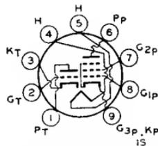
or as a reactance tube. The triode unit is used in low-frequency oscillator, sync-separator, sync-clipper, and phase-splitter circuits. Outline 12, OUTLINES SECTION. Tube requires miniature nine-contact socket and may be mounted in any position.
