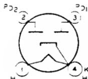
Glass type used in power supply of radio equipment having high dc requirements. Outline 43, OUTLINES SECTION. Tube requires four-contact socket. Heater volts (ac), 5.0; amperes, 2. This type is identical electrically with glass octal type 5V4-G. Type 83-v is a DISCONTINUED type listed for reference only.
