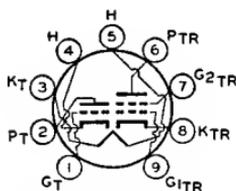
Miniature type used as combined oscillator and mixer in vhf tuners of television receivers employing series-connected heater strings. Outline 12, OUTLINES SECTION. Tube requires
