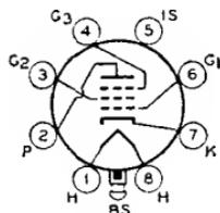
Glass lock-in type used as rf or if amplifier in ac/dc radio receivers. Outline 15, OUTLINES SECTION. Tube requires lock-in socket. Heater volts (ac/dc), 12.6; amperes, 0.15. Except for heater rating, this type is electrically identical with type 7H7. Type 14H7 is a DISCONTINUED type listed for reference only.
