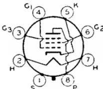
Metal type used in rf or if stages of radio receivers particularly those employing avc. Outline 3, OUTLINES SECTION. Tube requires octal socket and may be mounted in any position. Heater volts (ac/dc), 6.3; amperes, 0.15. Typical operation as class A<sub>1</sub> amplifier: plate volts, 250 (300 *max*); grid-No.2 supply volts, 300 *max*; grid-No.2 volts, 100; grid-No.1 volts, -3; grid No.3 connected to cathode at socket;
