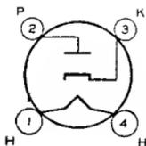
Glass type used in ac/dc or automobile receivers. Outline 34 or 35, OUTLINES SECTION. Tube requires four-contact socket. Heater volts (ac/dc), 6.3; amperes, 0.3. Maximum ratings as half-wave rectifier: peak inverse plate volts, 1000; peak plate ma., 270; peak heater-cathode volts, 500; dc output ma., 45. This type is used principally for renewal purposes.
