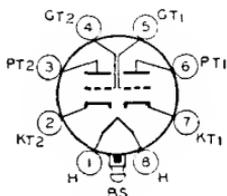
Glass lock-in type used as phase inverter or resistance-coupled amplifier in ac/dc radio receivers. Outline 15, OUTLINES SECTION. Tube requires lock-in socket. Heater volts (ac/dc), 12.6; amperes, 0.15. Except for heater rating, this type is electrically identical with lock-in type 7F7 and glass-octal type 6SL7-GT. Type 14F7 is used principally for renewal purposes.
