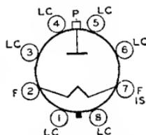
vision scanning systems. Outline 28, OUTLINES SECTION. This type may be supplied with pins 1, 4, and/or 6 omitted. Tube requires octal socket and may be mounted in any position. Except for physical dimensions, this type is identical with glass octal type 1B3-GT.
