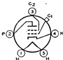
Heater volts (ac/dc), 2.5; amperes, 1.75. Typical operation and maximum ratings as class A<sub>1</sub> amplifier: plate volts, 250 (275 *max*); grid-No.2 volts, 90; grid-No.1 volts, -3; plate resistance, 0.6 megohm; transconductance, 1050  $\mu$ mhos; plate ma., 4; grid-No.2 ma., 1.7 *max*. This type is used principally for renewal purposes.
