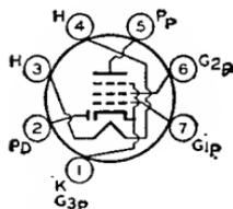
Miniature type used as combined detector and audio amplifier in automobile and ac-operated radio receivers. The diode unit is used as an AM detector, and the pentode unit as an automatic-volume-controlled audio amplifier. Outline 11, OUTLINES SECTION. Tube requires miniature seven-contact socket and may be mounted in any position.
