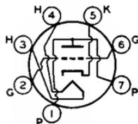
LINES SECTION. Tube requires miniature seven-contact socket and may be mounted in any position.
