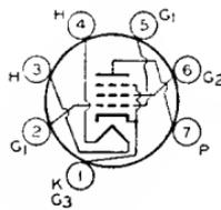
0.6; warm-up time (average), 11 seconds. Except for heater rating, this type is identical with miniature type 6CU5.
