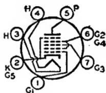
Miniature type used as rf amplifier in automobile radio receivers operating from a 12-volt storage battery. Outline 11, **OUTLINES SECTION**. Grid No.1 and grid No.3 are independent control electrodes. Tube requires miniature seven-contact socket and may be mounted in any position. This type is used principally for renewal purposes.
