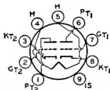
Miniature type used in direct-coupled cathode-drive rf amplifier circuits of vhf television tuners employing series-connected heater strings. Outline 12, OUTLINES SECTION.
