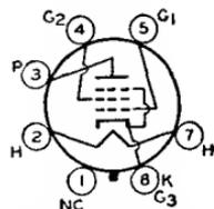
22, OUTLINES SECTION. This type may be supplied with pin No.1 omitted. Heater volts (ac/dc), 12.6; amperes, 0.6; warm-up time (average), 11 seconds. Peak heater-cathode volts: heater negative with respect to cathode, 300 max (the dc component must not exceed 200 volts); heater positive with respect to cathode, 200 max (the dc component must not exceed 100 volts). Except for heater and heater-cathode ratings, this type is identical with glass octal type 6W6-GT.
