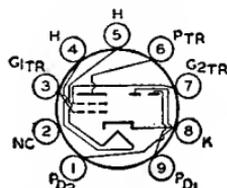
tection and automatic volume control, and the tetrode unit is used as the driver for the output stage. Outline 14, OUTLINES SECTION. Tubes require miniature nine-contact socket and may be mounted in any position. For characteristics and typical operation with grid-No.2-resistor bias of tetrode unit of the 12DS7 as class A<sub>1</sub> amplifier, refer to type 12DL8. Type 12DS7-A is a DISCONTINUED type listed for reference only.
