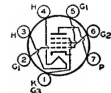
Miniature type used in the audio output stage of radio and television receivers and in phonographs. This type has unusually high power sensitivity and is capable of providing relatively high power output at low plate and screen-grid voltages with a low af grid-No.1 driving voltage. Outline 13, OUTLINES SECTION. Tube requires miniature seven-contact socket and may be mounted in any position.
