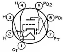
seven-contact socket and may be mounted in any position. For typical operation as resistance-coupled amplifier, refer to Chart 3, RESISTANCE-COUPLED AMPLIFIER SECTION.
