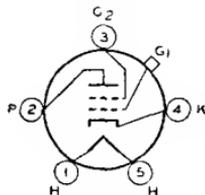
Glass type used as rf or if amplifier in ac receivers. Maximum over-all length, 5-1/32 inches; maximum diameter, 1-13/16 inches. Tube requires five-contact socket. Heater volts (ac/dc), 2.5; amperes, 1.75. Characteristics as class A<sub>1</sub> amplifier: plate volts, 250 (275 max); grid-No.2 volts, 90 max; grid-No.1 volts, -3
