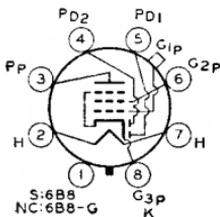
Metal type 6B8 and glass octal type 6B8-G are used as combined detector, amplifier, and avc tubes. Outlines 4 and 39, respectively, OUTLINES SECTION. Type 6B8 is used principally for renewal purposes; 6B8-G is a DISCONTINUED type listed for reference only. Tubes require octal socket. Heater volts (ac/dc), 6.3; amperes, 0.3. Maximum ratings of pentode unit as class A<sub>1</sub> amplifier: plate volts,
