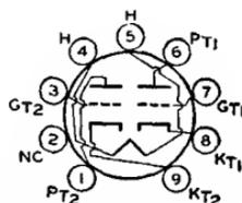
deflection circuits, and unit No.2 as a vertical deflection amplifier. This type has a controlled heater warm-up time for use in receivers employing series-connected heater strings. Outline 14, OUTLINES SECTION. Tube requires miniature nine-contact socket and may be mounted in any position.
