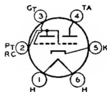
Glass type with triode unit used to indicate visually by means of a fluorescent target the effects of a change in a controlling voltage. It is used as a convenient means of indicating accurate radio-receiver tuning. Outline 34, OUTLINES SECTION. Tube requires six-contact socket. Heater volts (ac/dc), 6.3; amperes, 0.15. Maximum ratings in indicator service: triode-plate supply volts, 180 *max*; fluorescent-target volts, 180 *max*, 125 *min*. This type is used principally for renewal purposes.
