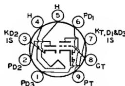
are used for FM detection. Type 6T8-A has a controlled heater warm-up time for use in receivers employing series-connected heater strings. Outline 12, OUTLINES SECTION. Tubes require miniature nine-contact socket and may be mounted in any position. For typical operation as resistance-coupled amplifier, refer to Chart 3, RESISTANCE-COUPLED AMPLIFIER SECTION. Type 6T8 is a DISCONTINUED type listed for reference only.
