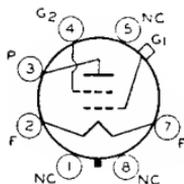
Glass octal type used in battery-operated receivers as rf or if amplifier. Outline 39, OUTLINES SECTION. Filament volts (dc), 2.0; amperes, 0.06. This is a DISCONTINUED type listed for reference only. It is similar electrically to type 1D5-GP.
