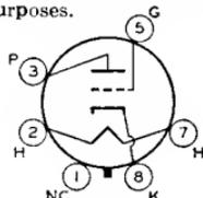
Glass octal type used as class A<sub>1</sub> amplifier in ac/dc radio receivers. Outline 22, OUTLINES SECTION. Heater volts (ac/dc), 6.3; amperes, 0.3. Maximum ratings as class A<sub>1</sub> amplifier: plate volts, 300 *max*; plate dissipation, 2.5 *max* watts. This is a DISCONTINUED type listed for reference only.
