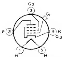
Glass type used as rf or if amplifier in radio receivers, particularly those employing avc. Outline 40, OUTLINES SECTION. Tube requires five-contact socket. Heater volts (ac/dc), 6.3; amperes, 0.3. Characteristics as class A<sub>1</sub> amplifier: plate volts, 250 max; grid-No.2 volts, 90 max; grid-No.1 volts, -3 min; plate ma., 5.8; grid-No.2 ma., 1.4; plate resistance, 1.0 meg-
