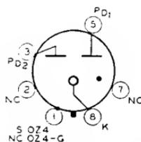
Maximum ratings for full-wave rectifier service: peak starting supply volts (per plate), 300 *min*; peak plate-to-plate volts, 1000 *max*; peak plate ma. (per plate), 200 *max*; dc output ma., 75 *max*; 30 *min*; dc output volts, 300 *max*; average dynamic tube voltage drop, 24 volts. These types are used principally for renewal purposes.
