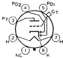
Glass octal type used as combined detector, amplifier, and avc tube. Outline 39, OUTLINES SECTION. Except for interelectrode capacitances, this type is identical electrically with type 85. Heater volts (ac/dc), 6.3; amperes, 0.3. For diode operation curves, refer to type 6AV6. Type 6V7-G is a DISCONTINUED type listed for reference only.
