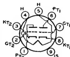
Heater volts (ac/dc), 4.7; amperes, 0.6; warm-up time (average), 11 seconds. Except for heater rating, this type is identical with miniature type 6BK7-B.
