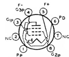
grid-No.1 volts, 0; plate resistance (approx.), 0.4 megohm; transconductance, 600  $\mu$ mhos; plate ma., 1.0; grid-No.2 ma., 0.4; total cathode ma., 2.0 max. Maximum diode plate ma., 0.25. This is a DISCONTINUED type listed for reference only.
