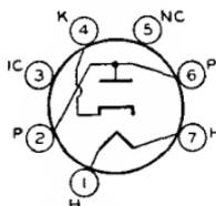
*ma.*, 390 *ma*; dc output *ma.*, 65 *ma*; peak heater-cathode volts, 175 *ma*. Typical operation with capacitor-input filter: ac plate volts (rms), 117; minimum total effective plate-supply impedance, 15 ohms; dc output *ma.*, 65. This is a DISCONTINUED type listed for reference only.
