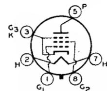
**OUTLINES SECTION.** Heater volts (ac/dc), 25; amperes, 0.3. Except for heater rating, this type is identical with glass octal type 6AV5-GA.
