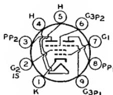
Heater volts (ac/dc), 3.15; amperes, 0.6; warm-up time (average), 11 seconds. Except for heater rating, this type is identical with miniature type 6BU8.
