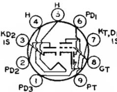
Miniature type used as combined audio amplifier, AM detector, and FM detector in AM/FM receivers of the a/c or "transformer" type. Outline 12, OUTLINES SECTION. Tube requires miniature nine-contact socket and may be mounted in any position. Heater volts (ac/dc), 18.9; amperes, 0.15. Except for heater rating, this type is identical with miniature type 6T8-A. Type 19T8 is used principally for renewal purposes.
