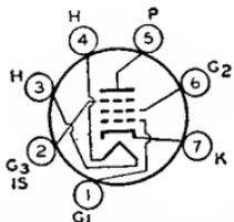
Miniature type used as rf amplifier in automobile radio receivers operating from a 12-volt storage battery. Outline 11, OUTLINES SECTION. Tube requires miniature seven-contact socket and may be mounted in any position.
