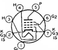
Miniature type used as rf or if amplifier in television receivers employing series-connected heater strings. Outline 11, OUTLINES SECTION. Heater volts (ac/dc), 3.15; amperes,
