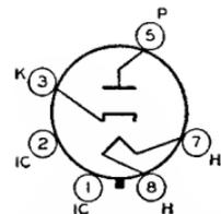
Glass octal type used as damper tube in television receivers. Outline 22, OUTLINES SECTION. This type may be supplied with pin No.1 omitted. Tube requires octal socket and may
