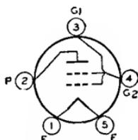
plification factor, 5.6; transconductance, 2350  $\mu$ mhos; load resistance for maximum undistorted power output, 6400 ohms; output watts, 1.25. This is a DISCONTINUED type listed for reference only.
