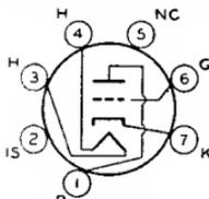
Miniature type used as cathode-drive amplifier, frequency converter, or oscillator at frequencies up to about 300 megacycles per second particularly in television and FM receivers. Outline
