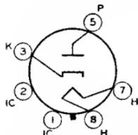
Heater volts (ac/dc), 25; amperes, 0.3. Except for heater rating, this type is identical with glass octal type 6AX4-GT.
