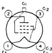
Glass type used as rf or if amplifier in battery-operated radio receivers, particularly those employing avc. Maximum over-all length, 5-1/32 inches; maximum diameter, 1-13/16 inches. Tube requires four-contact socket. Filament volts (dc), 2.0; amperes, 0.06. Characteristics as class A<sub>1</sub> amplifier: plate volts, 180 max; grid-No.2 volts, 67.5 max; grid-No.1 volts, -3
