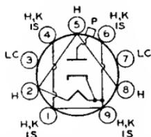
Miniature type used as rectifier of high-voltage pulses produced in scanning systems of color-television receivers. Outline 16, OUTLINES SECTION. Tube requires miniature 9-contact socket and may be mounted in any position. Socket terminals 3 and 7 may be connected to the heater. Heater volts (ac), 3.15; amperes, 0.22. Maximum ratings as pulsed rectifier in 525-line, 30-frame system: peak in verse plate volts.
