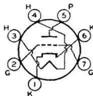
lead resistance with consequent reduction in input conductance. In addition, the basing arrangement facilitates isolation of input and output circuits and permits short, direct connections to base-pin terminals. Outline 11, OUTLINES SECTION. Tubes require miniature seven-contact socket and may be mounted in any position.
