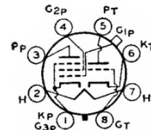
Heater volts (ac/dc), 25; amperes, 0.15. Typical operation of pentode unit as class A<sub>1</sub> amplifier: plate and grid-No.2 volts, 100; grid-No.1 volts, -3; plate ma., 7.6; grid-No.2 ma., 2; plate resistance, 185000 ohms; transconductance, 2000 μmhos. Triode unit: plate volts, 100; grid volts, -1; plate ma., 0.6; amplification factor, 112; plate resistance, 75000; transconductance, 1500 μmhos. This is a DISCONTINUED type listed for reference only.
