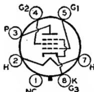
Tube requires octal socket and may be mounted in any position. For typical operation as push-pull class A<sub>1</sub>, class AB<sub>1</sub> (within maximum ratings), and class AB<sub>2</sub> amplifier, and for curves of average plate characteristics, refer to type 6L6-GC.
