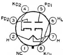
Glass octal type used as half-wave rectifier or voltage doubler in ac/dc receivers. Outline 36, OUTLINES SECTION. The heater is provided with a tap for operation of a panel lamp. Without panel lamp, heater volts (ac/dc) of entire heater (pins 2 and 7), 50; amperes, 0.15. With panel lamp, heater volts (ac/dc) of panel-lamp section (pins 6 and 7 with 0.15 ampere
