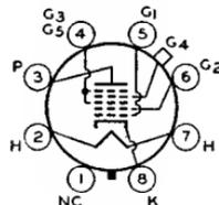
Glass octal type used in superheterodyne circuits. Outline 39, OUTLINES SECTION. Tube requires octal socket. Heater volts (ac/dc), 6.3; amperes, 0.15. Except for interelectrode capacitances and heater rating, the 6D8-G is similar electrically to type 6A8-G. Type 6D8-G is a DISCONTINUED type listed for reference only.
