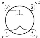
Glass type used in power supply of radio receivers. Maximum over-all length, 6-1/4 inches; maximum diameter, 2-7/16 inches. Tube requires four-contact socket. Filament volts (ac), 7.5; amperes, 1.25. Ratings as half-wave rectifier: peak inverse plate volts, 2000 *max*; peak plate ma., 500 *max*; dc output ma., 85 *max*. This is a DISCONTINUED type listed for reference only.
