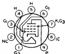
Heater volts (ac/dc), 4.7; amperes, 0.6; warm-up time (average), 11 seconds. Except for heater rating, this type is identical with miniature type 6CZ5.
