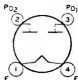
Glass type used in power supply of radio equipment having moderate direct-current requirements. Outline 43 and 34, OUTLINES SECTION, except maximum over-all length 4 inches; maximum seated length, 3-3/8 inches. Tube requires four-contact socket and should be mounted preferably in a vertical position. Horizontal mounting is permissible if pins 1 and 4 are in a horizontal plane. Filament volts (ac),
