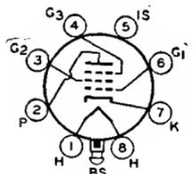
Glass lock-in type used as rf or if amplifier in radio receivers employing avc. Outline 15, OUTLINES SECTION. Tube requires lock-in socket. Heater volts (ac/dc), 6.3; amperes, 0.15. Characteristics and maximum ratings as class A<sub>1</sub> amplifier: plate volts, 250 (300 *max*); grid-No.2 volts, 100 *max*; grid-No.1 volts, -3 (positive-bias value, 0 *max*); grid No.3 and internal
