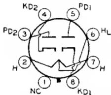
Glass octal type used as half-wave rectifier or voltage doubler in ac/dc receivers. This type is used particularly in "transformerless" receivers of either the ac/dc type or the voltage-doubler type. The heater is provided with a tap for operation of a panel lamp. Outline 22, OUTLINES SECTION. Tube requires octal socket.
