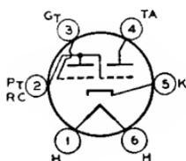
Glass type with triode unit used to indicate visually by means of a fluorescent target the effects of a change in a controlling voltage. It is used as a convenient means of indicating accurate radio receiver tuning. Outline 34 or 35, OUTLINES SECTION. Tube requires six-contact socket. Except for its heater rating (2.5 volts ac/dc; 0.8 ampere), the 2E5 has electrical characteristics identical with type 6E5. Type 2E5 is a DISCONTINUED type listed for reference only.
