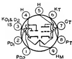
Miniature type used as combined horizontal phase detector and reactance tube in television receivers employing series-connected heater strings. The triode unit is used in sync-separator, sync-amplifier, or audio-amplifier circuits. Outline 12, OUTLINES SECTION. Heater volts (ac/dc), 8.4 (series), 4.2 (parallel); amperes, 0.225 (series), 0.45 (parallel); warm-up time (average), 11 seconds (parallel). Except for heater rating, this type is identical with type 6CN7.
