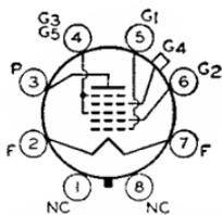
grid-No.1 (oscillator-grid) resistor, 50000 ohms; plate ma., 1.5; grids-No.3-and-No.5 ma., 4; grid-No.1 ma., 0.2. This is a DISCONTINUED type listed for reference only.
