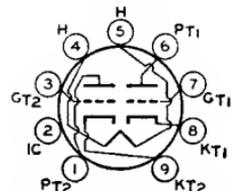
Miniature type used in television receivers employing series-connected heater-strings. Low-mu triode unit is used as vertical-deflection amplifier; high-mu triode unit is used as vertical-deflection oscillator. Outline 14, OUTLINES SECTION. Heater volts (ac/dc), 11; amperes, 0.45; warm-up time (average), 11 seconds. Except for heater rating, this type is identical with miniature type 6CY7.
