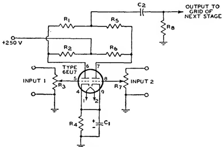
$C_1=10 \mu\text{f}$ , electrolytic, 25 v.
