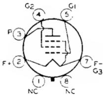
Glass octal type used in output stage of battery-operated receivers. Outline 42, OUTLINES SECTION. Tube requires octal socket. Filament volts (dc), 2.0; amperes, 0.12. Typical operation as class A<sub>1</sub> amplifier: plate and grid-No.2 (screen-grid) volts, 135 *max*; grid-No.1 volts, -16.5; plate ma., 7.0; grid-No.2 ma., 2.0; plate resistance, 105000 ohms; load resistance, 13500 ohms; output watts, 0.45. This is a DISCONTINUED type listed for reference only.
