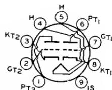
Heater volts (ac/dc), 5.6; amperes, 0.45; warm-up time (average), 11 seconds. Except for heater rating, this type is identical with miniature type 6BQ7-A.
