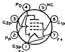
Miniature type used in battery-operated portable radio receivers as combined AM detector and af voltage amplifier. Outline 11, **OUTLINES SECTION**. Tube requires miniature seven-contact socket and may be mounted in any position. For typical operation as a resistance-coupled amplifier, refer to Chart 1, **RESISTANCE-COUPLED AMPLIFIER SECTION**.
