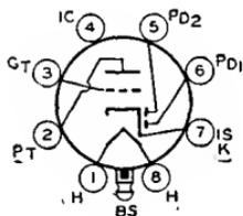
Glass lock-in type used as combined detector, amplifier, and avc tube. Outline 15, OUTLINES SECTION. Tube requires lock-in socket. Heater volts (ac/dc), 6.3; amperes, 0.3. Except for interelectrode capacitances, this type is the same electrically as metal type 6SQ7. Type 7B6 is used principally for renewal purposes.
