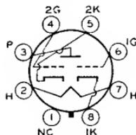
Glass octal type used as a voltage amplifier or as a driver for two type 6AC5-GT tubes in dynamic-coupled, push-pull amplifiers. In the latter service, type 6AE7-GT replaces two tubes ordinarily required as drivers. Outline 22, OUTLINES SECTION. Heater volts (ac/dc), 6.3; amperes, 0.5. This is a DISCONTINUED type listed for reference only.
