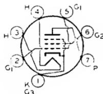
for terminal connections and slightly higher ratings, type 35C5 is equivalent in performance to miniature type 35B5 and, within its maximum ratings, to glass octal type 35L6-GT. The basing arrangement of the 35C5 simplifies the problem of meeting Underwriters' Laboratories requirements in the design of ac/dc receivers.
