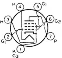
Miniature type used in output stage of compact, ac/dc radio receivers. Because of its high power sensitivity and high efficiency at plate and screen-grid voltages available in ac/dc receivers, the 50C5 is capable of providing a relatively high power output.
