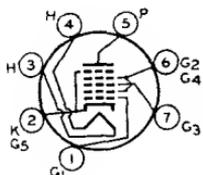
Miniature type used for converter applications in ac/dc radio receivers. Outline 11, OUTLINES SECTION. Tube requires miniature seven-contact socket and may be mounted in any position. Heater volts (ac/dc), 18; amperes, 0.1.
