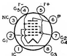
Subminiature type used in small, compact, battery-operated receivers for the standard AM broadcast band. Outline 8, OUTLINES SECTION. Tube requires subminiature eight-contact socket. Filament volts (dc), 1.25; amperes, 0.04. Typical operation as converter: plate volts and grids-No.2-and-No.4 supply volts, 67.5 *max*; grids-No.2-and-No.4 resistor, 20000 ohms; grid-No.3 volts, 0; grid-No.1 resistor, 0.1 megohm;
