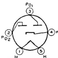
input filter: ac plate-to-plate supply volts (rms), 650; minimum total effective plate-supply impedance per plate, 150 ohms; dc output ma., 60. Typical operation with choke-input filter: ac plate-to-plate supply volts (rms), 900; minimum filter-input choke, 10 henries; dc output ma., 60. This type is used principally for renewal purposes.
