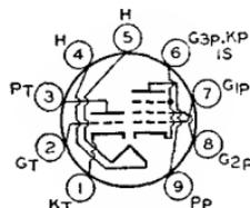
heater strings. The pentode unit is used as an if amplifier, video amplifier, agc amplifier, or reactance tube. The triode unit is used in low-frequency oscillator, sync-separator, sync-clipper, and phase-splitter circuits. Outline 14, **OUTLINES SECTION**. Tubes require miniature nine-contact socket and may be mounted in any position. Type 6AW8 is a discontinued type listed for reference only.
