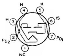
Miniature type used as a horizontal phase detector in television receivers. Outline 11, OUTLINES SECTION. Tube requires miniature seven-contact socket and may be mounted in
