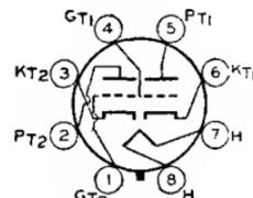
5, and 6) be used as the oscillator. Outline 22, **OUTLINES SECTION**. Tube requires octal socket and may be mounted in any position.
