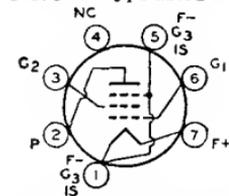
requires miniature seven-contact socket and may be mounted in any position. Because the grid No.2 can be operated at the same voltage as the plate, a voltage-dropping resistor is not needed. For typical operation as a resistance-coupled amplifier, refer to Chart 2, RESISTANCE-COUPLED AMPLIFIER SECTION.
