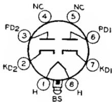
Lock-in type used as half-wave rectifier or voltage doubler in ac/dc receivers. Outline 20, OUTLINES SECTION. Tube requires lock-in socket. Heater volts (ac/dc), 50; amperes, 0.15. This type is electrically identical with glass octal type 50Y6-GT and, except for heater rating, with glass octal type 25Z6-GT. Refer to type 25Z6-GT for maximum ratings, typical operation, and curves. Type 50X6 is used principally for renewal purposes.
