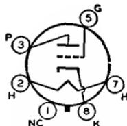
volts (ac/dc), 6.3; amperes, 0.4. Maximum ratings as push-pull class B power amplifier: plate volts, 250 *max*; peak plate ma., 110 *max*; average plate dissipation, 10 *max* watts. This type is used principally for renewal purposes.
