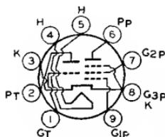
Miniature types used as combined oscillator and mixer tubes in television receivers utilizing an intermediate frequency in the order of 40 megacycles per second. When used in an AM/FM
