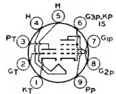
Triode unit is used in sync-amplifier, sync-separator, sync-clipper, and phase-inverter circuits. Outline 14, OUTLINES SECTION. Tube requires nine-contact socket and may be mounted in any position.
