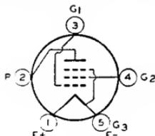
Glass type used in output stage of battery-operated receivers. Outline 43, OUTLINES SECTION. Tube requires five-contact socket. Filament volts (dc), 2.0; amperes, 0.12. Type 1F4 is similar electrically to type 1F5-G. Type 1F4 is a DISCONTINUED type listed for reference only.
