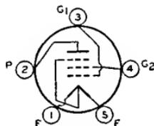
250 *ma*; cathode-bias resistor, 450 ohms; plate *ma.*, 31; grid-No.2 *ma.*, 6; plate resistance, 60000 ohms; transconductance, 2500  $\mu$ mhos; load resistance, 7000 ohms; power output, 2.7 watts. This type is used principally for renewal purposes.
