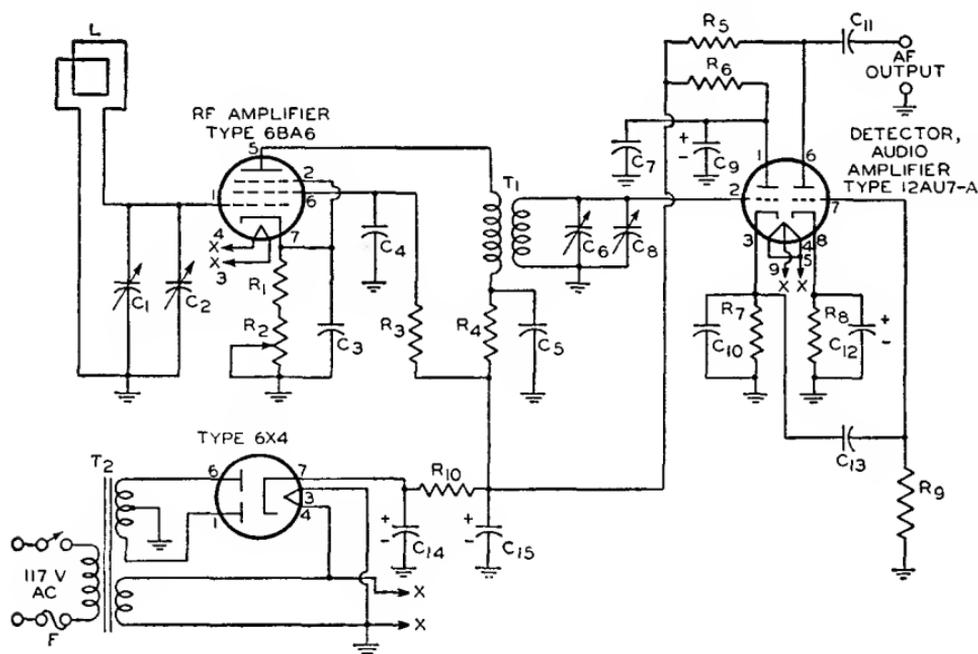
$C_1$   $C_6$ =Ganged tuning capacitors, 10-365  $\mu\text{f}$
