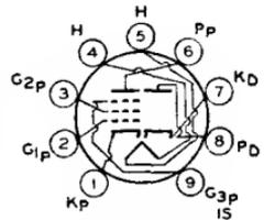
The pentode unit is used as an if amplifier, video amplifier, or age amplifier. The high-perveance diode is used as an audio detector, video detector, or dc restorer. Outline 12, OUTLINES SECTION. Tubes require miniature nine-contact socket and may be mounted in any position. Type 6AM8 is a DISCONTINUED type listed for reference only.
