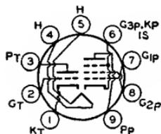
ploying series-connected heater strings. The pentode unit is used as a video amplifier, an agc amplifier, or a reactance tube. The triode unit is used in low-frequency oscillator and phase-splitter circuits. Outline 14, OUTLINES SECTION. Tube requires miniature nine-contact socket and may be mounted in any position.
