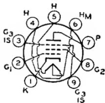
Miniature type used as video-output-amplifier tube in television receivers employing series-connected heater strings. Outline 14, **OUTLINES SECTION**. Tube requires miniature nine-contact socket and may be operated in any position.
