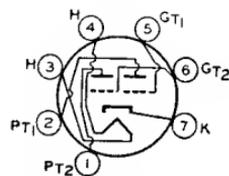
(ac, dc), 4.7; amperes, 0.6; warm-up time (average), 11 seconds. Except for heater rating, this type is identical with miniature type 6J6.
