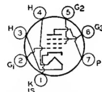
OUTLINES SECTION. Heater volts (ac/dc), 4.2; amperes, 0.45; warm-up time (average), 11 seconds. Peak heater-cathode volts, 200 *max*. When the heater is positive with respect to the cathode, the dc component of the heater-cathode voltage must not exceed 100 volts. Except for heater and heater-cathode ratings, this type is identical with miniature type 6BN6.
