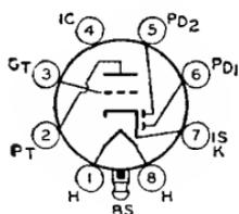
Glass lock-in type used as combined detector, amplifier, and avc tube in ac/dc radio receivers. Outline 15, OUTLINES SECTION. Tube requires lock-in socket. Heater volts, (ac/dc), 12.6; amperes, 0.15. Except for heater rating, this type is electrically identical with lock-in type 7E6 and miniature type 6BF6. Type 14E6 is a DISCONTINUED type listed for reference only.
