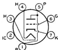
Miniature type used in compact radio equipment as a local oscillator in FM and other high-frequency circuits. It may also be used as a class C rf amplifier. In such service, it delivers
