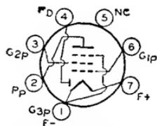
proved structure which greatly reduces any tendency toward microphonic effects. In addition, the diode unit is effectively shielded from the pentode unit to prevent "play-through." Outline 11, OUTLINES SECTION. Tube requires miniature seven-contact socket and may be mounted in any position. For typical operation as a resistance-coupled amplifier, refer to Chart 1, RESISTANCE-COUPLED AMPLIFIER SECTION.
