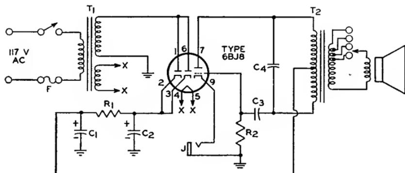
$C_1$   $C_2$  = 20  $\mu$ f, electrolytic, 150 v.
