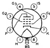
max watt; grid No.1 volts, -3; grid No.3 connected to cathode at socket; plate resistance, greater than 1 megohm; transconductance, 1575 μmhos; plate ma., 2.2; grid-No.2 ma., 0.7. Within the limits of its maximum ratings, this type is similar in performance to metal types 6SJ7 and 12SJ7. Type 14C7 is used principally for renewal purposes.
