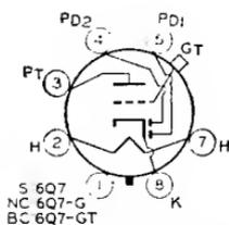
Similar electrically in most respects to types 6SQ7 and 6AT6. Maximum ratings and typical operation of the triode unit as a class A<sub>1</sub> amplifier are the same as those for type 6AT6 except that with a plate voltage of 100 volts, the transconductance is 1200  $\mu$ mhos and the plate resistance 58000 ohms. For triode-unit, grid-bias considerations and diode curves, refer to type 6AV6.
