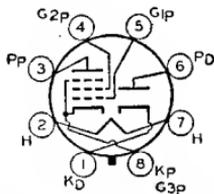
$\mu$ mhos; load resistance, 4500 ohms; output watts, 0.77. Maximum ratings of rectifier unit: peak inverse plate volts, 350; peak plate ma., 450; dc output ma., 75; peak heater-cathode volts, 175. This is a DISCONTINUED type listed for reference only.
