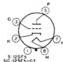
Heater volts (ac/dc), 12.6; amperes, 0.15. Except for heater rating, these types are identical with metal type 6SF5 and glass octal type 6SF5-GT, respectively. Type 12SF5-GT is a **DISCONTINUED** type listed for reference only.
