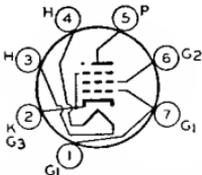
Miniature type used in output stage of compact ac/dc receivers. Because of its high power sensitivity at plate and screen-grid voltages available in ac/dc receivers, it is capable of providing a relatively high power output. Outline 13, OUTLINES SECTION. Tube requires miniature seven-contact socket and may be mounted in any position. Except for basing arrangement, type 50B5 is identical with miniature type 50C5.
