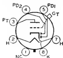
Glass octal type used as combined detector, amplifier, and avc tube. Outline 39, OUTLINES SECTION. Tube requires octal socket. Heater volts (ac/dc), 6.3; amperes, 0.3. Within its triode maximum plate-voltage rating of 250 volts, this type is similar electrically to type 6SQ7 and curves under that type apply to the 6B6-G. This is a DISCONTINUED type listed for reference only.
