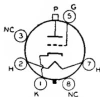
*max*; peak grid volts, -550 *max*; dc plate ma., 1.5 *max*; plate dissipation, 6BD4 20 *max* watts, 6BD4-A 25 *max* watts; peak heater-cathode volts, 180 *max*. These are DISCONTINUED types listed for reference only.
