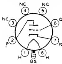
Glass lock-in type used in resistance-coupled amplifier circuits. Outline 15, OUTLINES SECTION. Tube requires lock-in socket. Heater volts (ac/dc), 6.3; amperes, 0.3. Except for interelectrode capacitances, this type has the same maximum ratings and characteristics as metal types 6F5 and 6SF5. Type 7B4 is used principally for renewal purposes.
