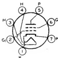
Heater volts (ac/dc), 6.3, amperes, 0.18.
