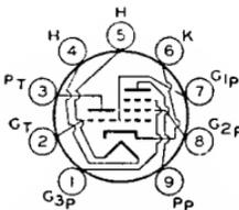
Miniature type used as combined oscillator and mixer tube in "transformerless" AM/FM receivers. Outline 12, OUTLINES SECTION. Tube requires miniature nine-contact socket and may be mounted in any position. Heater volts (ac/dc), 18.9; amperes, 0.15. Except for heater rating, this type is identical with miniature type 6X8.
