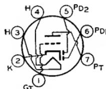
output stages in automobile receivers. It is equivalent in performance to metal type 6SR7. Outline 11, OUTLINES SECTION. Tube requires miniature seven-contact socket and may be mounted in any position.
