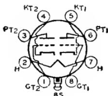
Glass lock-in type used as amplifier or oscillator in ac/dc radio equipment. Outline 15, OUTLINES SECTION, except over-all length is 2-9/32 max inches and seated length is 1-3/4 inches. Tube requires lock-in socket. Heater volts (ac/dc), 12.6; amperes, 0.15. Except for heater rating, this type is electrically identical with lock-in type 7F8. Type 14F8 is used principally for renewal purposes.
