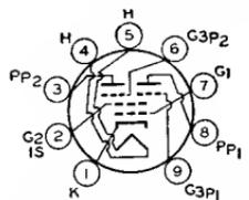
Miniature type used as combined sync separator, sync clipper, and age amplifier tube in television receivers employing series-connected heater strings. Outline 14, OUTLINES SECTION.
