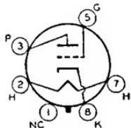
Glass octal type used as detector, amplifier, or oscillator in ac/dc radio equipment. Outline 24, OUTLINES SECTION. This type may be supplied with pin No.1 omitted. Heater volts (ac/dc), 12.6; amperes, 0.15. Except for heater rating and base, this type is identical with glass-octal type 6J5-GT. Type 12J5-GT is used principally for renewal purposes.
