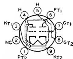
Miniature type used as combined vertical oscillator and vertical deflection amplifier in television receivers employing series-connected heater strings. Outline 14, OUTLINES SECTION. Heater volts (ac/dc), 8.4; amperes, 0.45; warm-up time (average), 11 seconds. Except for heater rating, this type is identical with miniature type 6CM7.
