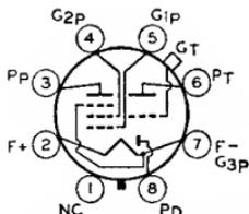
transconductance, 925 μmhos; load resistance, 12000 ohms; total harmonic distortion, 10 per cent; power output, 200 milliwatts. Characteristics of triode unit as class A<sub>1</sub> amplifier: plate volts, 90 (110 max); grid volts, 0; amplification factor, 25; plate resistance (approx.), 43500 ohms; transconductance, 575 μmhos; plate ma., 1.1. This is a DISCONTINUED type listed for reference only.
