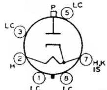
Glass octal type used as rectifier of high-voltage pulses produced in the scanning systems of color television receivers. Outline 32, OUTLINES SECTION. Tube requires octal socket
