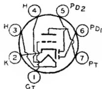
Miniature type used for combined detector, amplifier, and avc tube in compact ac/dc radio receivers. Outline 11, OUTLINES SECTION. Tube requires miniature seven-contact socket and may be mounted in any position. Heater volts (ac/dc), 18; amperes, 0.1.
