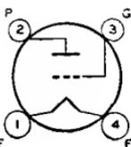
Glass type used in output stage of radio receivers. Outline 43, OUTLINES SECTION. Tube requires four-contact socket. Filament volts (ac/dc), 2.5; amperes, 1.5. Typical operation as class A<sub>1</sub> amplifier: plate supply volts, 275 max; grid volts, -56; cathode-bias resistor, 1550 ohms; amplification factor, 3.5; plate resistance, 1700 ohms; transconductance, 2050
