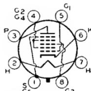
in ELECTRON TUBE APPLICATIONS SECTION. Outline 3, OUTLINES SECTION. Tube requires octal socket and may be mounted in any position. Heater volts (ac/dc), 6.3; amperes, 0.3. For maximum ratings and characteristics in converter service, refer to type 6BA7. Type 6SB7-Y is used principally for renewal purposes.
