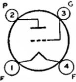
ma., 55; plate resistance, 1800 ohms; amplification factor, 3.8; transconductance, 2100  $\mu$ mhos; load resistance, 4350 ohms; output watts, 4.6. This is a DISCONTINUED type listed for reference only.
