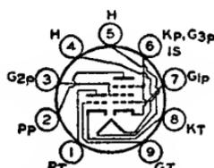
amplifiers in which low hum and reduced noise are required. Outline 12, OUTLINES SECTION. Tube requires miniature nine-contact socket and may be mounted in any position. For operation as resistance-coupled amplifier, refer to Charts 14 and 15, RESISTANCE-COUPLED AMPLIFIER SECTION. In direct-coupled voltage-amplifier phase-splitter circuits, the pentode unit should drive the triode unit.
