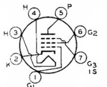
Miniature type used as if and as rf amplifier in television receivers employing series-connected heater strings. Outline 11, OUTLINES SECTION. Heater volts (ac/dc), 4.2; amperes,
