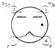
Glass type used to supply dc power of uniform voltage to receivers in which the rectified current requirements are subject to considerable variation. Outline 43, OUTLINES SECTION. Tube requires four-contact socket and should be mounted in vertical position with base down. Filament volts (ac), 2.5; amperes, 3. Maximum ratings for full-wave rectifier service: peak in-
