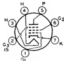
**OUTLINES SECTION.** Tube requires miniature seven-contact socket and may be mounted in any position. For a discussion of limiters, refer to **ELECTRON TUBE APPLICATIONS SECTION**. For typical operation as resistance-coupled amplifier, refer to Chart 4, **RESISTANCE-COUPLED AMPLIFIER SECTION**.
