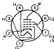
0.6; warm-up time (average), 11 seconds. Peak heater-cathode volts: heater negative with respect to cathode, 300 *max*; heater positive with respect to cathode, 200 *max* (the dc component must not exceed 100 volts). Except for heater and heater-cathode ratings, this type is identical with miniature type 6CB6.
