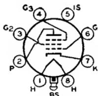
*max* watts; grid-No.2 input, 0.75 *max* watt; grid No.3 and internal shield connected to cathode at socket; plate resistance (approx.), greater than 1 megohm; transconductance, 4200  $\mu$ mhos; cathode-bias resistor, 250 ohms; plate ma., 6; grid-No.2 ma., 2; peak heater-cathode volts, 90 *max*. This type is used principally for renewal purposes.
