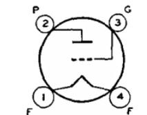
detector: plate volts, 180; grid volts, -21. This is a DISCONTINUED type listed for reference only.
