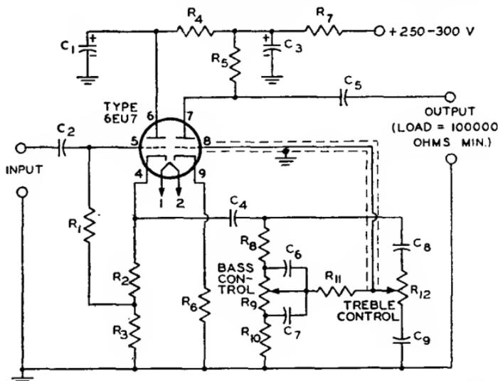
$C_1, C_3 = 20 \mu\text{f}$ , electrolytic, 450 v.
