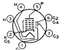
Miniature type used as a gated amplifier in television receivers. In such service, it may be used as a combined sync separator and sync clipper. Outline 11, OUTLINES SECTION.
