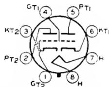
octal socket and may be mounted in any position. Except for the common heater, each triode unit is independent of the other. For typical operation as phase inverter or resistance-coupled amplifier, refer to Chart 3, **RESISTANCE-COUPLED AMPLIFIER SECTION**.
