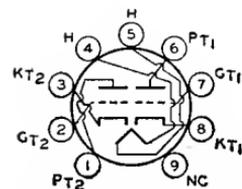
LINES SECTION. Tube requires miniature nine-contact socket and may be mounted in any position.
