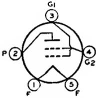
ductance, 1125  $\mu$ mhos; load resistance, 11000 ohms; output watts (approx.), 0.17. This is a DISCONTINUED type listed for reference only.
