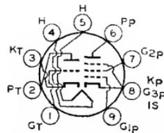
Miniature types used in a wide variety of applications in color and black-and-white television receivers. Especially useful as combined triode oscillator and pentode mixer in vhf
