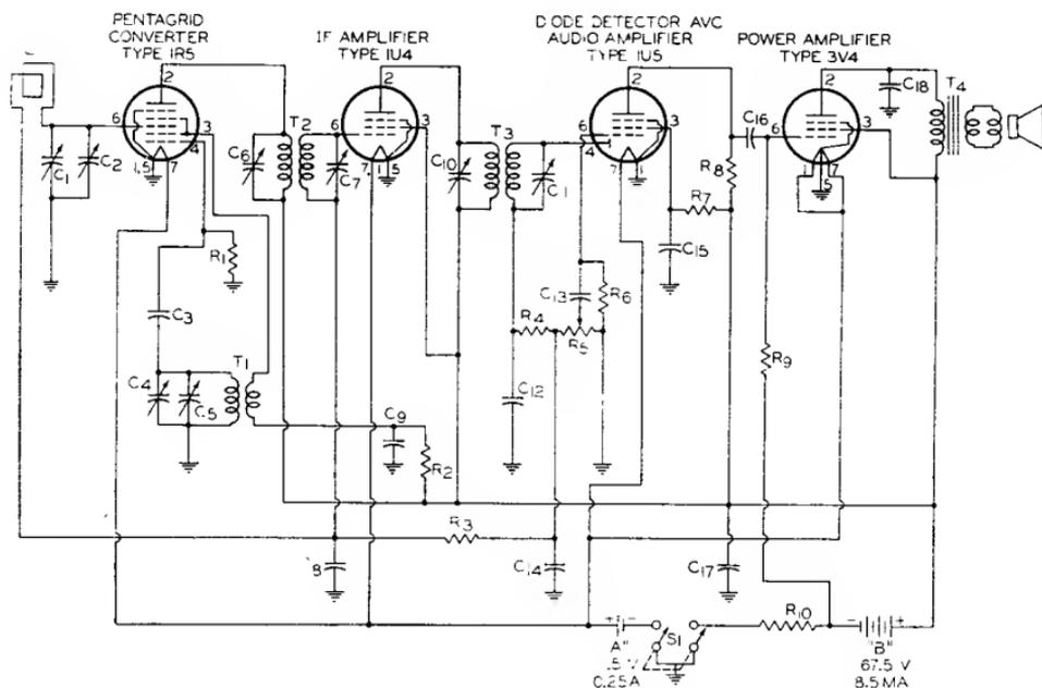
$C_1$   $C_4$  = Ganged tuning capacitors:  $C_1$ , 10-27.4  $\mu\text{f}$ ;  $C_4$ , 7.5-122.5  $\mu\text{f}$
