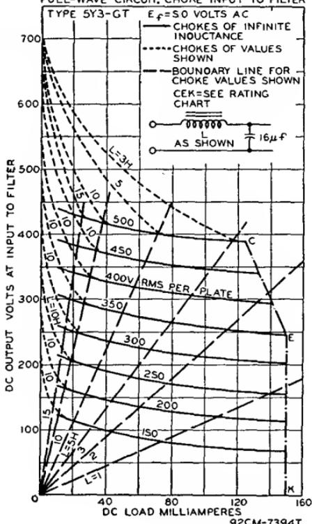
Typical Operation of 5Y3-GT with Choke Input to Filter:
