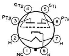
signal plate ma. per plate, 4.2; plate-to-plate load resistance, 12000 ohms; output watts, 4.2 with average input of 320 milliwatts applied between grids. This is a DISCONTINUED type listed for reference only.
