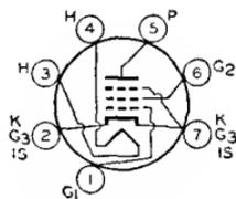
OUTLINES SECTION. Tube requires miniature seven-contact socket and may be mounted in any position.
