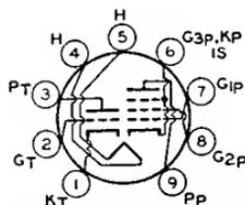
Miniature type used in television receivers employing series-connected heater strings. Pentode unit is used as video amplifier; triode unit is used in sound if amplifier, sweep-oscillator, sync-separator, sync-amplifier, and sync-clipper circuits. Outline 14, OUTLINES SECTION. Heater volts (ac/dc), 8; amperes, 0.6; warm-up time (average), 11 seconds. Except for heater rating, this type is identical with type 6CX8.
