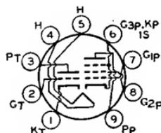
verter circuits. Outline 14, OUTLINES SECTION. Tube requires miniature nine-contact socket and may be mounted in any position.
