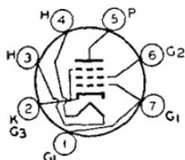
Miniature type used in output stage of compact, ac/dc radio receivers. Because of its high power sensitivity at plate and screen-grid voltages available in ac/dc receivers, it is capable of providing a relatively high power output. Outline 13, OUTLINES SECTION. Tube
