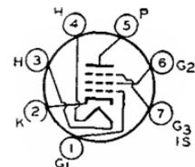
cause of its plate-current cutoff characteristic, this type is used in gain-controlled stages of video if amplifiers. This type is electrically similar to miniature type 6CB6. Outline 11, OUTLINES SECTION. Heater volts (ac/dc), 6.3; amperes, 0.3.
