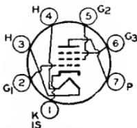
OUTLINES SECTION. Heater volts (ac/dc), 3.15; amperes, 0.6; warm-up time (average), 11 seconds. Peak heater-cathode volts, 200 max. When the heater is positive with respect to the cathode, the dc component of the heater-cathode voltage must not exceed 100 volts. Except for heater and heater-cathode ratings, this type is identical with miniature type 6BN6.
