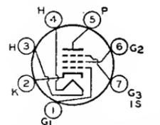
Miniature type used in gain-controlled video if stages of television receivers employing series-connected heater strings. Outline 11, OUTLINES SECTION. Heater volts (ac/dc), 4.2;
