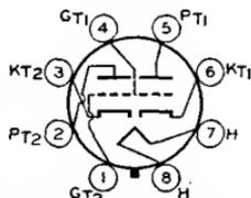
5, and 6) be used as the oscillator. Outline 22, OUTLINES SECTION. Tubes require octal socket and may be mounted in any position. Type 6BL7-GT is a DISCONTINUED type listed for reference only.
