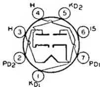
Miniature, high-perveance type used as detector in FM and television circuits. It is especially useful as a ratio detector in ac/dc FM receivers. Outline 9, OUTLINES SECTION. Heater volts (ac/dc), 12.6; amperes, 0.15. Except for heater rating, this type is identical with miniature type 6AL5.
