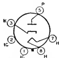
strings. Outline 22, OUTLINES SECTION. These types may be supplied with pin No.1 omitted. Heater volts (ac/dc), 12.6; amperes, 0.6; warm-up time (average) for 12AX4-GTA, 11 seconds. Except for heater rating, these types are identical with glass octal type 6AX4-GT. Type 12AX4-GT is a DISCONTINUED type listed for reference only.
