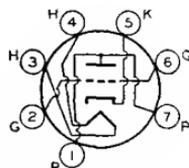
0.6; warm-up time (average), 11 seconds. Except for heater rating, this type is identical with miniature type 6AF4-A.
