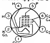
Heater volts (ac/dc), 3.15; amperes, 0.6; warm-up time (average), 11 seconds. Except for heater rating, this type is identical with miniature type 6BY6.
