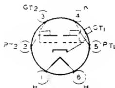
Glass type used in output stage of radio receivers as a class B power amplifier or a class A<sub>1</sub> driver. Outline 40, OUTLINES SECTION. Tube requires six-contact socket. Heater volts (ac/dc), 6.3; amperes, 0.6. Maximum ratings and typical operation as class B power amplifier: plate volts, 250 *max*; grid volts, 0; zero-signal plate ma., 10.5; effective load resistance
