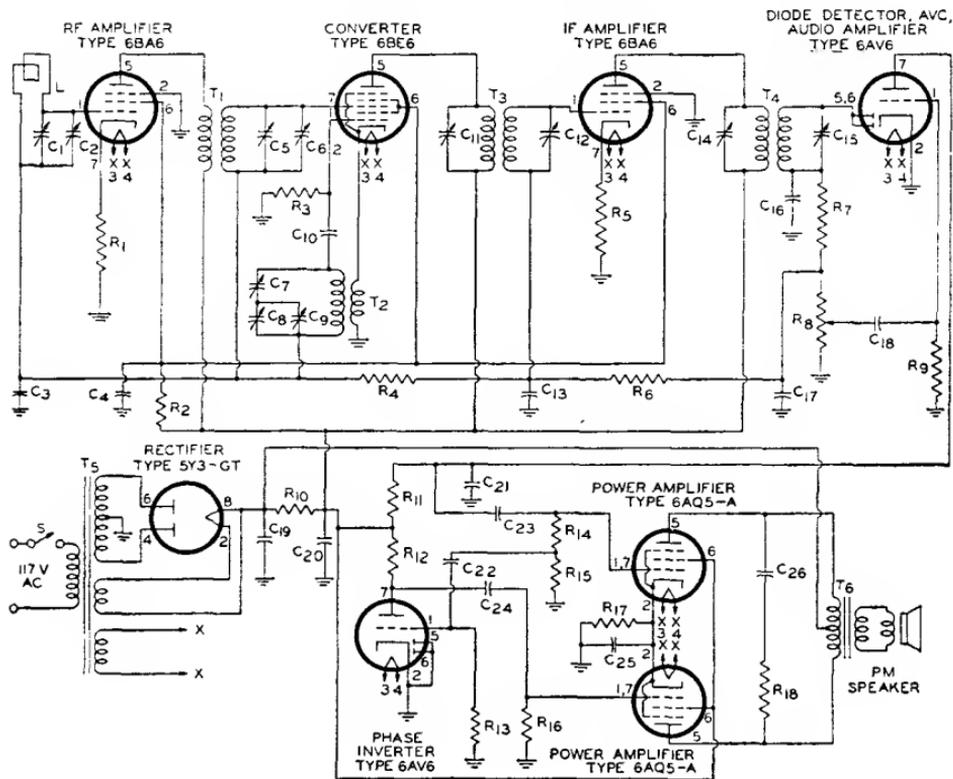
$C_1 C_3$  = Ganged tuning capacitors, 10-365  $\mu\text{f}$
