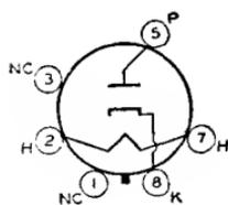
Glass octal type used in power supply of ac/dc receivers. Outline 22, OUTLINES SECTION. Tube requires octal socket. This type may be supplied with pin No.1 omitted. Heater volts (ac/dc), 35; amperes, 0.15. For maximum ratings and typical operation, refer to glass octal type 35Z5-GT without panel lamp. Type 35Z4-GT is used principally for renewal purposes.
