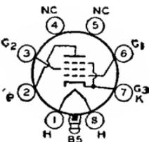
Glass lock-in type used as output amplifier in radio receivers. Outline 20, OUTLINES SECTION. Tube requires lock-in socket. Heater volts (ac/dc), 6.3; amperes, 0.45. Refer to metal type 6V6 for maximum ratings and typical operation as class A<sub>1</sub> amplifier and as push-pull class A<sub>1</sub> amplifier. Type 7C5 is used principally for renewal purposes.
