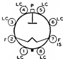
Glass octal type used in high-voltage, low-current applications such as the rectifier in a high-voltage, rf-operated power supply or as a rectifier of high-voltage pulses produced in television scanning systems. For curve of average plate characteristics, see page 67.
