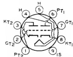
Miniature type used in direct-coupled, cathode-drive, rf amplifier circuits in vhf television tuners. In such circuits, one triode unit is used as the direct-coupled, grounded-cathode
