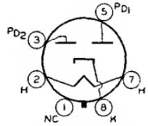
Tube requires octal socket and may be mounted in any position. It is especially important that this tube, like other power-handling tubes, be adequately ventilated.
