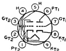
Miniature type used as combined vertical-deflection-oscillator and vertical-deflection-amplifier tube in television receivers. Outline 14, OUT-LINES SECTION. Tube requires miniature nine-contact socket and may be operated in any position.
