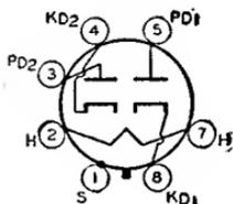
Metal type used as detector, low-voltage rectifier, or avc tube in ac/dc radio receivers. Outline 1, OUTLINES SECTION. Heater volts (ac/dc), 12.6; amperes, 0.15. Except for heater rating, this type is identical with metal type 6H6.
