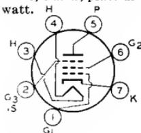
Miniature type used as rf amplifier in standard broadcast and FM receivers, as well as in wide-band, high-frequency applications. This type is similar in performance to metal type
