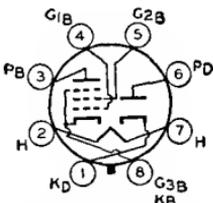
volts, 5.2; plate ma., 43; grid-No.2 ma., 4 (zero-signal); 5.5 (maximum-signal); plate input, 6 *max* watts; grid-No.2 dissipation, 1 *max* watt; plate resistance (approx.), 17000 ohms; transconductance, 5300  $\mu$ mbos; load resistance, 4000 ohms; total harmonic distortion, 5 per cent; maximum-signal power output, 0.85 watt. Type 117L7/M7-GT is used principally for renewal purposes.
