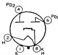
any position. Heater volts (ac), 5.0; amperes, 2.0. Maximum ratings: peak inverse plate volts, 1400 *max*; peak plate ma. per plate, 375 *max*. Typical operation as full-wave rectifier with capacitor-input filter: ac plate-to-plate supply volts (rms), 700; total effective plate-supply impedance per plate, 50 ohms; dc output ma., 125. Typical operation with choke-input filter: ac plate-to-plate supply volts, 1000; minimum filter-input choke, 5 henries; dc output ma., 125.
