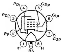
Glass lock-in type used as combined detector, amplifier, and avc tube in ac/dc receivers. Outline 15, OUTLINES SECTION. Tube requires lock-in socket. Heater volts (ac/dc), 12.6; amperes, 0.15. Except for heater rating, this type is electrically identical with lock-in type 7E7. Type 14E7 is a DISCONTINUED type listed for reference only.
