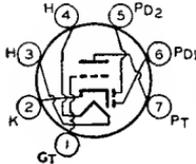
Miniature type used as combined detector and af voltage amplifier in automobile radio receivers operating from a 12-volt storage battery. Outline 11, OUTLINES SECTION. Tube requires miniature seven-contact socket. Heater-voltage range (ac/dc), 10 to 15.9 volts; amperes at 12.6 volts, 0.15. Characteristics with heater volts of 12.6 and maximum ratings of triode unit as class A<sub>1</sub> amplifier: plate volts, 12.6 (30
