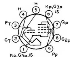
Miniature type used as combined oscillator and mixer tube in vhf tuners of television receivers having series-connected heater strings. Outline 12, **OUTLINES SECTION**. Tube requires nine-contact socket and may be mounted in any position.
