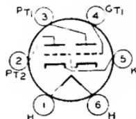
Glass type used as class A<sub>1</sub> power amplifier. One triode, the driver, is directly connected within the tube to the second, or output, triode. Heater volts (ac/dc), 25; amperes, 0.3. Maximum ratings and characteristics are the same as for type 25N6-G. Type 25B5 is a DISCONTINUED type listed for reference only.
