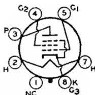
and may be mounted in any position. Heater volts (ac/dc), 12.6; amperes, 0.225. Except for heater rating, this type is identical with glass octal type 6V6-GT.
