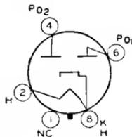
mounted in any position. The heater is designed to operate from the ac line through a step-down transformer. The voltage at the heater terminals should be 5.0 volts under operating conditions at an average line voltage of 117 volts. It is especially important that these tubes, like other power-handling tubes, be adequately ventilated. Type 5V4-G is used principally for renewal purposes.
