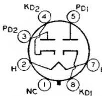
cathode volts, 350 *max*. Typical operation as half-wave rectifier with capacitor-input filter or as half-wave or full-wave voltage doubler: ac plate supply volts per plate (rms), 117; filter-input capacitor, 50  $\mu$ f; minimum total effective plate-supply impedance per plate, 15 (30 for half-wave doubler service); dc output ma. per plate, 60. This type is used principally for renewal purposes.
