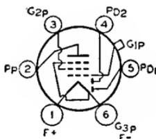
Glass type used as combined detector, amplifier, and avc tube in battery-operated receivers. Outline 39, OUTLINES SECTION. Tube requires six-contact socket. Filament volts (dc), 2.0; amperes, 0.06. Typical operation of pentode unit as class A<sub>1</sub> amplifier: plate volts, 180 *max*; grid-No.2 (screen-grid) volts, 67.5 *max*; grid-No.1 volts, -1.5; plate ma., 2.2; grid-No.2 ma., 0.7. This is a DISCONTINUED type listed for reference only.
