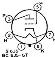
high amplification factor. Outlines 3 and 24, respectively, **OUTLINES SECTION**. Tubes require octal socket and may be mounted in any position. For typical operation as resistance-coupled amplifiers, refer to Chart 6, **RESISTANCE-COUPLED AMPLIFIER SECTION**.
