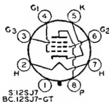
Heater volts (ac/dc), 12.6; amperes, 0.15. Except for heater rating, these types are identical with metal type 6SJ7 and glass-octal type 6SJ7-GT. Type 12SJ7-GT is a **DISCONTINUED** type listed for reference only.
