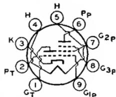
trolled heater warm-up time for use in receivers employing series-connected heater strings. Outline 12, OUTLINES SECTION. Except for interelectrode capacitances and basing arrangement, these types are identical with miniature type 6X8. The basing arrangement of the 6AT8 and 6AT8-A is particularly suitable for connection to the coils of certain designs of turret tuners. Type 6AT8 is a DISCONTINUED type listed for reference only.
