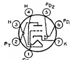
requires miniature seven-contact socket and may be mounted in any position.
