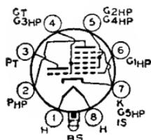
Glass lock-in type used as combined triode oscillator and heptode mixer in ac/dc radio receivers. Outline 15, OUTLINES SECTION. Tube requires lock-in socket. Heater volts (ac/dc), 12.6; amperes, 0.15. Except for heater rating, this type is electrically identical with lock-in type 7J7. Type 14J7 is a DISCONTINUED type listed for reference only.
