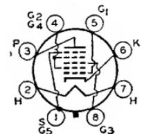
Metal type 12SA7 and glass octal type 12SA7-GT used as converter in ac/dc receivers. Outlines 3 and 22, respectively, OUTLINES SECTION. Heater volts (ac/dc), 12.6; amperes, 0.15. Except for heater ratings, these types are identical with metal type 6SA7 and glass octal type 6SA7-GT. Type 12SA7-GT is used principally for renewal purposes.
