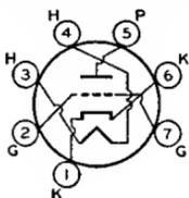
Miniature type used as rf amplifier in grid-drive circuits of vhf television tuners. The double base-pin connections for both cathode and grid reduce effective lead inductance and
