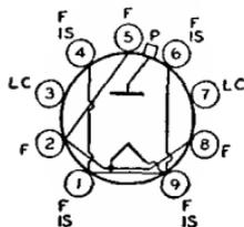
vision scanning systems. Outlines 16 and 17, respectively, **OUTLINES SECTION**. Tubes require miniature nine-contact socket and may be mounted in any position. Socket terminals 3 and 7 may be used as tie points for components at or near filament potential. For high-voltage considerations, refer to type 1B3-GT. For curve of average plate characteristics, see page 67. Type 1X2-A is used principally for renewal purposes.
