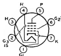
*max*); grid-No.1 volts, -3; plate resistance (approx.), 0.8 megohm; transconductance, 2000  $\mu$ hos; plate dissipation, 3 *max* watts; grid-No.2 input, 0.65 *max* watt; plate ma., 9; grid-No.2 ma., 3; total cathode ma., 14 *max*; peak heater-cathode volts, 90 *max*. This type is used principally for renewal purposes.
