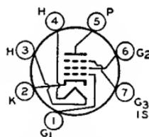
controlled plate-current cutoff and high transconductance (14000  $\mu$ mhos) combined with low interelectrode capacitance values. The 6EW6 is provided with separate base pins for grid No.3 and cathode to permit the use of an unbypassed cathode resistor to minimize changes in input conductance and input capacitance with bias, without causing oscillation. Outline 11, OUTLINES SECTION. Tube requires miniature seven-contact socket and may be mounted in any position.
