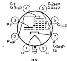
Glass lock-in type used as combined oscillator and heptode mixer in radio receivers. Outline 15, OUTLINES SECTION. Tube requires lock-in socket. Heater volts (ac/dc), 6.3; amperes, 0.3. For maximum ratings and typical operation, refer to glass-octal type 6J8-G. Type 7J7 is used principally for renewal purposes.
