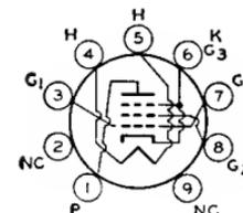
Miniature type used in audio output stages of television and radio receivers. Also used as video amplifier. Outline 14, OUTLINES SECTION. Heater volts (ac/dc), 25; amperes, 0.3. Except for heater rating, this type is identical with miniature type 6BK5.
