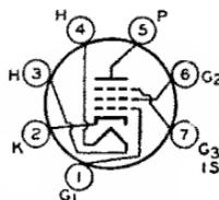
LINES SECTION. Tube requires seven-contact miniature socket and may be mounted in any position.
