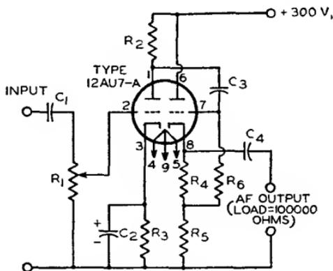
$C_1, C_3 = 0.1 \mu\text{f}$ , paper, 400 v.
