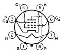
and may be mounted in any position. Two separate cathode terminals enable the input and output circuits to be isolated effectively from each other. This type is not recommended for high-gain audio-amplifier applications because undesirable hum may be encountered. For typical operation as a resistance-coupled amplifier, refer to Chart 4, RESISTANCE-COUPLED AMPLIFIER SECTION.
