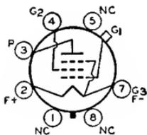
Glass octal type used as rf amplifier or detector in battery-operated receivers. Outline 39, OUTLINES SECTION. \*Tube requires octal socket. Filament volts (dc), 2.0; amperes, 0.06. Characteristics as class A<sub>1</sub> amplifier: plate volts, 180 *max*; grid-No.2 volts, 67.5 *max*; grid-No.1 volts, -3; plate ma., 1.7; grid-No.2 ma., 0.6; plate resistance, 1.5 megohms; transconductance, 650  $\mu$ hos. This is a DISCONTINUED type listed for reference only.
