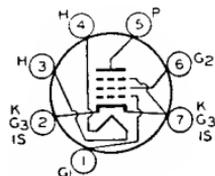
seven-contact socket and may be mounted in any position. For typical operation as resistance-coupled amplifier, refer to Chart 13, RESISTANCE-COUPLED AMPLIFIER SECTION.
