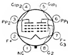
Glass octal type used in push-pull output stage of battery-operated receivers. Outline 22, OUTLINES SECTION. Tube requires octal socket. Filament volts (dc), 2.0; amperes, 0.24. Typical operation as push-pull class A<sub>1</sub> amplifier: plate and grid-No.2 volts, 135 *max*; grid-No.1 volts, -7.5; plate ma., 10.5; grid-No.2 ma., 3.5; output watts, 0.575. This is a DISCONTINUED type listed for reference only.
