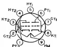
miniature nine-contact socket and may be mounted in any position. Each triode unit is independent of the other except for the common heater. For typical operation as a resistance-coupled amplifier, refer to Chart 10, RESISTANCE-COUPLED AMPLIFIER SECTION.
