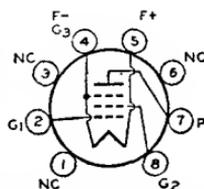
No.1 volts, 4.5; zero-signal plate ma., 2; zero-signal grid-No.2 ma., 0.4; cathode ma., 4 max; plate resistance, 0.15 megohm; transconductance, 750  $\mu$ mhos; load resistance, 25000 ohms; total harmonic distortion, 10 per cent; maximum-signal power output, 50 milliwatts. This is a DISCONTINUED type listed for reference only.
