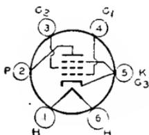
Glass type used in output stage of radio receivers. Outline 34 or 35, OUTLINES SECTION. Tube requires six-contact socket. Heater volts (ac/dc), 6.3; amperes, 0.4. This type is electrically identical with type 6K6-GT. Type 41 is used principally for renewal purposes.
