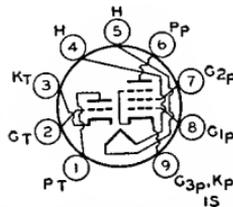
is used in vertical-deflection-oscillator, sync-separator, sync-clipper, and sync-amplifier circuits. Outline 12, OUTLINES SECTION. Tube requires miniature nine-contact socket and may be mounted in any position.
