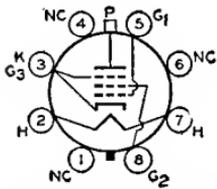
18.9; amperes, 0.3. Except for heater rating and interelectrode capacitances, type 19BG6-GA is electrically identical with glass octal type 6BG6-G. Type 19BG6-G is a DISCONTINUED type listed for reference only. Type 19BG6-GA is used principally for renewal purposes.
