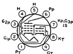
Miniature type used in multivibrator-type horizontal-deflection circuits in television receivers employing a series heater-string arrangement. Also used for agc-amplifier or sync-separator applications in such receivers. Outline 12, OUTLINES SECTION. Tube requires miniature nine-contact socket and may be mounted in any position.
