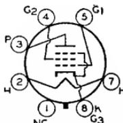
No.1 omitted. Heater volts (ac/dc), 4.7; amperes, 0.6; warm-up time (average), 11 seconds. Except for heater rating, this type is identical with glass octal type 6V6-GT.
