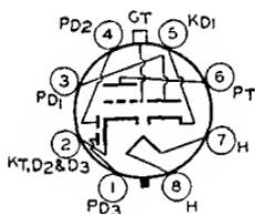
Glass octal type used as audio amplifier, AM detector, and FM detector in AM/FM receivers. Outline 21, OUTLINES SECTION, except over-all length is 3-9/16 *max* inches and seated height is 3 *max* inches. Heater volts (ac/dc), 12.6; amperes, 0.15. Except for heater rating, this type is identical with glass octal type 6S8-GT. Type 12S8-GT is a DISCONTINUED type listed for reference only.
