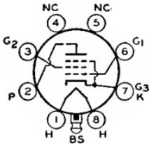
Glass lock-in type used in output stage of ac/dc receivers. Outline 20, OUTLINES SECTION. Tube requires lock-in socket. Heater volts (ac/dc), 50; amperes, 0.15. For ratings and data, refer to glass-octal type 50L6-GT. Type 50A5 is used principally for renewal purposes.
