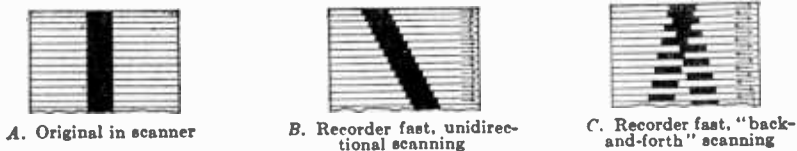
Fig. 23—Recorder not perfectly synchronized.
