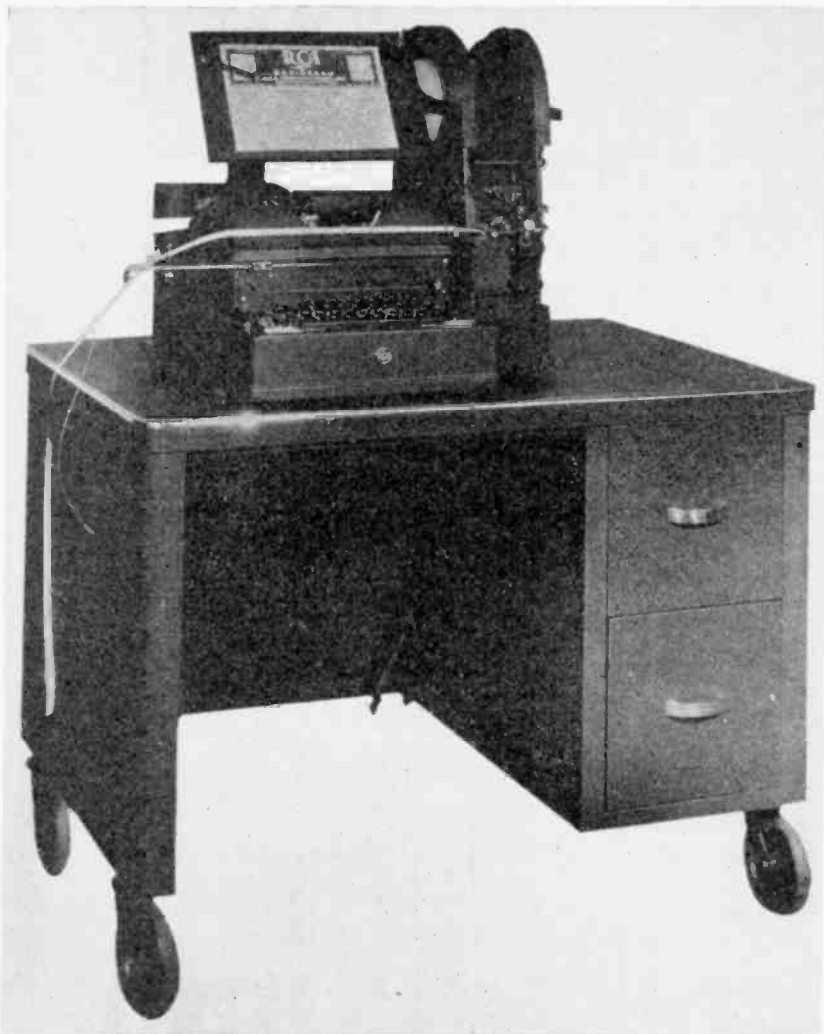
Fig. 8—Special tape facsimile typewriter and transmitter.
