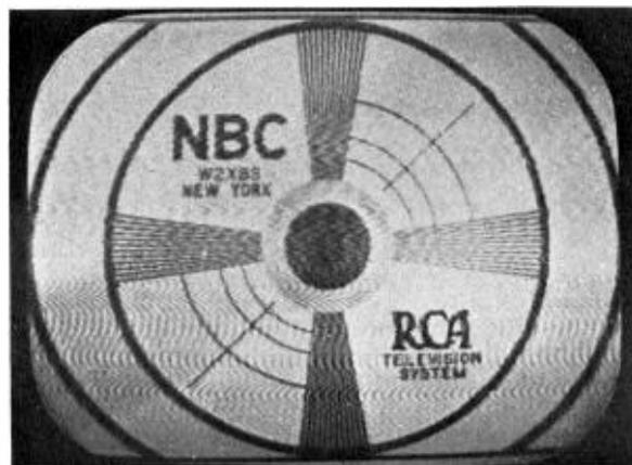
Figure 45—Excessive Diathermy Interference
