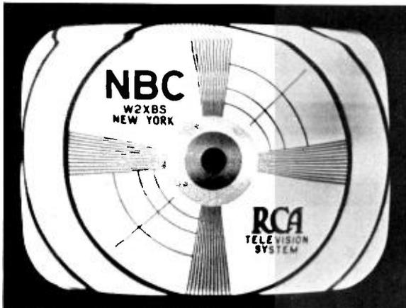
**Figure 52—Unstable—“Tear-Out”—Horizontal Synchronization**
