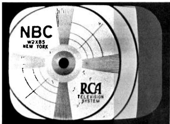
**Figure 36—Horizontal Centering Control Incorrectly Set**
