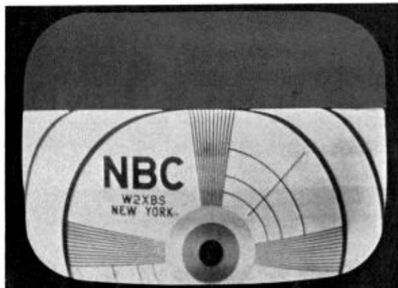
**Figure 38—Vertical Centering Control Incorrectly Set**
