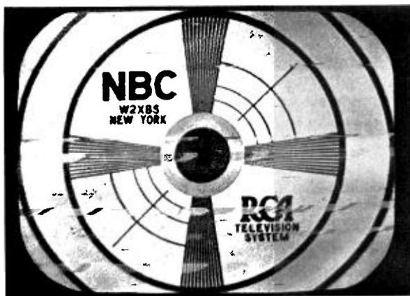
Figure 44—Excessive Auto Ignition Interference
