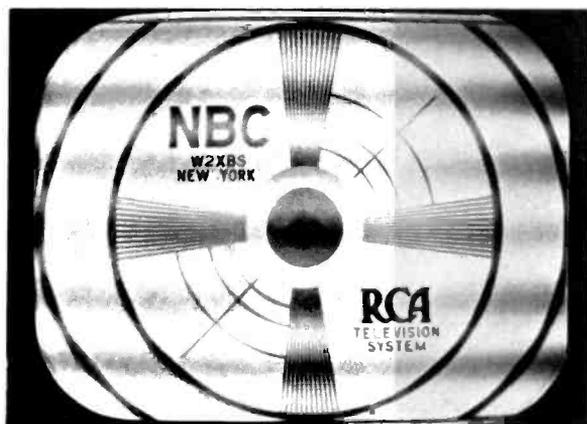
**Figure 33—Sound Modulation in Picture**
