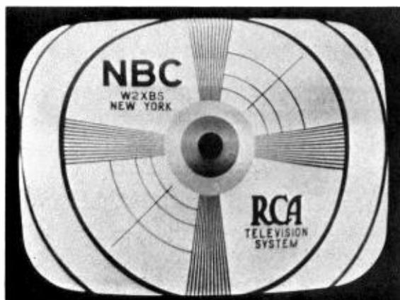
**Figure 41—Vertical Linearity Control Incorrectly Set**
