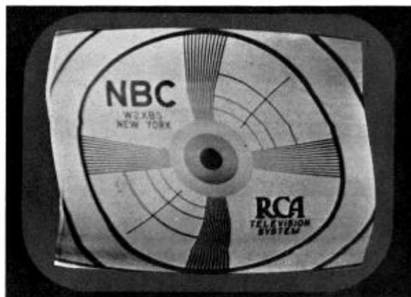
Figure 47—Excessive Ripple in Horizontal Deflection
