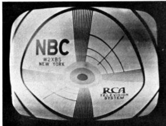
**Figure 54—Excessive Ripple in Vertical Deflection**
