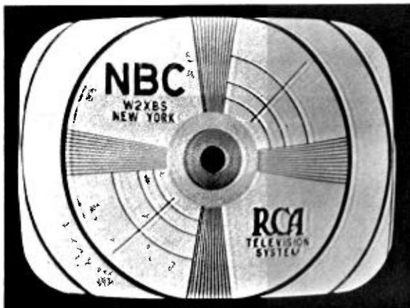
Figure 56—Transients in Test Pattern
