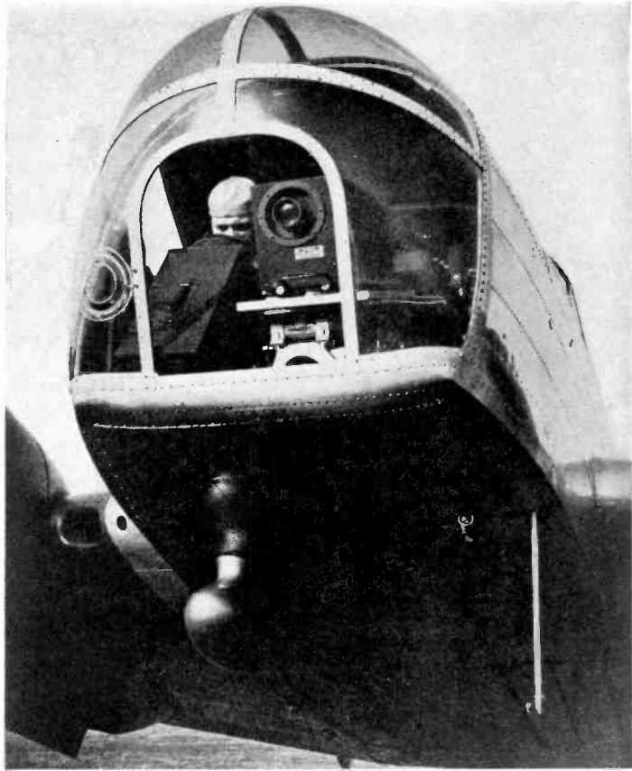
Mounted in the nose of an airplane, special RCA airborne television equipment gives ground observers a bird's-eye view of great areas of land or sea as the pilot sees them.
