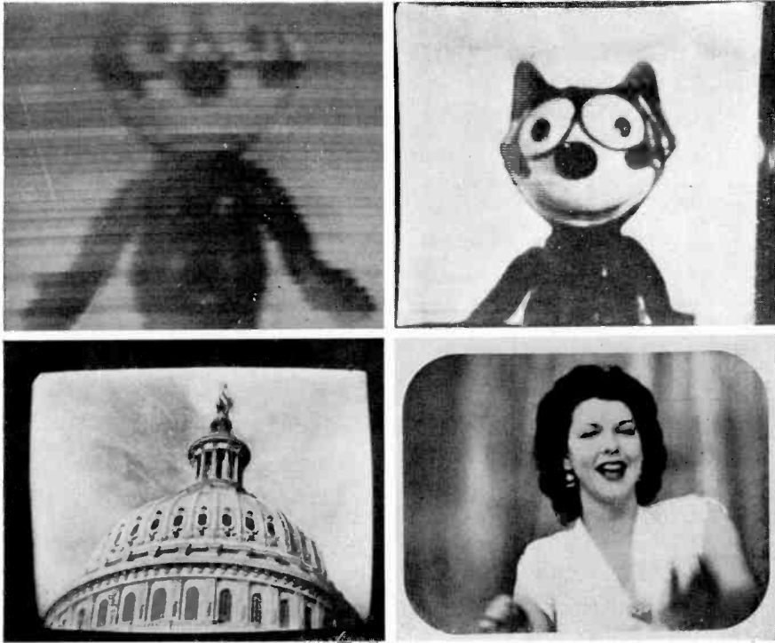
By increasing the number of scanning lines in each picture frame, the detail and definition in television images have been vastly improved. This series of photographs shows, upper left, 60-line definition; upper right, 120-line; lower left, 441-line, and lower right, 525-line.
