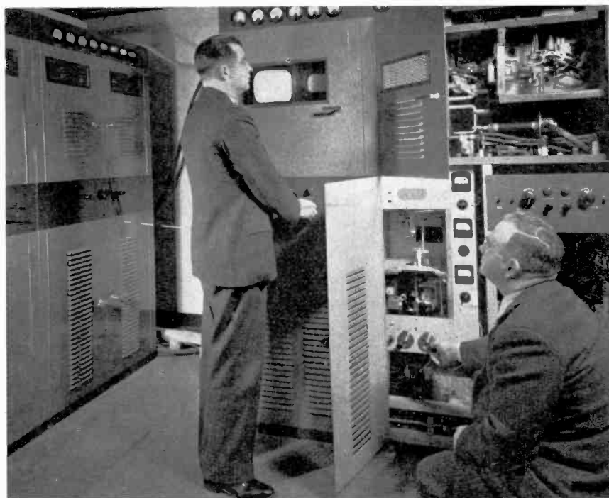
Left — The appearance of NBC's futuristically designed television antenna atop the Empire State Tower in New York was changed in the Fall of 1945 by the addition of new structure (right) to enable field tests of a new RCA 288-megacycle video transmitter. Below— The new high-frequency transmitter.
