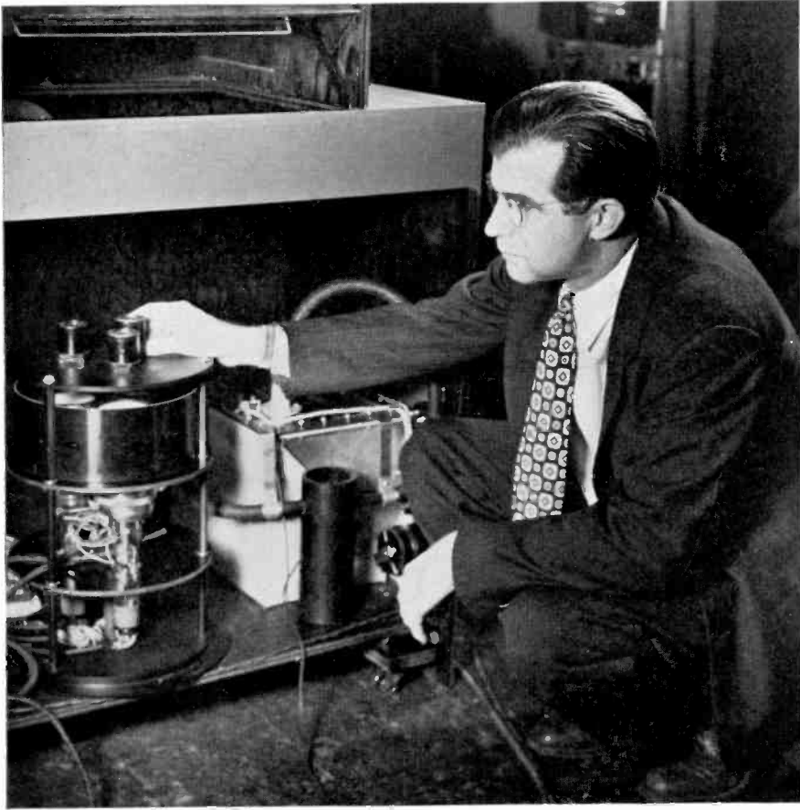
Ray D. Kell, engineer in charge of research on television equipment at RCA Laboratories, points to the Trinoscope in RCA's all-electronic color television receiver.
