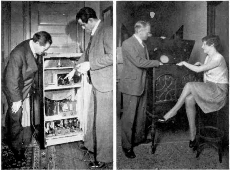
Left — A neon lamp, just above motor, “painted” images on the screens of 1928 television receivers. Right — In 1929, Dr. V. K. Zworykin demonstrated his all-electronic television receiver.
