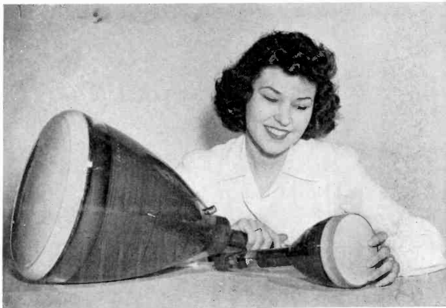
RCA television picture tubes, prewar at the left and postwar at right.
