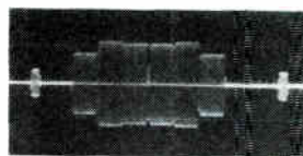
Fig. 18(a) - CA3071 chroma input 1.25 V p-p ; one horizontal line of NTSC input signal.
