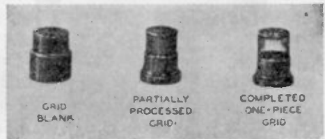
Fig. 8—Fabrication of one-piece grid.
