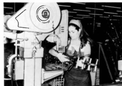
Fig. 6—Automated riveting operation.
