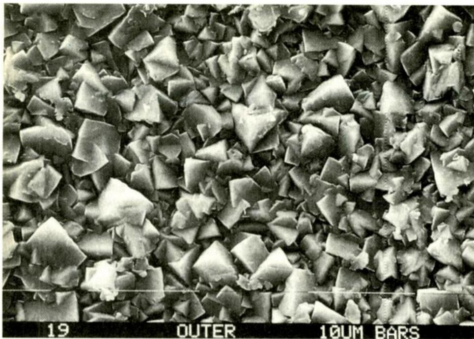
*Pilkington Electro-optic Materials has combined high-energy plasma and chemical vapour deposition to coat variety of surfaces with polycrystalline diamond.*
