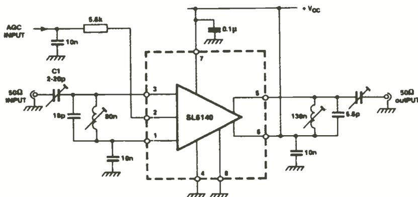
amplifier to increase gain; power gain in the circuit shown is 35dB. Input and output coupling trimmers optimise gain, but too high a reflected impedance at the amplifier terminals could give rise to oscillation. Gain is traded for bandwidth.
