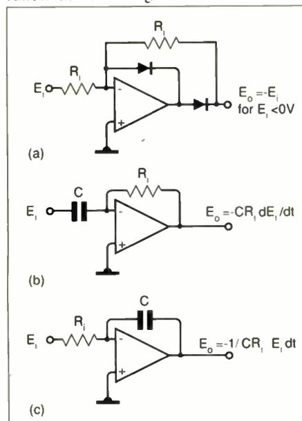
Fig. 6. (a) Suitable precision block for halfwave rectification. (b) differentiation (c) integration.
