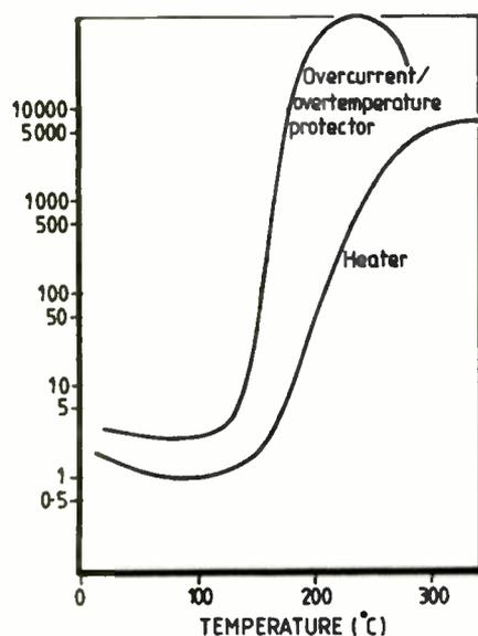
Fig. 2. PTC applications. The steep PTC curve is required for over-current and thermal fuse applications, where the current needs to be switched off quickly. The shallow curve, on the other hand, is more suitable for heaters, where there is a gradual reduction in current as temperature rises.
