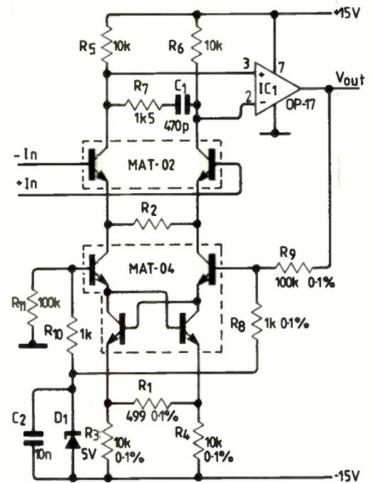
Fig. 4. Low-noise high speed instrumentation amplifier (PMI application note AN-105) shown here, with some minor changes, is implemented by using the linearised cross-quad circuit as a precision differential output voltage-to-current converter.
