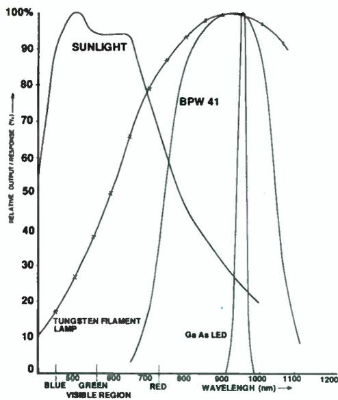
Fig. 2. Spectral response of The BPW41 with some common light sources.
