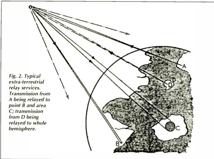
**Fig. 2. Typical extra-terrestrial relay services. Transmission from A being relayed to point B and area C; transmission from D being relayed to whole hemisphere.**
