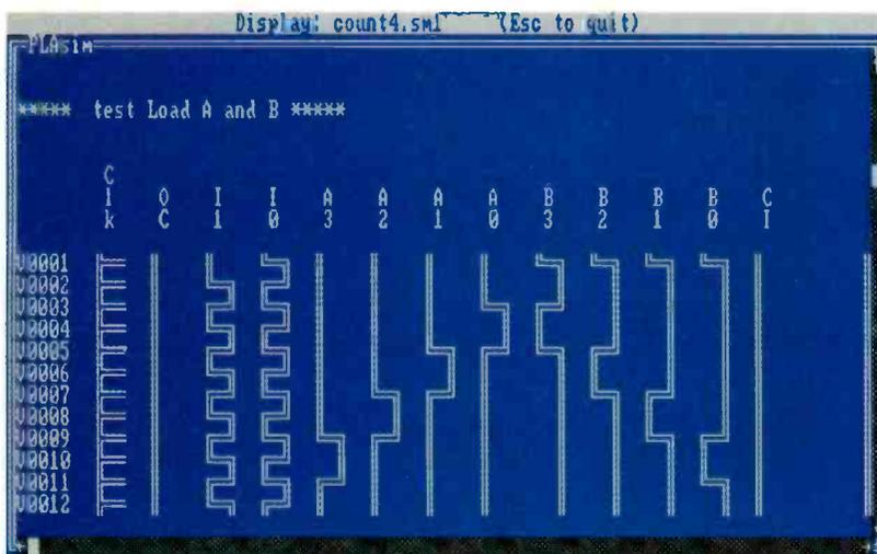
Fig. 5. Pix simulation with waveform output is one of the display choices.
