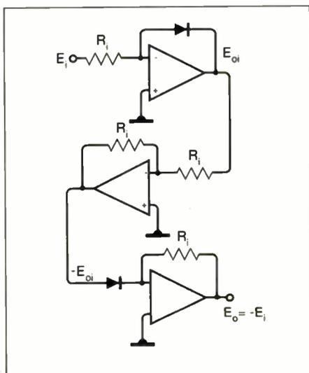
Fig. 3. Taking logs and antilogs.
