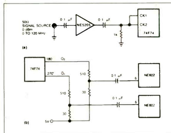
Fig. 5. You can effectively drive the 74F74 and other TTL gates with the circuit shown in (a). The total resistance in the interface circuit (b) establishes a conservative current drain (approximately 10mA) from the 74F74, and the divider tap optimises NE602 operation.
