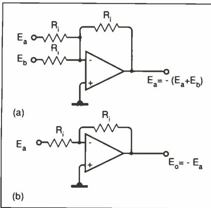
Fig. 1. Basic SAE functions; (a) addition and (b) negation.
