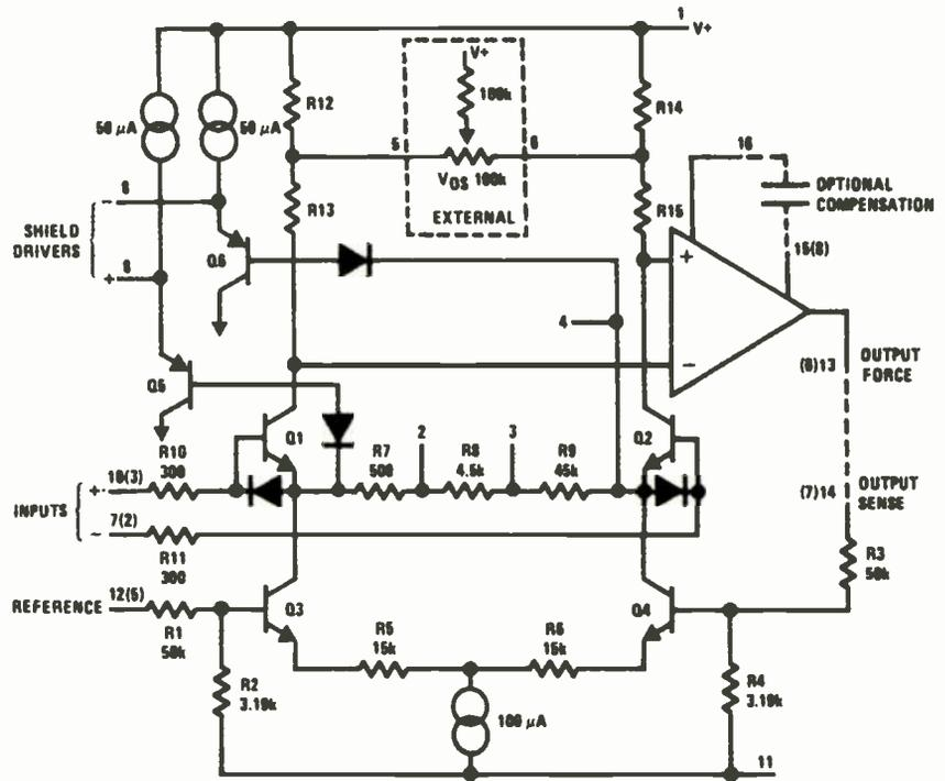
Fig.1. Skeleton circuit diagram of National Semiconductor's LM363 instrumentation amplifier. Two-stage amplifier yields extremely high open-loop gain and gain/bandwidth product, but remains stable at all closed-loop gains.
