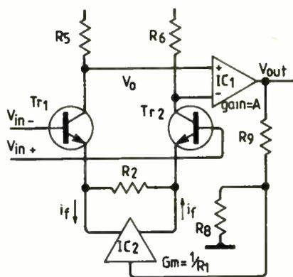
Fig. 3. The cross-quad is represented by the transconductance amplifier  $U_2$ , having  $G_m = 1/R_1$ , which feeds currents  $-i_f$  and  $+i_f$  into the input stage.
