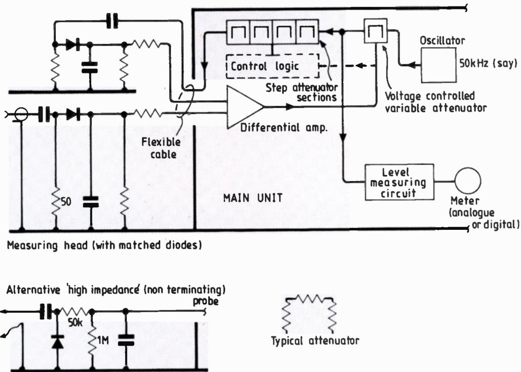
Fig. 3. Accurate RF level measurement requires linearisation of the diode response. This can be done by using a dummy diode and separate RF reference source for comparison with the rectified level of the signal under test.
