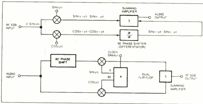
**Fig. 2. The input signal feeds in phase to two RF mixers in the phasing-method detector (a). A local oscillator (LO) supplies a second signal to the mixers in quadrature. In the generator (b), a divide-by-4 flip-flop provides the  $\sin(yt)$  and  $\cos(yt)$  signals for the mixer.**
