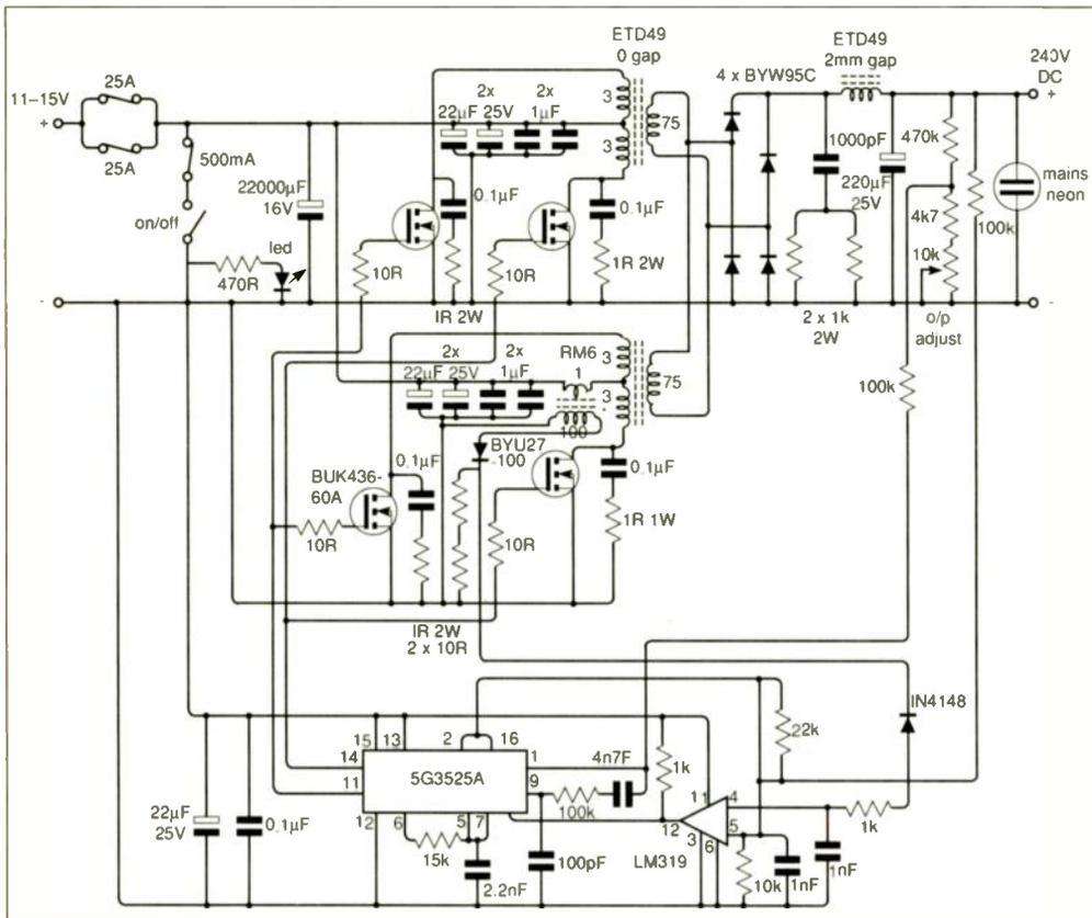
**250V, 500W inverter using power mosfets.** Equivalents to the SGS-Thomson device are obtainable from Linear Technology, Motorola, National Semiconductor, Sprague and Unitrode.
