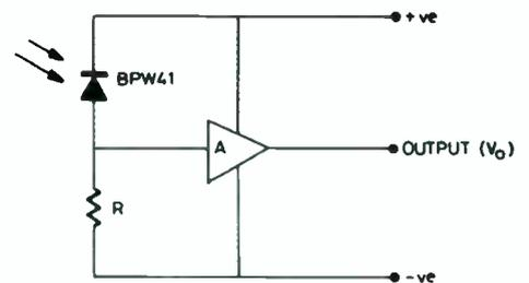
Fig. 3. A commonly used single resistor is the simplest load.
