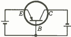
Fig. 1. Bipolar transistor in common-base mode.
