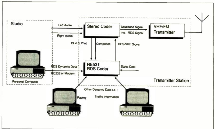
Fig. 2. An RDS network configuration downloading data from PCs to the coder.
