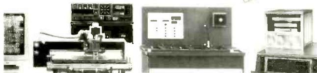
CAD → Milling/Drilling Prototypes → Through Plating → MULTIPRESS
