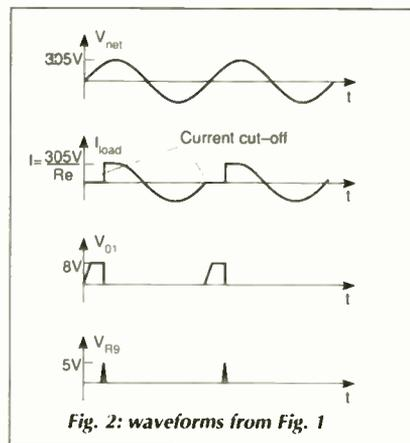
Fig. 2: waveforms from Fig. 1
