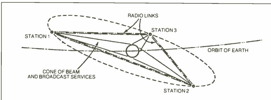
**A project which goes part of the way towards the goal envisaged in this article has been put forward by Westinghouse in collaboration with the Glen L Martin Co of America. The radius of coverage would be increased from 50 to 211 miles by beamed radiation from an aircraft flying at a height of 30,000ft and equipped with television and FM transmitters.**
