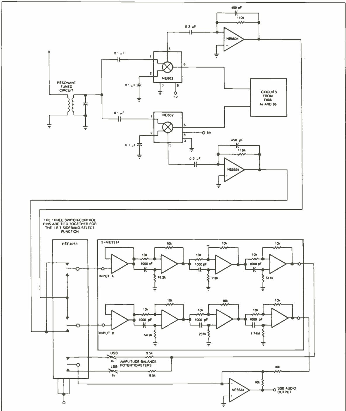
Fig. 7. Using the phasing filter technique, you can design a complete, yet simple, SSB receiver. The antenna connects directly (via a bandpass filter) to the inputs of the NE602s' mixer stage.
