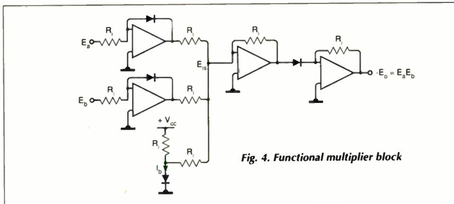
Fig. 4. Functional multiplier block
