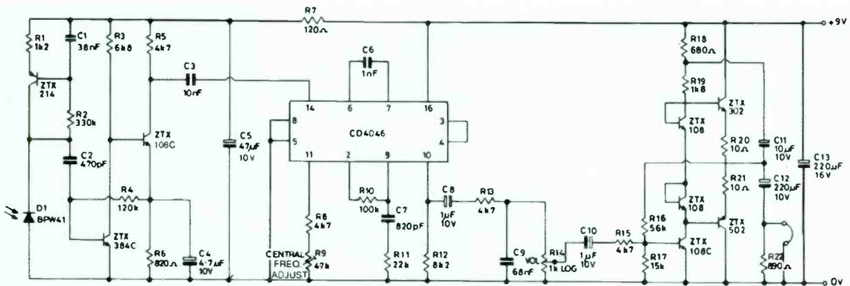
amplifier stage. Consequently the range can be easily extended by either raising the amplifier gain by adding further stages or by increasing the received signal level using a lens with the transmitter led. An experimental system using both techniques operates at over 40m.
