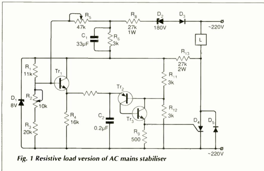
Fig. 1 Resistive load version of AC mains stabiliser
