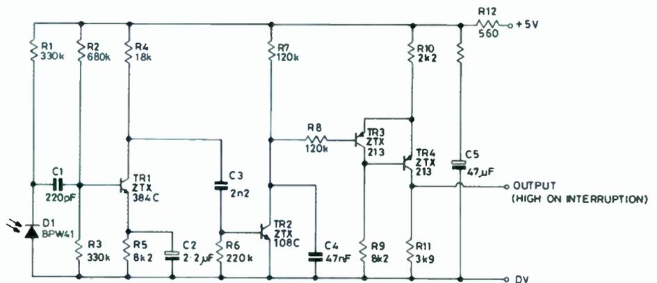
Fig. 6. A 70cm range infra-red system intended for parts counting.
