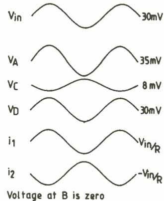
$Q_3$ ;  $Q_3$  has a voltage  $V_C$  input at its base and a voltage  $V_D$  driving its emitter through resistor  $R$ . Since  $V_B = 0$ , the current through  $R$  is given by:  $i_R = V_D / R = V_A \cdot g_m / (1 + g_m \cdot R)$ .
