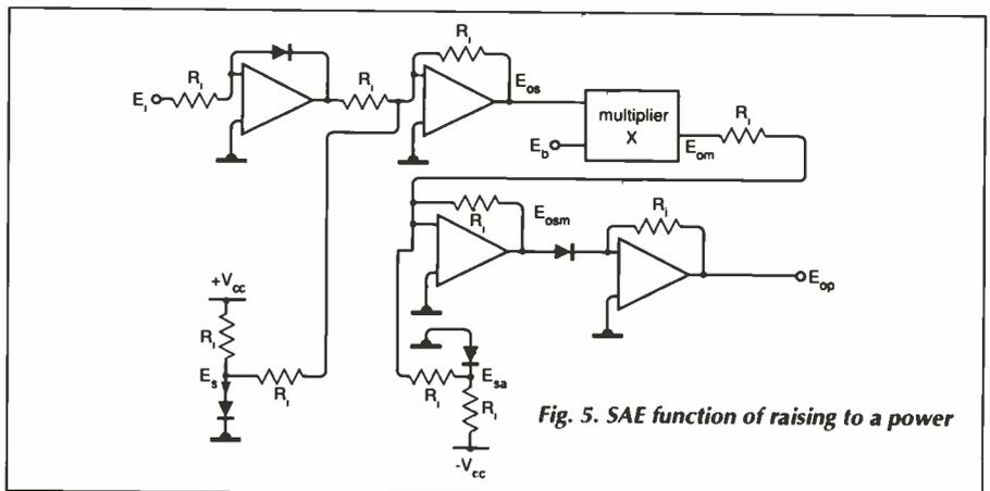
Fig. 5. SAE function of raising to a power
