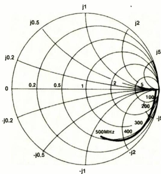
Fig.2. Input-impedance matching network, of which  $C_1$  forms a part, looks like 50ohms to the source (chart normalised to 50ohms)
