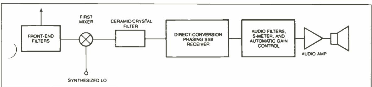
rejection greater than 70dB. Using the circuit shown in Fig. 6, you can reliably obtain rejection levels of 35dB. Add an inexpensive 2-pole crystal or ceramic filter, and you can meet the 70dB requirement. Fig. 7 shows a complete SSB receiver that uses the phasing filter technique. The block labelled "direct conversion phasing SSB
