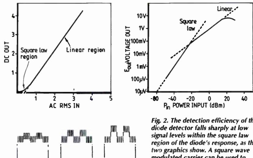
Fig. 2. The detection efficiency of the diode detector falls sharply at low signal levels within the square law region of the diode's response, as the two graphics show. A square wave modulated carrier can be used to determine sensitivity. See text.
