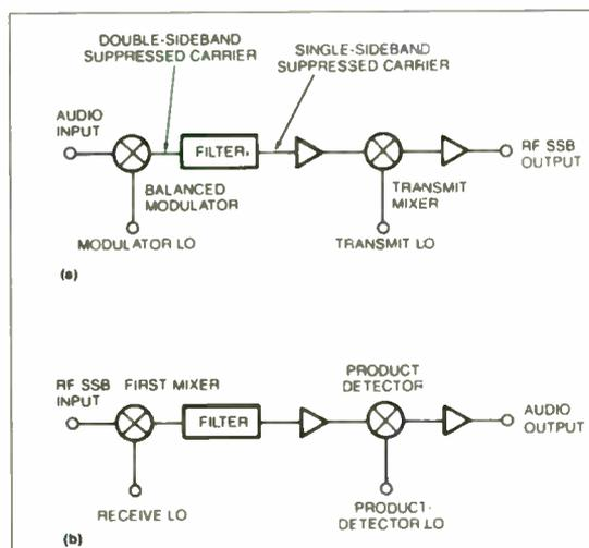
Fig. 1. In the traditional filter method, the generator (a) produces a double-sided signal, and the balanced modulator nulls the carrier. The detector (b) simply reverses the generation procedure to develop the audio output.
