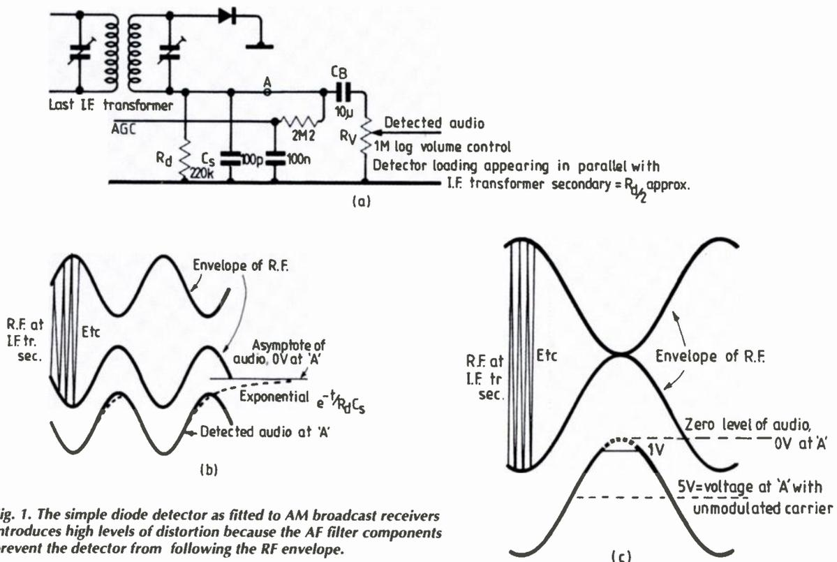
Fig. 1. The simple diode detector as fitted to AM broadcast receivers introduces high levels of distortion because the AF filter components prevent the detector from following the RF envelope.
