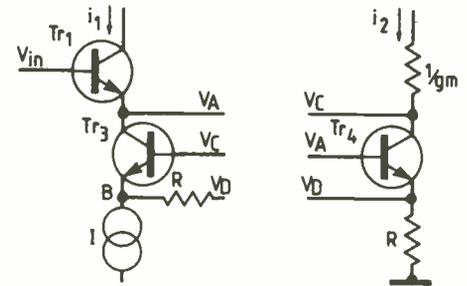
Fig. 1. The circuit is divided into two parts, to analyse the operation of the cascode  $Q_2, Q_4$ .
