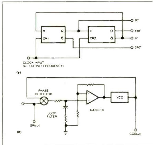
Fig. 4. You need quadrature dual mixers whether you are using the phasing or the Weaver method. The mixer in (a) maintains good phase integrity at clock rates ranging to several MHz. Clock and operating frequencies are equal in the mixer circuit (b), which gives an advantage over the flip-flop design.
