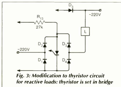
Fig. 3: Modification to thyristor circuit for reactive loads: thyristor is set in bridge
