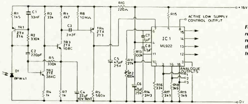
Fig. 7. A simple IR remote control receiver (left) and the associated transmitter (below).
