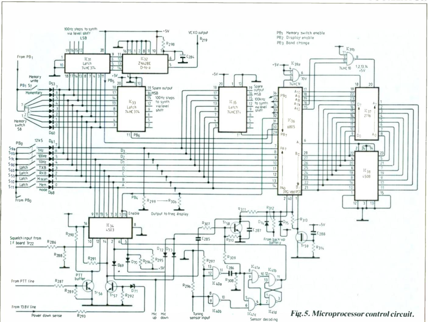
**Fig.5. Microprocessor control circuit.**
