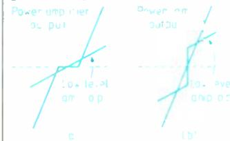
the switch and increase the input signal level to obtain the same output amplitude, and assume that the presence of the signal feedback removes all crossover distortion from the output. If this is to happen, the output from the low-level amplifier must look as in Fig. 2(b) with an infinitely fast step in the waveform, implying that this part of the circuit must have infinite bandwidth and slew-rate.
