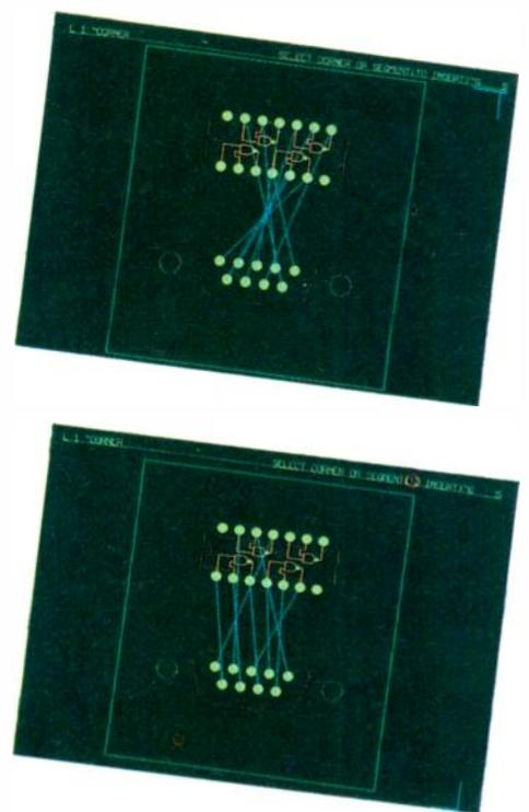
**Fig.5.** Optimising the layout by pin and gate swapping. The effect of swapping is shown below.
