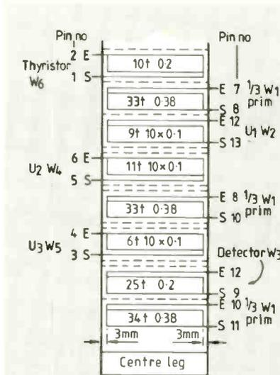
Fig. 2. Winding details of the transformer.
