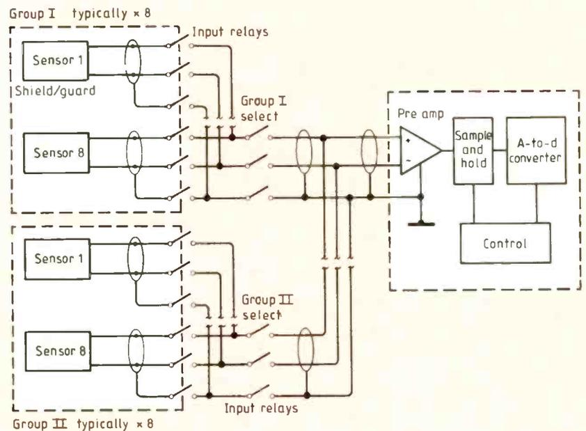
**Fig. 6.** Typical multiplexer system.
