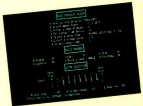
**Fig.3. User defaults screen used to select displayed layers and other screen defaults.**
