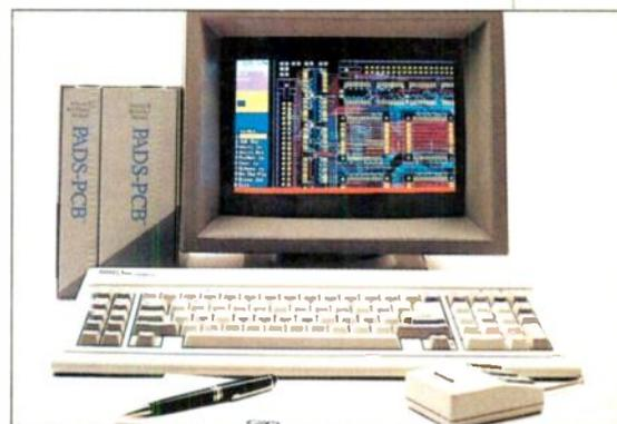
*Typical PC-based cad station with PCB design in progress, using PADS-PCB from Microtel which is to be described in a future issue.*
