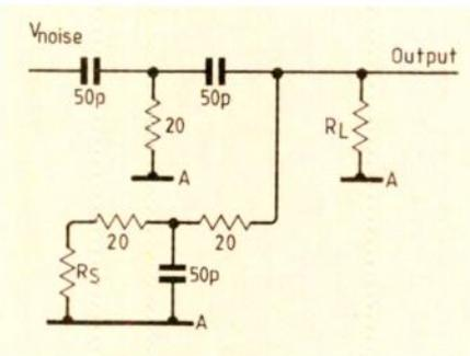
Fig. 10. Equivalent of T-switch circuit.
