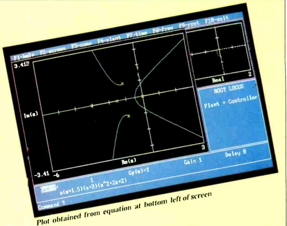
Plot obtained from equation at bottom left of screen
