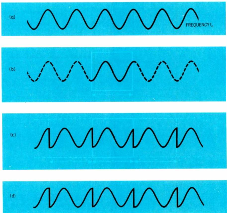
or should it? (Fig. 1). In general, major discontinuities exist at the window edges, are assumed to be part of the true signal and are therefore transformed into the frequency domain, leading to false results. What form will this distortion of the results take?
