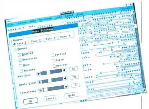
**Fig.3.** Strategy set-up window for an autorouter.
