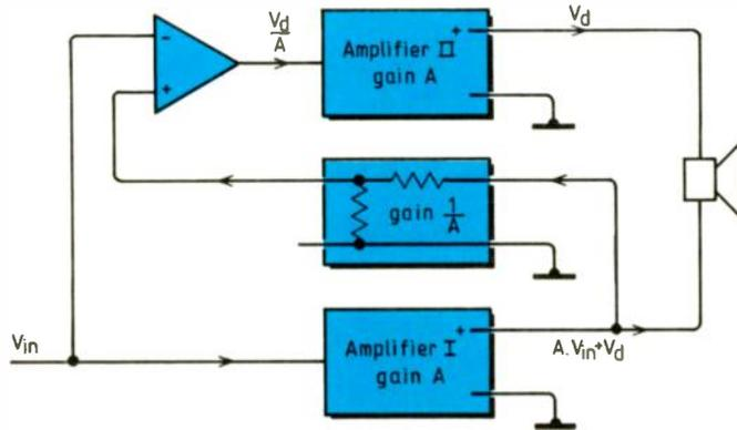
have to do is to connect the loudspeaker to the 'plus' (or 'hot') connectors of two amplifiers. The loudspeaker is then driven by the difference of the two power signals. Mr Brown's Fig. 3 can then be implemented as illustrated here.
