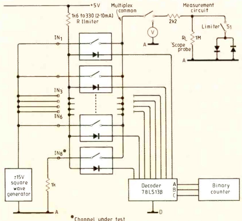
**Fig. 7.** Eight-channel multiplexer test circuit using photovoltaic relays.
