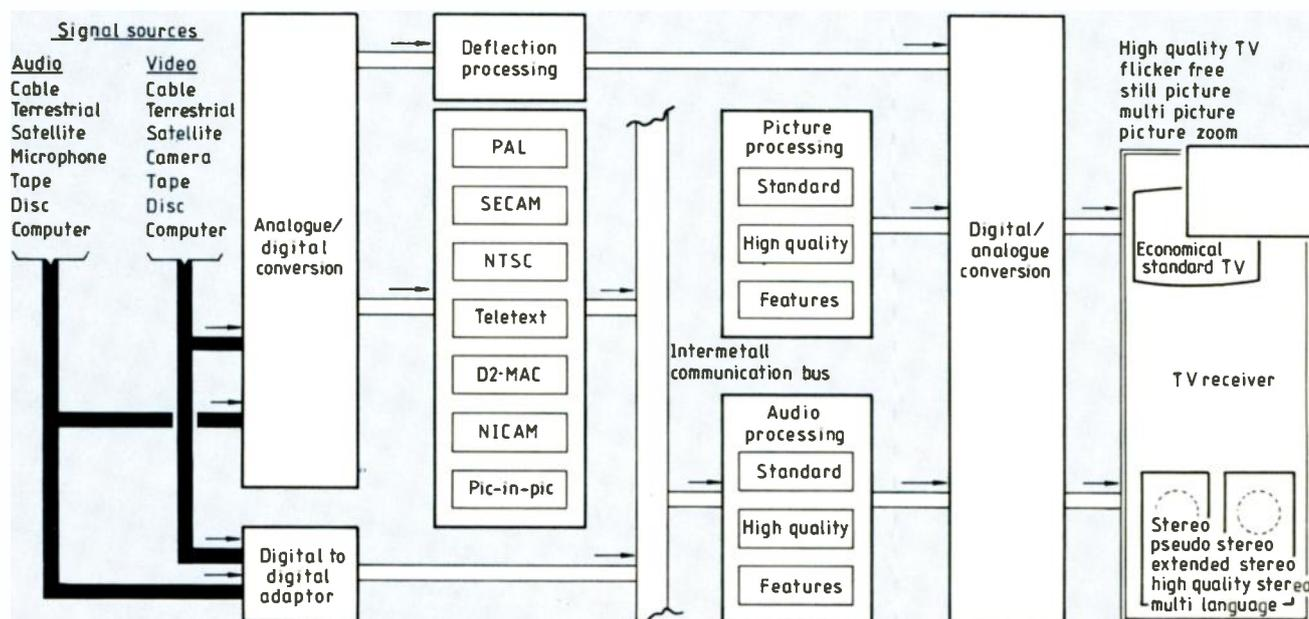
standards, the digital audio signal is contained in the baseband. It is separated and conditioned for further processing in the audio signal section.
