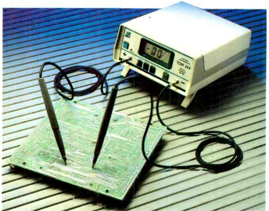
simple as it is novel, the measurement of DC potentials in the microvolt range has required some ingenuity on the part of the designer, David Mawdsley. The instrument requires twin contact electrode probes. An inner spring-loaded point measures potential while an outer fixed point provides the current injection. Successful measurement also re-
