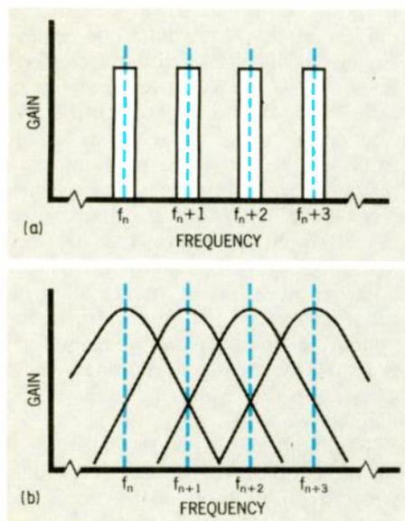
**Fig. 4. The idealized band-pass filter at (a) is, in practice, more like that shown in (b).**
