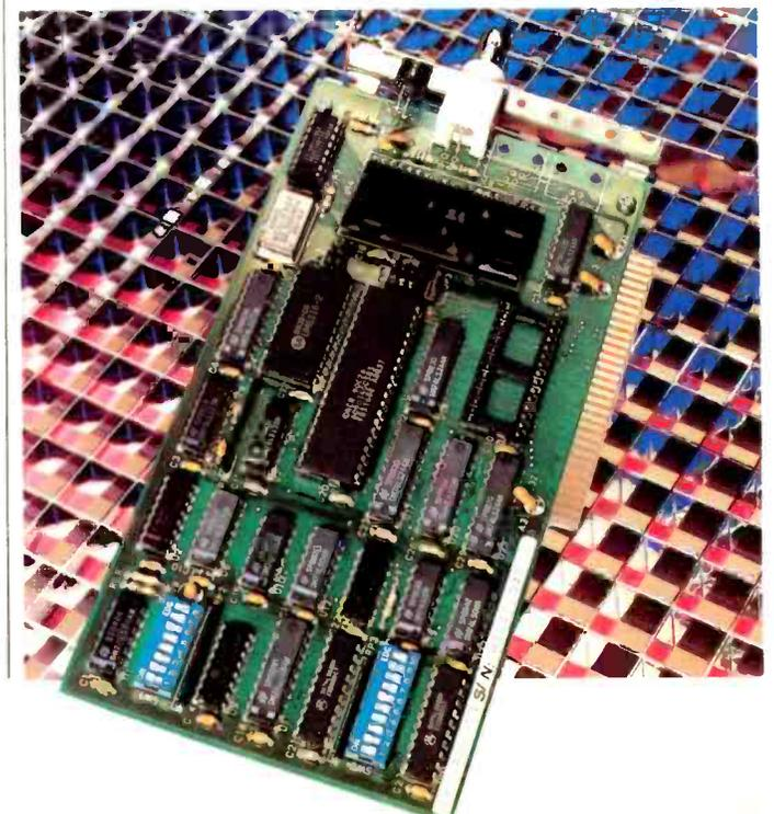
on an IBM PC or compatible system. The SO16SIMPC allows H16 programs to be developed, tested and debugged before any target hardware has been developed, allowing hardware and software design to progress in parallel. Hitachi Europe, 0923 246488
