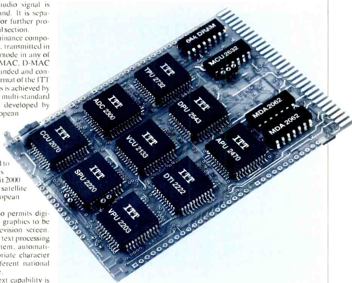
*This prototype board, measuring 8×10cm, accommodates the complete system for all standards; it includes text processing and other functions.*
