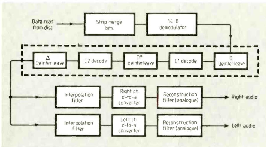
However, details of how the CD player data system works make up for the over-adventurous title. Cross-interleave Reed-Solomon coding, data framing and oversampling are all outlined in the article. There is also a run-down of advantages that accrue from using the ADSP210 family DSP chips and a note that there is an entire section on multi-rate digital filtering in the ADSP210x Family Applications Handbook, Volume Two.
