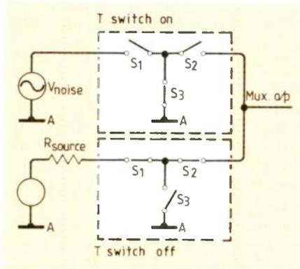
Fig. 9. Simplified arrangement of T-switch multiplexer.
