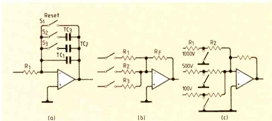
Fig. 12. Applications of photovoltaic relays: (a) integrator time constant and reset selector; (b) input selector; (c) high voltage selector.
