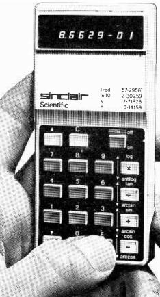
• 12 functions on simple keyboard Basic logs and trig functions (and their inverses), all from a keyboard as simple as a normal arithmetic calculator's. 'Upper and lower case' operation means basic arithmetic keys each have two extra functions
