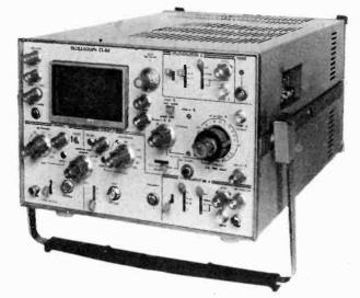
Power supplies: $115/230V \pm 10\%$ , 50–40 Hz.Dimensions: $300 \times 200 \times 420$  mm.Weight:19kg.PRICE, complete with full complement of connectors, cables, adaptors and accessories £470 exclusive of VAT.
