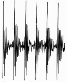
Fig. 1. A section of the first vowel sound in the word "hello" as seen on an oscilloscope
