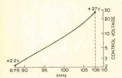
Fig.5. Voltage available from the tuning control unit as a function of frequency.
