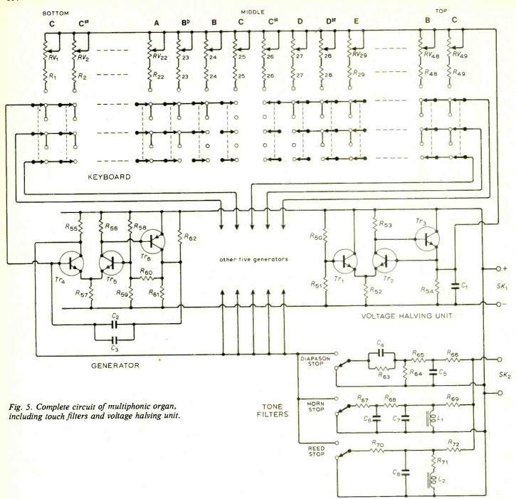
in which the normally open contact of one pole, the normally made contact of the next pole of the same switch and the changeover contact of same pole of the next switch is one piece of gold plated wire. This eliminates all wiring between poles of each switch and between switches.
