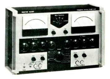
Each of these bridges has ten decade ranges and can be used to measure any type of component or complex impedance.
