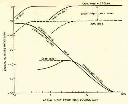
Fig. 7. Noise performance of the modified receiver compared with the original curves of the April 1971 article.
