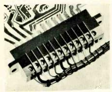
connector and a screw terminal block. The Edgeblock has a single row of 12 contact positions on 5.08mm pitch and is designed to accept p.c.b. thicknesses from 1.37mm to 1.88mm. The gold-plated phosphor bronze screw terminal contacts are rated at 5A and can accommodate wire sizes ranging from 7/0.22mm to 19/0.3mm. The dielectric moulding is grey self-extinguishing a.b.s. having a working temperature range of minus 20°C to plus 80°C. Pye Connectors Ltd, Hitchin Street, Biggleswade, Beds.
