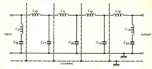
Fig. 3. Harmonic suppression filter to prevent television interference.
