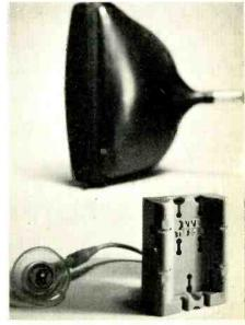
E.h.t. rectifiers and multipliers for solid-state colour television in silicon by General Instrument Europe (left) and in selenium by ITT.
