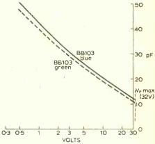
Fig.1. Capacitance versus voltage relationship for the variable-capacitance diode alternatives.
