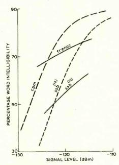
Fig. 4. Estimated threshold intelligibility performance of "Frena" compared to single sideband and carrier position modulation.
