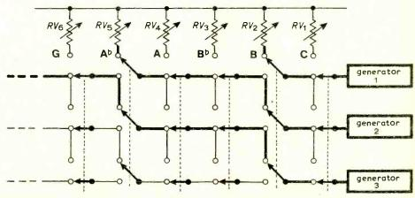
Fig. 4. Part of a multiphonic organ with two keys, Ab and B, pressed simultaneously. The connection paths between the variable resistors and the generators are shown by the thickened lines.
