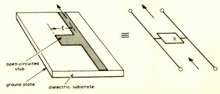
Fig. 1. Illustrating a T-junction in microstrip transmission line. Reactance X is a function of the stub length and can be made to vary between zero ohms and infinity.
