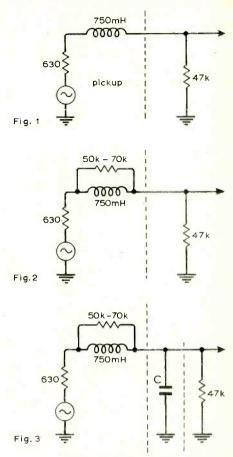
are normally tailored by the cartridge designer for an optimum load of  $47k\Omega$ . Please note, I have not taken into account at all the inevitable mechanical resonances in the pickup such as that which arises from the stylus mass and the compliance of the record material. These will almost certainly contribute to an additional rise in amplitude at the h.f. end of the passband.
