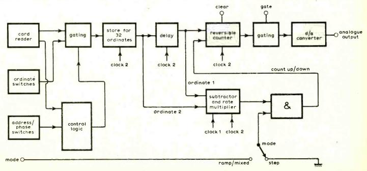
One way of generating waveforms digitally, proposed at Leicester Polytechnic, which can be used with an inexpensive pencilled-card reader.
