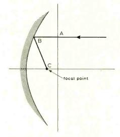
Fig. 1 The difficulty with a parabolic reflector arises because reflector size is comparable to wavelength at some frequencies.
