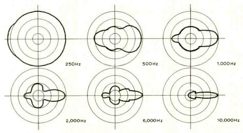
Fig. 9 Polar diagrams of M69 cardioid microphone in 24in diameter reflector of 7in focal length.
