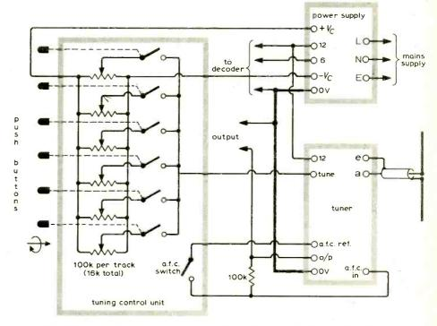
Fig.3. Method of connecting the switches of the tuner control unit to the tuner.
