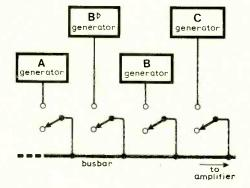
Fig. 2 (left). The polyphonic organ has a generator, individually tuned and switched, for each note.
