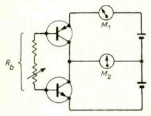
has the higher  $h_{\rm FE}$ . If the base-emitter drops can be allowed for  $R_b$  may be calibrated in base current: this is useful information when the matched pair is transferred to a working circuit.
