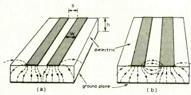
Fig. 2. Coupled microstrip lines showing the electric field distributions for the two analytical modes. Coupling is a function of the spacing and is much stronger for the odd-mode, making the characteristic impedance less than that of the even-mode case.
