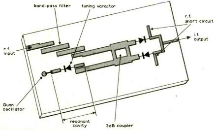
Fig. 6. Microstrip receiver with integrated local oscillator, approximately four times full size. Even when packaged, size and weight are many times smaller than waveguide circuitry.
