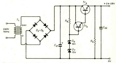
Fig. 4. Power supply circuit diagram.
