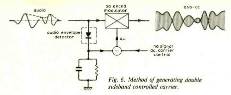
been proposed in which the carrier amplitude is made to vary inversely as the sideband amplitude<sup>16</sup>.
