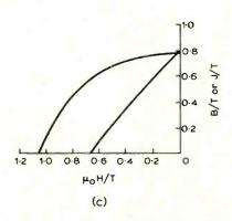
Fig. 1. (a) Demagnetization curve with B in tesla and M and  $Am^{-1}$  against H in  $Am^{-1}$ . (b) With B in tesla and J in tesla against H in  $Am^{-1}$ . (c) With B in tesla, J in tesla against  $\mu_oH$  in tesla. The left curve in each case is that of  $B - \mu_oH$ .
