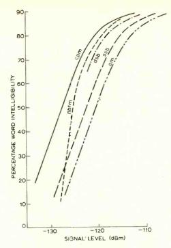
Fig. 3. Threshold intelligibility performance of amplitude modulation, single sideband, double sideband suppressed carrier, narrow band frequency modulation and carrier position modulation.
