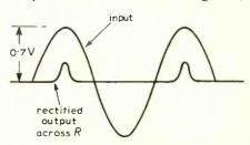
simple diode rectifier would give no measurable output with such a small amplitude input signal. In the circuit of Fig. 10.2 the diode  $D_1$  is connected in the feedback path of the amplifier so that the initial forward voltage drop required to make the diode conduct is supplied by the amplifier output voltage. Before diode conduction starts the amplifier acts virtually open loop so that the signal required at the input to cause diode conduction is very small,  $\frac{0.5}{A_{VOL}}$ V.
