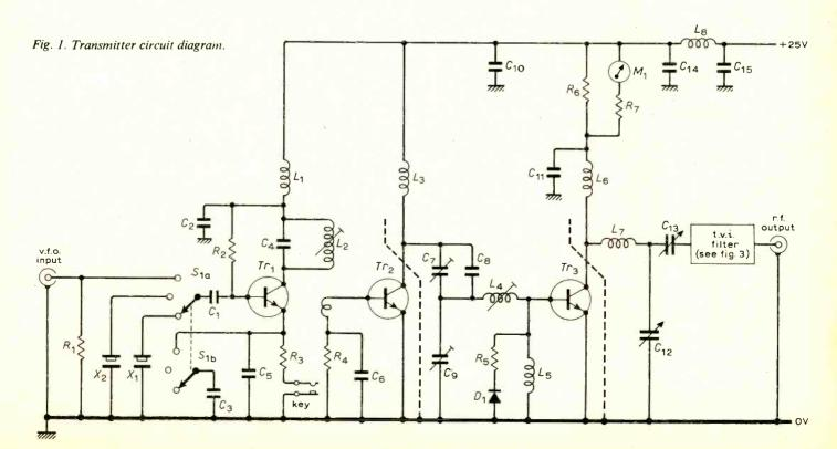
stage must be correctly matched to the load. The output impedance of this transistor is made up of a resistive component  $R_p$  in parallel with a capacitive component  $X_p$  representing the collector capacitance and circuit strays.
