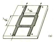
Fig. 5. Two examples of microstrip directional coupler, invariably used to produce an equal power split. There is always a 90° phase difference between the two outputs due to the different path lengths involved.
