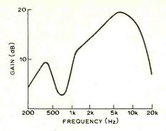
Fig. 2 Frequency response of omnidirectional DP6 microphone in 24in diameter reflector of 7in focal length.
