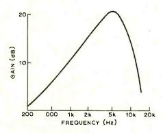
Fig. 5 Frequency response of M69 cardioid microphone in 24in diameter reflector of 7in focal length.
