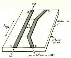
Fig. 4. Coupled-line microstrip directional coupler. An input at 1 produces a main-line output at 2 with a coupled output at 4. The output at 4 is a function of the spacing.
