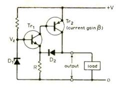
not affect the circuit other than to provide some temperature compensation for  $V_{be}$  changes in  $Tr_1$ . The maximum  $Tr_1$  collec-
