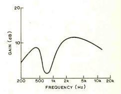
Fig. 6 Frequency response of DP6 microphone in 24in diameter reflector of 7in focal length with sound source 10° off axis.
