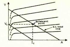
Fig. 5. Optimum load for maximum signal handling is represented by load line cutting axes at  $2V_C$ ,  $2I_C$ , for Fig. 3 (d) or (e) and depends on the quiescent condition and not transistor output resistance. In general optimum load can be calculated from peak voltage/peak current.
