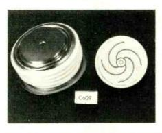
The C609 inverter thyristor from General Electric, rated at 1kHz and 1200A. The involuted cathode structure permits a rating of 850A at 5kHz, long-term di/dt of 500A/microsecond and minimum dv/dt of 400V/microsecond.
