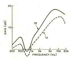
Fig. 3 Frequency response of DP6 microphone in 18 and 12in diameter reflectors of 7in focal length.
