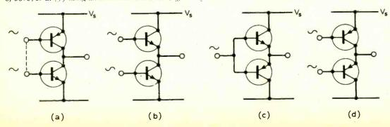
circuit quiescent current: at the point when the current in one transistor reaches zero the other has doubled. The peak load voltage remains at half the supply voltage when the output is biased to the supply mid-point for maximum undistorted output.
