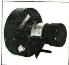
wide frequency coverage without spurious resonance. The multi-turn helical dial/drive mechanism is directly calibrated in GHz and gives high resolution throughout. The FMC 1 calibration accuracy is ±1MHz, and Type N connectors are fitted as standard. Flann Microwave Instruments Ltd, Dunmere Road, Bodmin, Cornwall.
