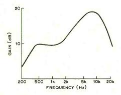
Fig. 4 Frequency response of DP6 microphone in 24in diameter reflector of 4in focal length.
