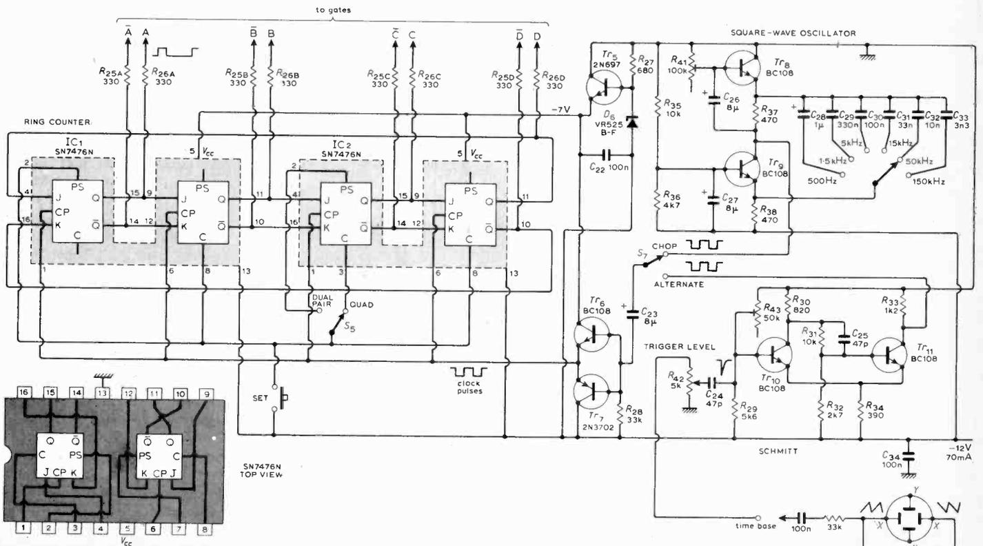
Fig. 8. Ring counter and clock pulse circuits.
