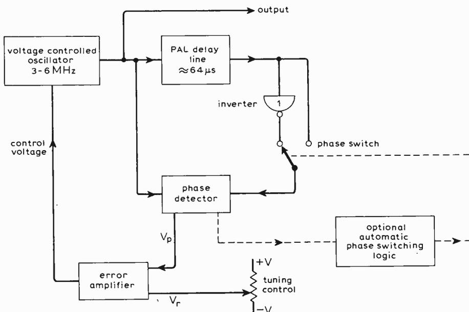
Fig. 1. Block diagram of the delay-stabilized oscillator.
