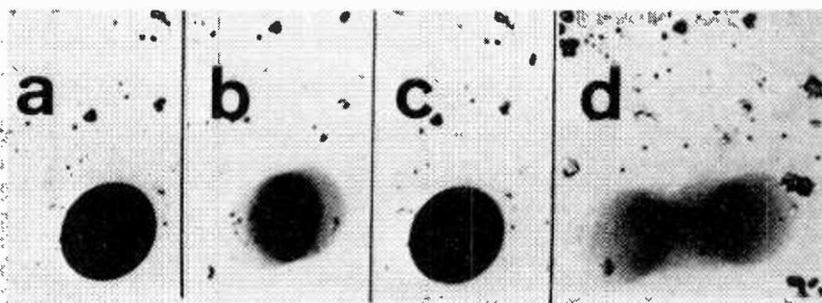
*Cylindrical magnetic domain (a) can be displaced by application of a gradient field — sinusoidally varying in this case — to give a lateral force, on the bubble (b). Sensitivity can be increased (d) by addition of an auxiliary field of higher frequency. Photographs are taken by shining polarized light through a thin slice of material and then through an analyser, the plane being rotated according to direction of magnetization (Faraday effect).*
