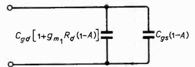
Fig. 18. Input equivalent circuit of Fig. 16.
