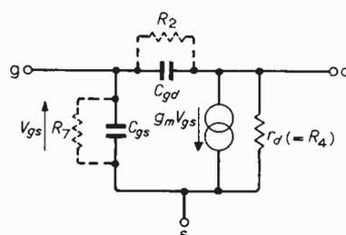
Fig. 4. The equivalent circuit for use at medium-frequencies.
