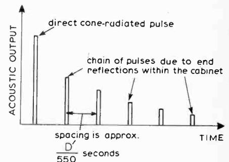
Fig. 3. Pulse-response (idealized) of cabinet shown in Fig. 2.
