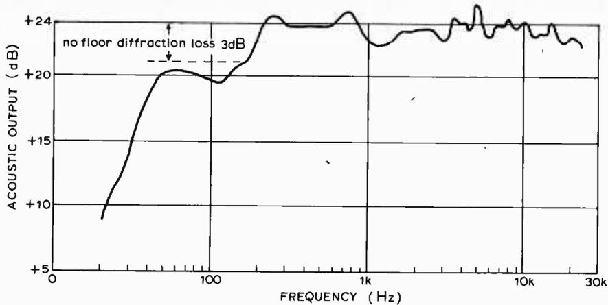
Fig. 8. Anechoic response curve of complete loudspeaker system.
