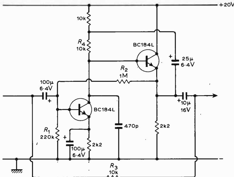
leads were used to the controls. Even a 470pF capacitor between input and output did not fully cure the hash pick-up, and so we hung a few hundred pF from  $Tr_1$  collector to earth, with good results.
