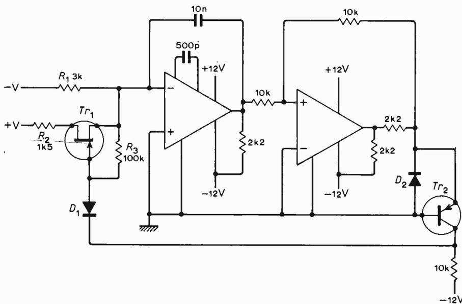
The circuit as it stands suffers from poor frequency stability against temperature due to the temperature coefficients of  $D_2$  and  $Tr_2$ , but this may be improved by increasing the amplitude of the square-wave using 3V zener diodes.
