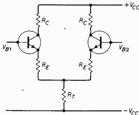
Fig. 3. Basic circuit of a push-pull stage.
