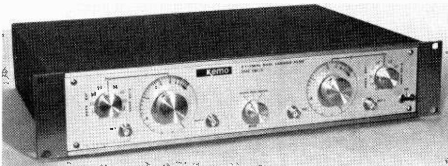
attenuation of 24dB/octave. The channels can be arranged in series or parallel by front-panel function-switch so forming a single band-pass or band-reject filter or low-pass or high-pass unit having 48dB/octave slope. The VBF/3 is one of a wide range of variable filters ranging in price from £130 to £1,500. Kemo (Consultants) Ltd, 42 Chancery Lane, Beckenham, Kent.
