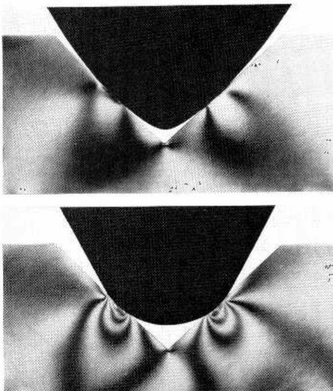
*New Shibata stylus (top) developed by JVC claims to reduce record wear by reducing pressure to one-quarter of that with an elliptical stylus (bottom) and to improve phase and amplitude response. Stress patterns shown are for equal downward force.*
