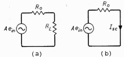
Fig. 17. Output equivalent circuits; (a) with load and (b) short circuit conditions.
