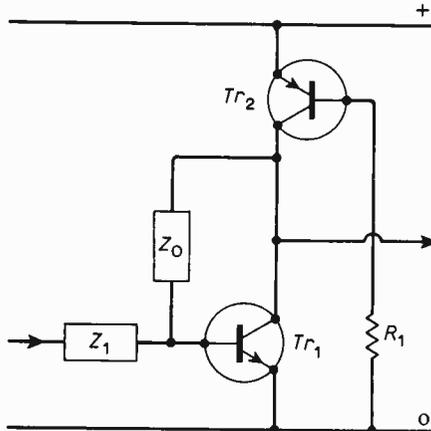
at the same d.c. level. For such circumstances the circuit shown gives a high voltage gain and low drift. Current gain can be added by means of emitter followers.
