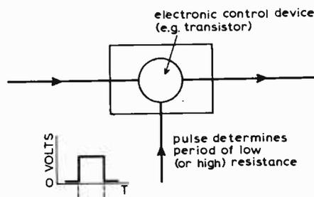
Fig. 2. Practical gate is an electronic device of which the resistance can be electrically controlled.
