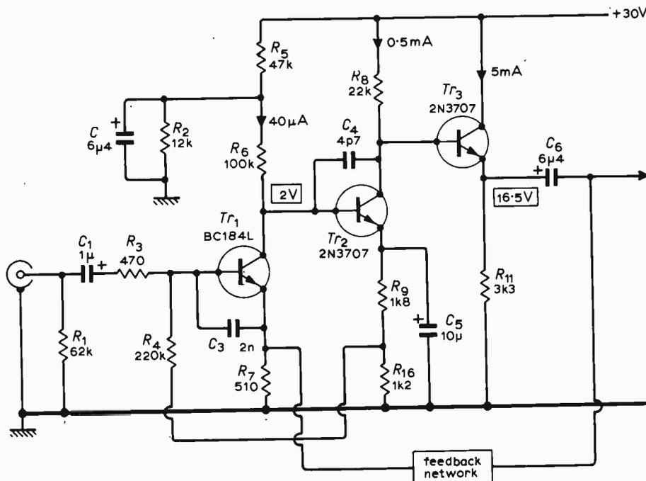
Fig. 8. Circuit of pre-amplifier for a magnetic pickup used to illustrate low-noise design procedure.
