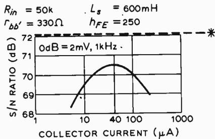
Fig. 7. Calculated signal-to-noise ratio of an equalized amplifier as plotted against  $I_C$  of first stage. \*Broken line represents theoretical maximum with noiseless transistor. (Graph neglects excess noise.)
