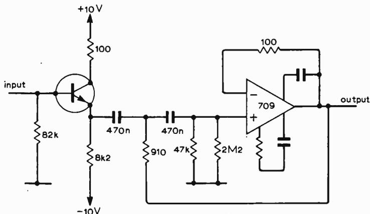
Fig. 3. Filter section to be added.
