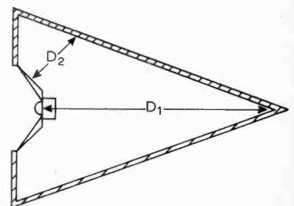
Fig. 4. Triangular cabinet showing different reflecting path lengths.
