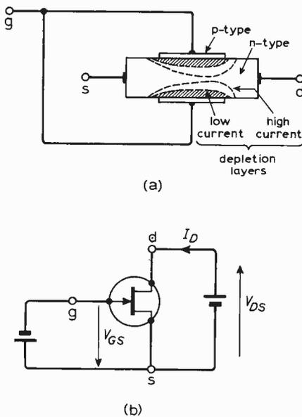
Fig. 1. (a) A bar of *n*-type silicon sandwiched between two *p*-type layers together form an *n*-channel f.e.t. (b) The polarity of power supply and bias voltages when using an *n*-channel device.
