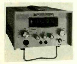
LO" switch simplifies operation in production line testing, and an analogue output, scaled zero to  $\pm 6V$  at 1mA, can be used to drive an alarm monitor or recorder. A fourth digit 100% overrange virtually doubles the measurement capability. U.K. agents: General Test Instruments Ltd., Gloucester Trading Estate, Hucclecote, Gloucestershire GL3 4AA.
