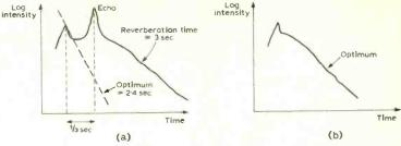
Fig. 3. Reproduction of transient sound at 500Hz in the Royal Albert Hall (a) before treatment and (b) after treatment.
