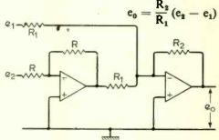
Features. Subtraction is accomplished by a process of inversion and summation. Both amplifiers are used in the inverting configuration and common-mode voltages are effectively eliminated.
