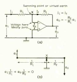
Fig. 1. (a) Inverting amplifier employing "operational feedback". (b) A voltage "lever" analogy of the inverter connection. Point X corresponds to the fulcrum, and the summation of currents at X is analogous to the summation of moments about the point of balance.
