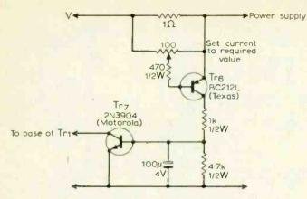
Fig. 10. Amplifier current regulation circuit.
