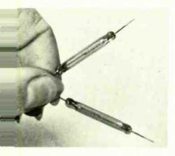
ild them closed. Closure time is 1ms and release ne 50 $\mu$ s. Current of 100mA can be switched it 1A can be carried by the closed contacts. Inlation resistance between the reeds exceeds )<sup>5</sup>M  $\Omega$  and minimum breakdown voltage is 1000V. esonant frequency is approximately 1650Hz. mbient operating temperature range extends om  $-55^{\circ}$  to  $+100^{\circ}$ C. Mullard Ltd., Mullard ouse, Torrington Place, London W.C.1. **'W 322 for further details**
