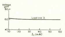
Fig. 4. Voltage gain versus collector current, common-base.
