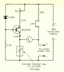
Fig. 3. Test circuit for diode and zener diode temperature coefficients.
