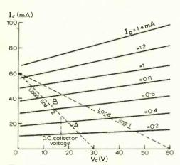
Fig. 1. Output characteristics of a commonemitter stage.
