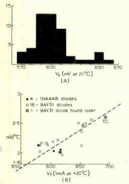
Fig. 2(a). Spread of forward voltage obtained from a random selection of 50 diodes type BAY31 when operated at a current of 1mA.
