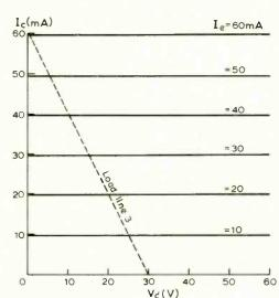
Fig. 3. Output characteristics, common-base.
