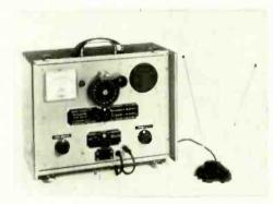
is heard the instrument locks on to the signal which, say the makers, enables the operator to determine if the signal is from a legitimate local transmitter or from a clandestine unit. Having established that the room contains hidden illegal equipment, a probe enables the offending equipment to be located. Leonard Wadsworth & Co. Ltd., Broadway House, Broadway, London S.W.19. WW 326 for further details
