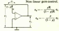
Features. A wide-range variable-gain amplifier; range from zero to very high values. Gain is not linear with respect to potentiometer rotation and the input impedance drops as the gain is increased.
