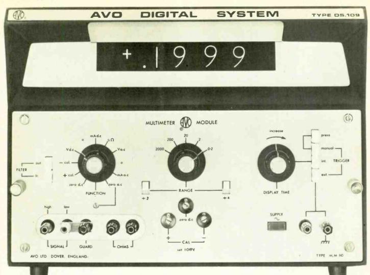
With the Multimeter module and an optional a.c. converter, the new Avo Digital System measures not only a.c. and d.c. voltages but also a.c:/d.c. current and resistance.
