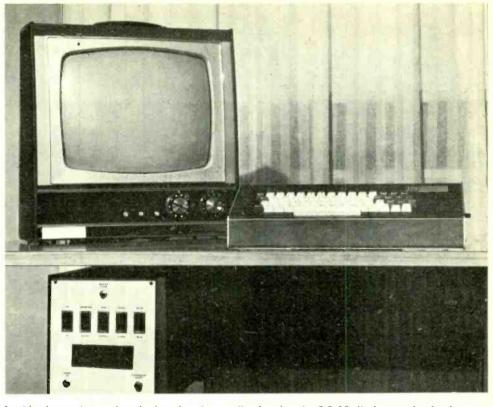
In this picture the monitor, keyboard and controller forming the CC-30 display can be clearly seen.
