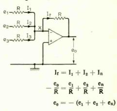
Features. A separate input resistor is used for each input signal to be summed. Any number of inputs may be used; the output gives the inverted sum of all inputs. The summing point X being a virtual earth, the inputs are effectively isolated from one another. If the individual input resistors are given values different from that of the feedback resistor the output is the sum of a series of terms each proportional to one of the input signals but each multiplied by some arbitrary coefficient, i.e.
