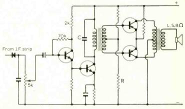
Fig. 1. Circuit diagram of the original amplifier and output stages
