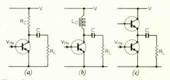
Fig. 1. Basic class A circuits using (a) load resistor  $R_c$  giving power conversion efficiency of about 12%, (b) l.f. choke giving better efficiency but being bulky and expensive, and (c) a second transistor as collector load.
