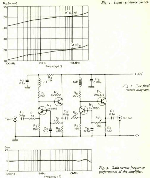
emitter-follower connection and a 2N3866 was chosen to provide a common-base input amplifier. The most suitable operating point of the output stage was computed in a manner similar to that indicated in the graphs of Figs 1 and 2 with the result that a quiescent emitter current in the order of 120 mA was established for the 2N3375 at a supply voltage of 30 V.
