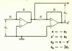
Features. A combination of two unity gain inverters arranged to give a balanced output. Used for driving balanced loads or push-pull stages when earth reference is critical. The peak-to-peak output swing is double that of a single amplifier.
