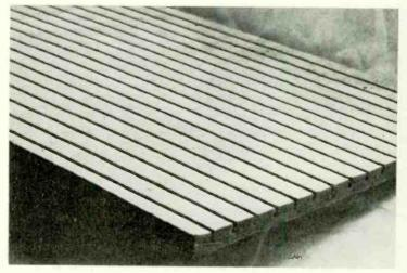
(d) Halltex acoustic fibreboard. Decorative panelling widely used on walls and ceilings.
