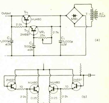
Fig.9. (a) Power supply unit, and (b) parallel connected transistors for high currents.
