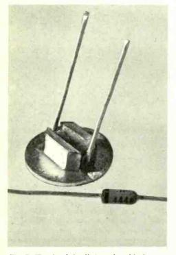
Fig. 7. The tip of the diode probe with the diode fixed in position.
