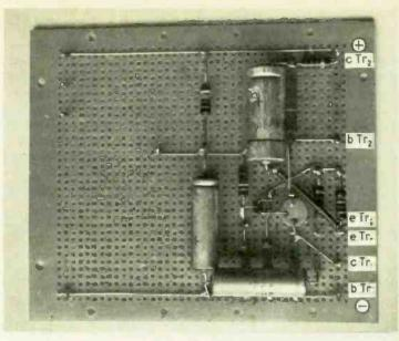
Layout of single channel of 10 + 10 watt amplifier on standard  $4in \times 4\frac{3}{4}in$  'Lektrokit' s.r.b.p. pin board.
