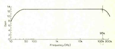
Fig.4. Gain/frequency response curve of amplifier.
