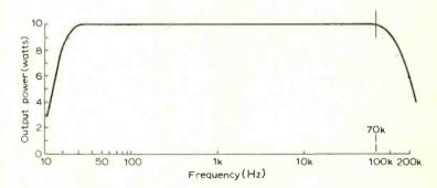
Fig.5. Output power/frequency response curve of amplifier.
