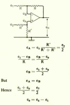
Features. The amplifier acts as a unity-gain differential-input single-ended output amplifier. A variation of this circuit is the subtractor with gain shown below.
