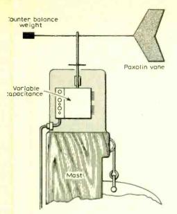
Fig. 3 Some details of the wind-vane and capacitor unit
