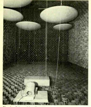
Fig. 4. Polyester/glass-fibre diffusers as used in the Royal Albert Hall undergoing tests in an anechoic chamber.
