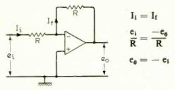
Features. Input impedance equals  $R_i$ , output impedance small, usually less than 1 ohm. Used wherever sign changes are necessary or to lower the impedance level of a signal.
