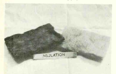
(a) Glass-fibre. Available in 20-ft rolls of various widths, lin & 2in thick. Used in loudspeaker enclosures, and in roof insulation.
