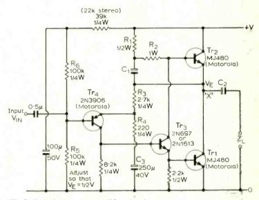
Fig. 3. Practical power amplifier circuit.
