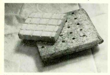
(c) Expanded polystyrene. Small tiles or large 8ft × 4ft sheets up to 3in thick available. Perforated sample is Jablite, in 1, 2, or 3ft squares or large sheets. materials which can be used to control reverberant sound energy is required. A sound-absorbent material is one whichcan dissipate as frictional (heat) losses, some part of the sound energy incident on or penetrating its surface.
