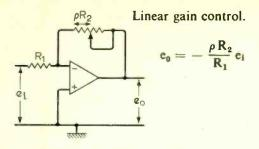
**Features.** A narrower range of gain settings than in previous circuit, 0 to  $R_2/R_1$ , but gain is linear with respect to potentiometer rotation. Input impedance equals  $R_1$ .
