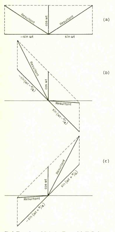
Fig. 3. The resultants of the local oscillator and the idealized swinging burst are shown at (a) and what actually happens in two successive lines at (b) and (c). The two resultants in each diagram represent the inputs to the two diodes of the phase discriminator.
