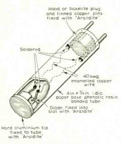
Fig. 8. Internal construction of the diode probe.
