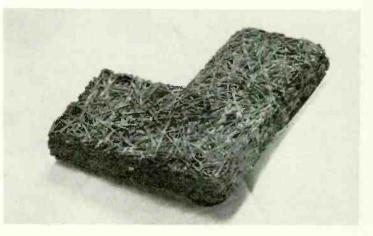
(e) Gypklith. Building slabs of wood/wool material. Provides both thermal and sound insulation. In many sizes and thicknesses. Density 28lb per cubic foot.
