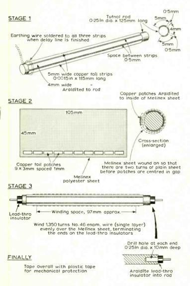
Fig. 1. Constructional details of the 0.6-µsec delay line are given here.
