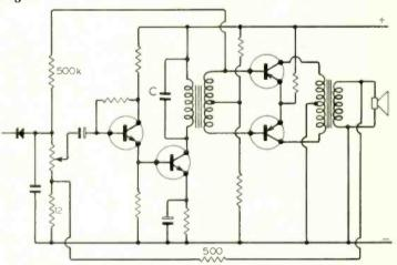
Fig. 2. Amplifier and output stages modified by the addition of positive and negative feedback. The  $500k \Omega$  resistor is connected by trial and error method to the end of the driver transformer winding which gives a slight increase in sound output
