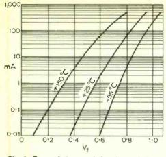
Fig. 1. Forward characteristics of a typical high-conductance diode
