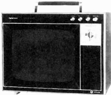
**Teleton model 12-T 203U** portable TV receiver with 31cm c.r.t. Power source 220/240V a.c. or 12V d.c. All v.h.f. and u.h.f. channels covered, 300-Ω balanced input. Eighteen transistors and four diodes employed. Weight 7kg. Price: about £79.
