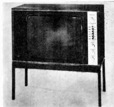
*Bush model CTV174D colour TV receiver using 56cm tube with 4:3 aspect ratio. Also features integrated circuit colour decoder and R,G,B drive to c.r.t. Price: 299gn. The Murphy CV2210D is similar.*
