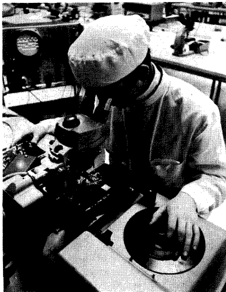
Testing completed integrated circuits with probes.
