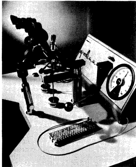
Bonding machine used for making connections to the mounted semiconductor chips.
