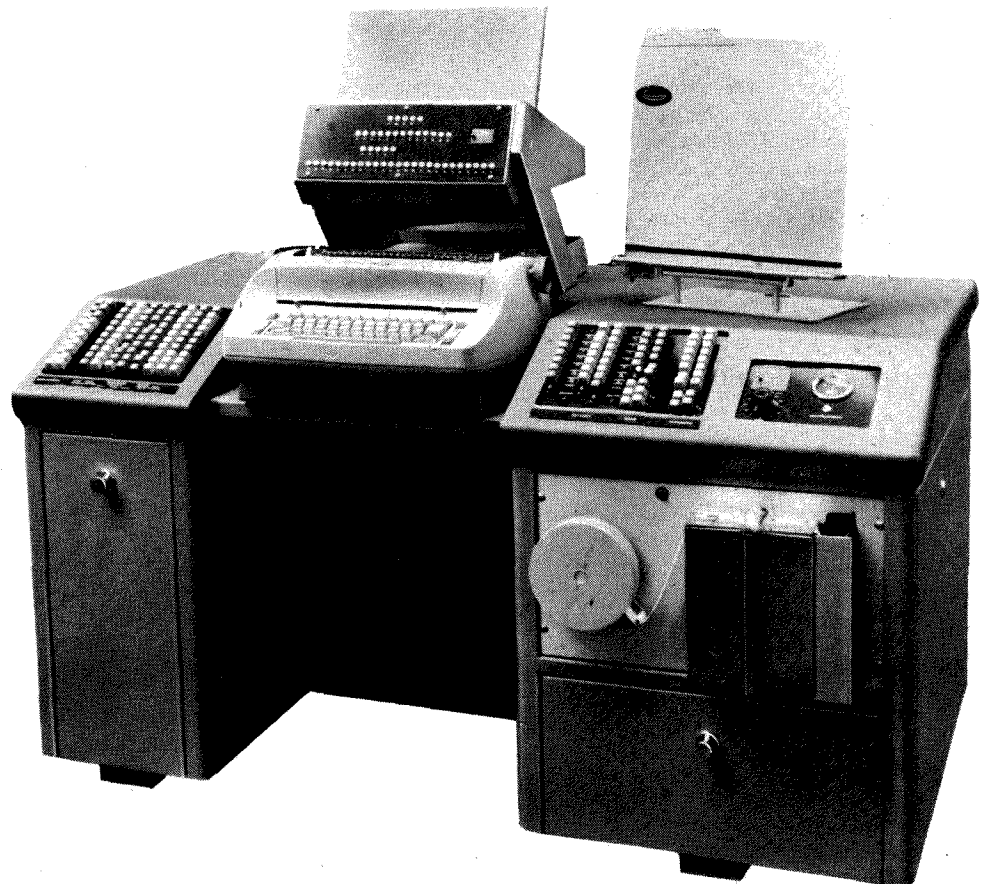
The Lumitype 540 keyboard. In the 540 system this keyboard carries out the part of the justifying cycle which involves calculating the deficit in the line and counting the inter-word spaces. The banks of keys to right and left of the typewriter allow the operator to select typeface, size, inter-line spacing and line length.
