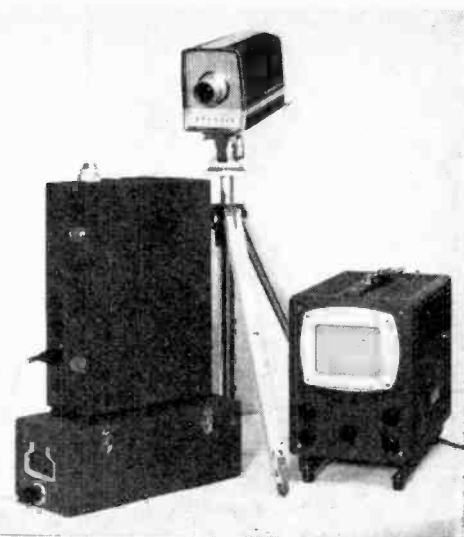
The inexpensive Grundig television camera, mentioned last autumn in our report of the Frankfurt radio show, can now be obtained with a portable battery-operated radio link, working on 440-460 Mc/s. The range is stated to be 2km average.
