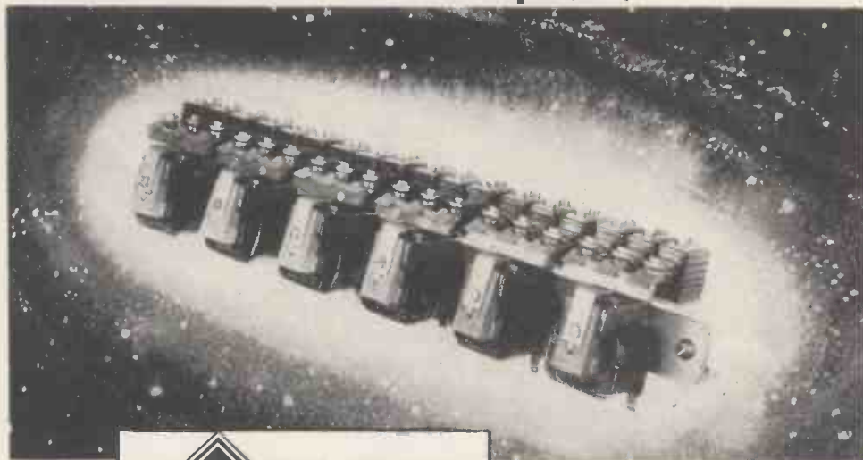
This rack of relays shown left occupies a length of only 9 inches
