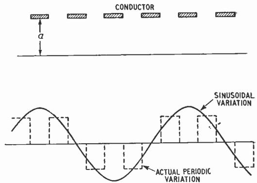
Fig. 4. R.F. fields in a periodic circuit.
