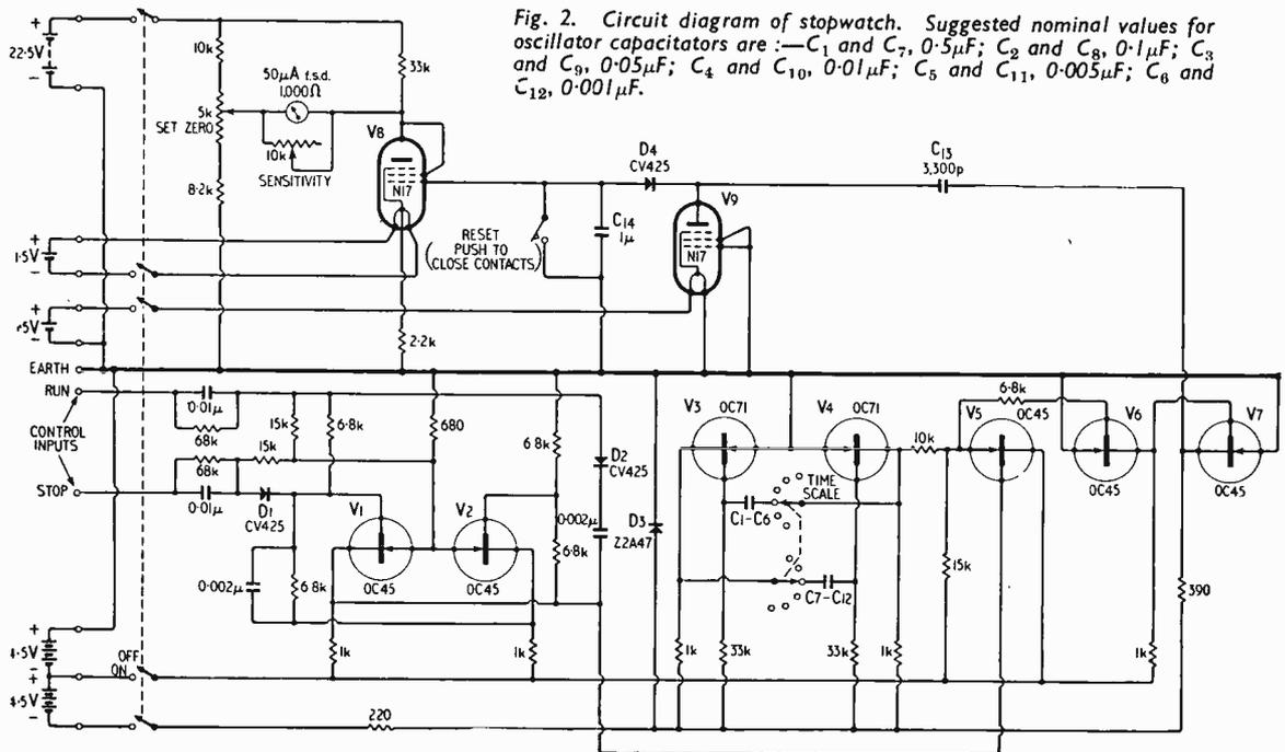
Fig. 2. Circuit diagram of stopwatch. Suggested nominal values for oscillator capacitors are:—C<sub>1</sub> and C<sub>7</sub>, 0.5μF; C<sub>2</sub> and C<sub>8</sub>, 0.1μF; C<sub>3</sub> and C<sub>9</sub>, 0.05μF; C<sub>4</sub> and C<sub>10</sub>, 0.01μF; C<sub>5</sub> and C<sub>11</sub>, 0.005μF; C<sub>6</sub> and C<sub>12</sub>, 0.001μF.
