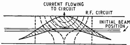
Fig. 14. Displacement of beam in crossed-field interaction.
