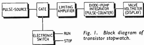
Fig. 1. Block diagram of transistor stopwatch.
