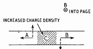
be forces as shown by the full arrows acting on the electrons at A and B, and this will result as previously in motion as shown by the dotted arrows, giving the situation shown in Fig. 17.
