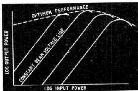
Fig. 3. Gain characteristics of helix type tubes.
