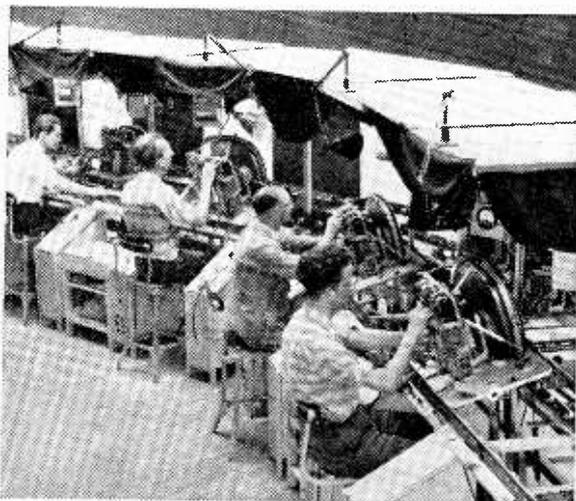
*TAILOR-MADE gravity conveyors constructed from Dexion slotted angle and "Glidewheel's" are being used on the television receiver assembly line at the Southend-on-Sea factory of E. K. Cole Ltd.*
