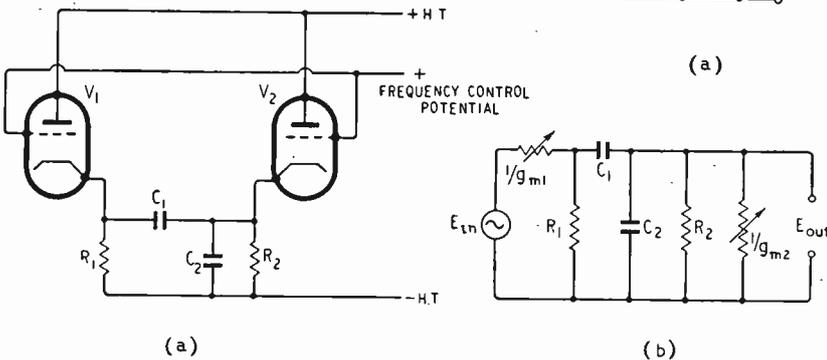
Left: Fig. 2. (a) Practical arrangement for achieving voltage-controlled variation of  $R_1$  and  $R_2$ . (b) Equivalent circuit, showing where the input voltage can be injected.  $R_k$  should be much larger than  $1/g_m$ .
