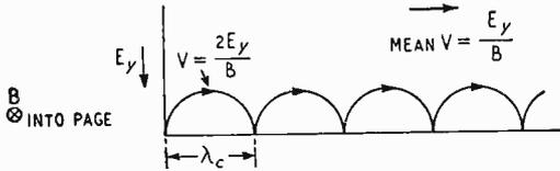
Fig. 10. Electron motion in crossed fields.
