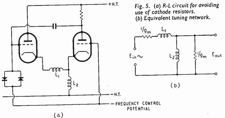
Fig. 5. (a) R-L circuit for avoiding use of cathode resistors. (b) Equivalent tuning network.
