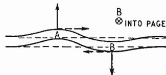
Fig. 17. Effect of r.f. disturbance on a sheet beam in crossed fields.
