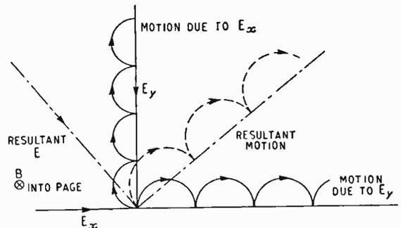
Fig. 11. Electron motion in combined crossed fields.
