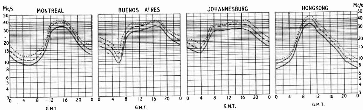
THE full-line curves indicate the highest frequencies likely to be usable at any time of the day or night for reliable communications over four long-distance paths from this country during November.
