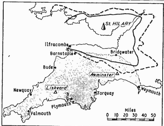
ESTIMATED SERVICE AREA of the two I.T.A. stations which will serve the south-west of England is shown (shaded) in relation to the primary and secondary service areas of the St. Hilary station. The two stations, one near Axminster and the other near Liskeard, will be operated jointly by one programme contractor. They are planned to be in service early in 1961.
