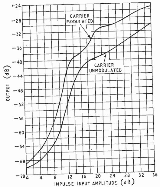
Fig. 14. Input/output characteristic for impulsive interference. Input carrier level 500  $\mu$ V, impulse p.r.f. 2,500/sec; relative output is referred to output with  $\pm 35$ kc/s deviation at 2kc/s and impulse input amplitude is referred to 1  $\mu$ V peak per kc/s bandwidth.
