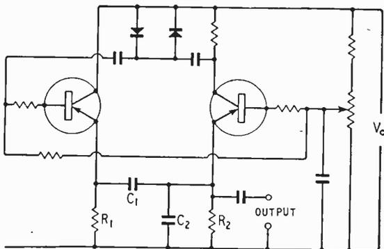
Fig. 6. Transistor-oscillator circuit (equivalent to Fig. 3).
