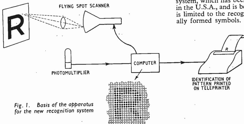
Fig. 1. Basis of the apparatus for the new recognition system
