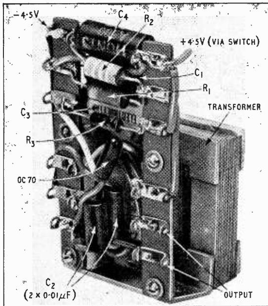
Fig. 4. A convenient form of construction for the transistor oscillator. Components can be identified from Fig. 3.
