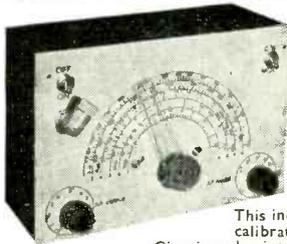
**KIT OF PARTS FOR SIGNAL GENERATOR.** Coverage 110 Kc/s.-320 Kc/s., 320 Kc/s.-900 Kc/s., 900 Kc/s.-2.75 Mc/s., 2.75 Mc/s.-8.5 Mc/s., 8.5 Mc/s.-20 Mc/s. Metal case 10in. x 6 1/2 in. x 4 1/2 in., size of scale 6 1/2 in. x 3 1/2 in. 2 valves and 1 rectifier valve, A.C. mains 230/250. Internal modulation 400 c.p.s. to a depth 30 per cent. Frequency calibration accuracy plus or minus 1 per cent. Modulated or unmodulated R.F. output continuously variable 100 millivolts, £3/10/-, P. & P. 4/-.
