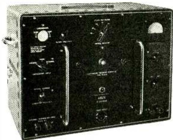
The Aren Sub-standard Frequency Generator is a portable instrument of rugged construction, designed for either laboratory or field operation. It may be used for checking and calibrating all types of Frequency Meters, Frequency-Indicating-Alarm Systems or as a Time Standard, etc.
