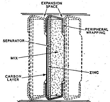
Inter-cell leakage is prevented and expansion permitted by the flexible wrapping of the latest flat-type dry cell.
