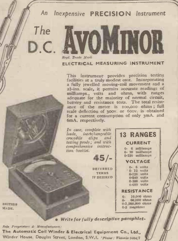
This instrument provides precision testing facilities at a truly modest cost. Incorporating a fully jewelled moving-coil movement and a 2 1/2-ins. scale, it permits accurate readings of milliamps., volts and ohms, with ranges adequate for the majority of normal circuit, battery and resistance tests. The total resistance of the meter is 100,000 ohms; full scale deflection of 300v. or 600v. is obtained for a current consumption of only 3mA. and 6mA. respectively.
