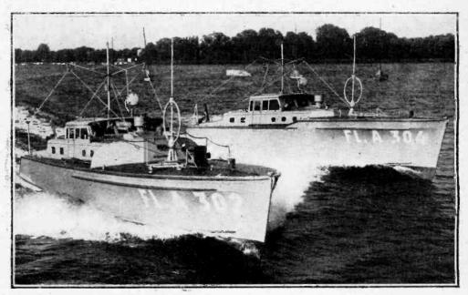
SEAPLANE TENDERS of the German Air Force have recently been fitted with mediumand short-wave transmitters (500-1000 and 50-100 metres) and direction-finding gear for use in locating aircraft in distress at sea. In the above photograph can be seen the DF loop and the transmitting and receiving aerials.
