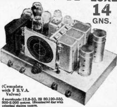
Controls.—A feature of the receiver is the number of independent controls fitted, making it extremely interesting to operate. These include sensitivity control (varying bias on R/F stage), or Q.A.V.C. with manual muting control for inter-station noise suppression. 5 position wave-change and gramophone switch. Progressive variable tone control operative on radio and gram.
