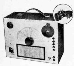
Wearite AC mains operated all-wave test oscillator. Note spare coils shown in inset.
