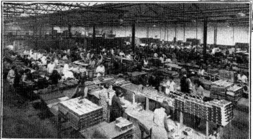
of this class of battery in the G.E.C. works. Next, the cells are assembled in cardboard boxes divided into the requisite number of compartments and the cells are interconnected to form a complete battery. ther voltage tests are made, and, finally, a bitumastic compound is poured over the top to seal the battery. It is then labelled, wrapped and packed ready for despatch.
