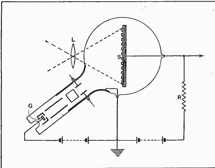
Photo-sensitive screen mounted in a CR tube for use in television transmitters.
