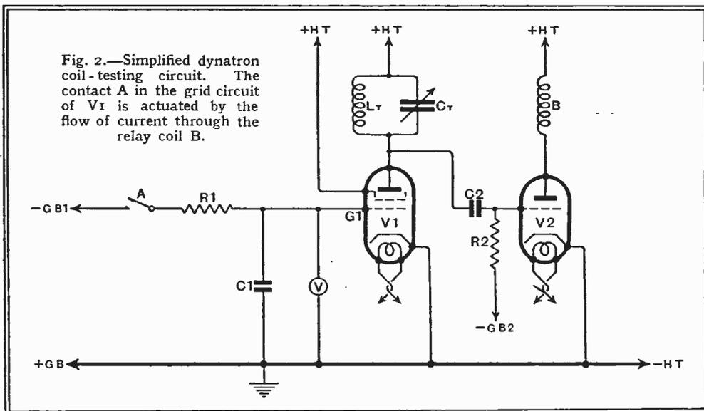
Fig. 2.—Simplified dynatron coil-testing circuit. The contact A in the grid circuit of V1 is actuated by the flow of current through the relay coil B.
