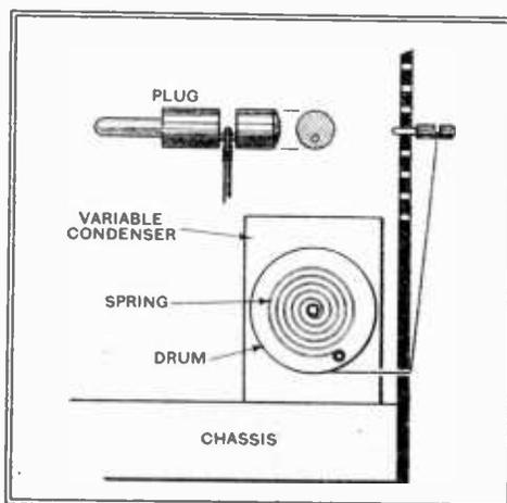
Operation of the Gody tuning system. Note the cord round the condenser drum, which is rotated against the tension of a return spring.
