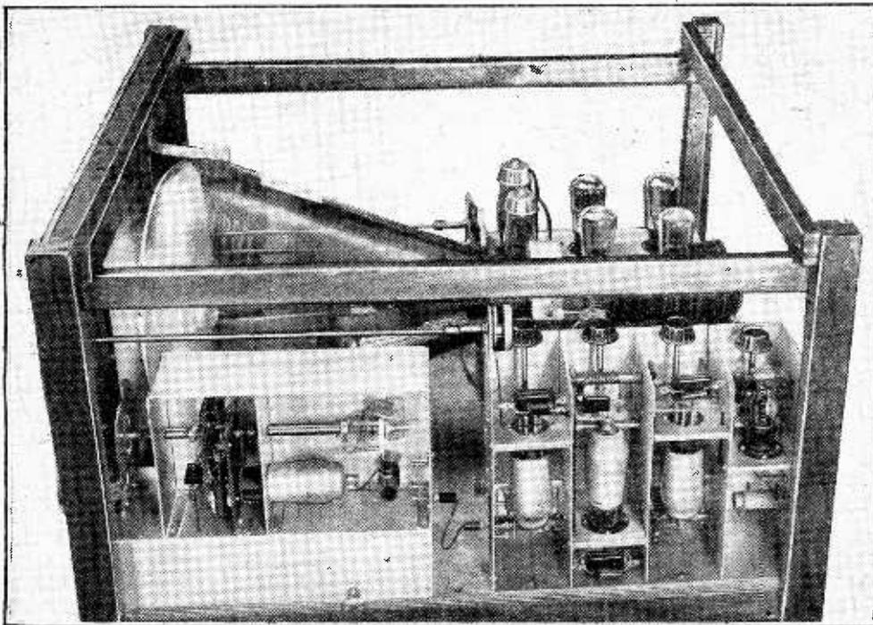
In this view of the upper deck of the complete television equipment the vision receiver can be seen on the right, with the sound receiver on the left. The time-base is on the far side at the back of the CR tube.
