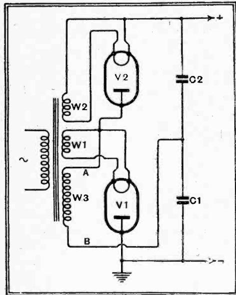
Fig. 35.—For a given output voltage, the lowest voltages between windings are obtained with the voltage-doubler circuit shown here.
