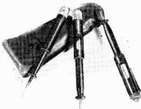
Forbat Pressler neon test prods.
