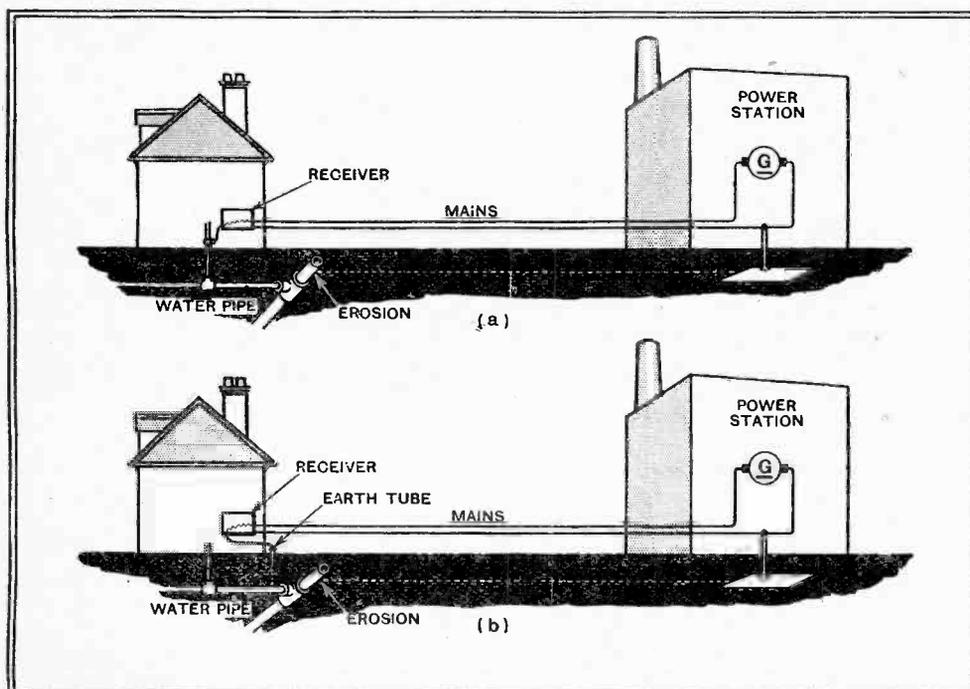
Diagrammatic sketch showing (a) how erosion of a water-pipe may be produced by a receiver in which there is a serious leakage to earth. But the substitution of a direct earth (b) would not necessarily prevent, or even greatly reduce, the erosion of the pipe.
