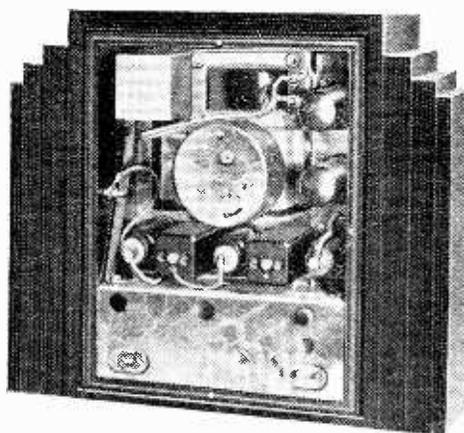
Back view of Radiochron showing all-metal valves grouped round central synchronous clock movement. The hands are driven through the hollow pole-piece of the moving-coil loud speaker.
