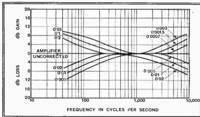
Fig. 4.—Characteristics of the tone-control system shown in Fig. 3.
