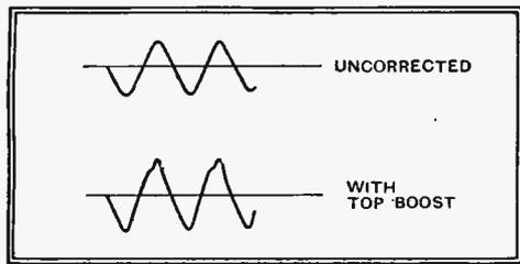
Fig. 5.—How top boost accentuates the harmonic distortion of the uncorrected waveform
