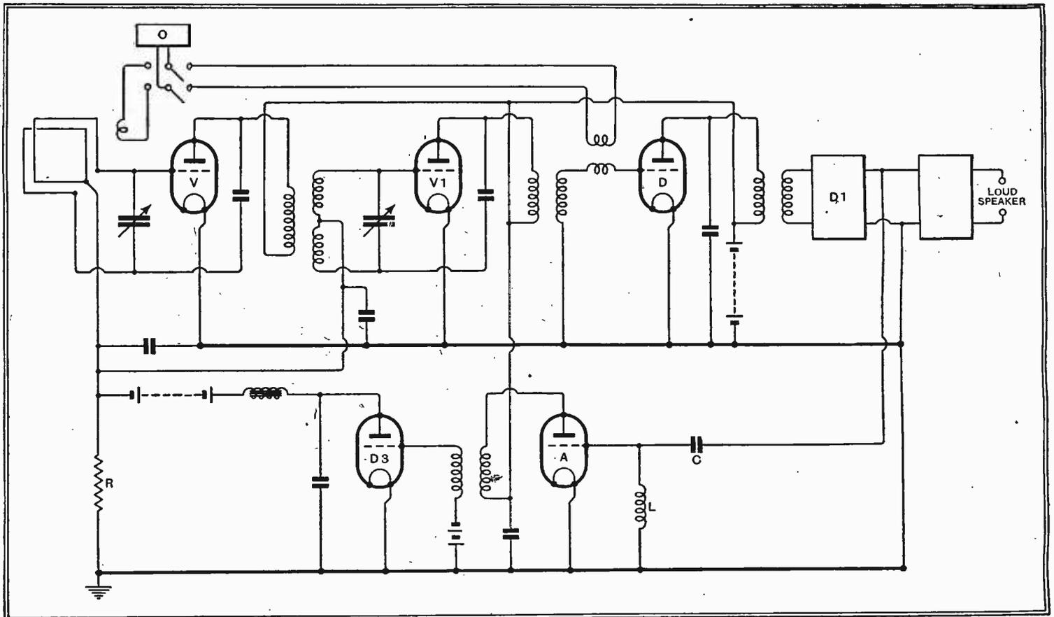
Fig. 2.—An early method of controlling the gain of an RF amplifier
