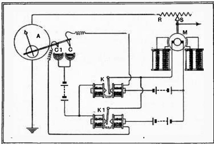
Fig. 1.—Automatic control of signal current as applied to land-line communication.
