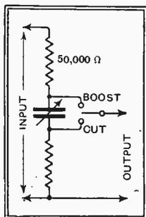
Fig. 2.—Circuit for bass control.
