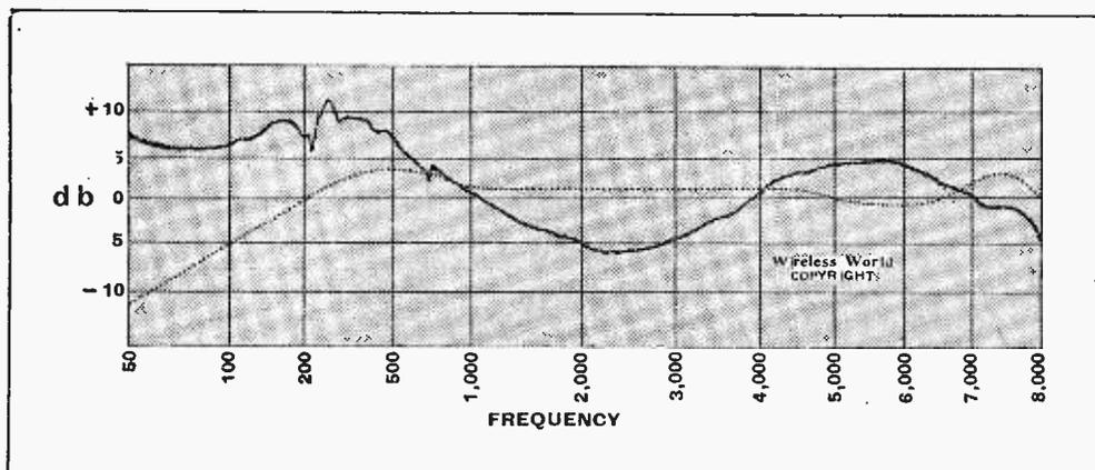
Response curve of Shure Model 99A crystal pick-up with 0.5 MΩ, shunt. Zero db is equivalent to 1 volt RMS and the dotted curve shows the characteristic of test record.
