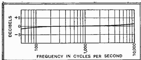
Fig. 5.—Overall frequency characteristic of amplifier.
