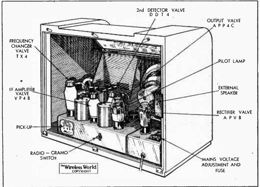
A single high-voltage pilot lamp mounted in the centre of the receiver chassis provides uniform illumination for the large rectangular tuning scale.
