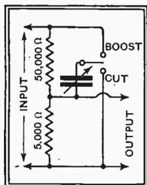
Fig. 1.—Principle of the simple tone-correction circuit discussed.
