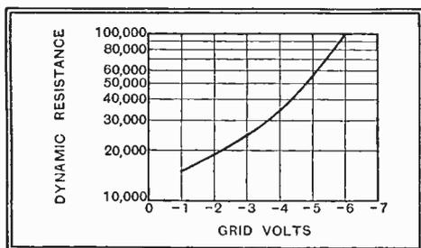
Fig. 1.—Specimen calibration curve: AC/SG valve with 90V on anode and 30V on screen.
