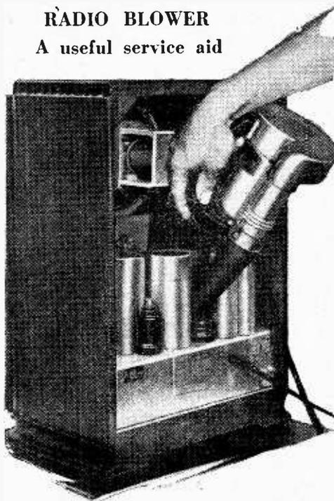
Specially designed for blowing dust out of the nooks and crannies of a receiver chassis, this American machine is fitted with an insulating nozzle of soft rubber that cannot damage delicate parts.
