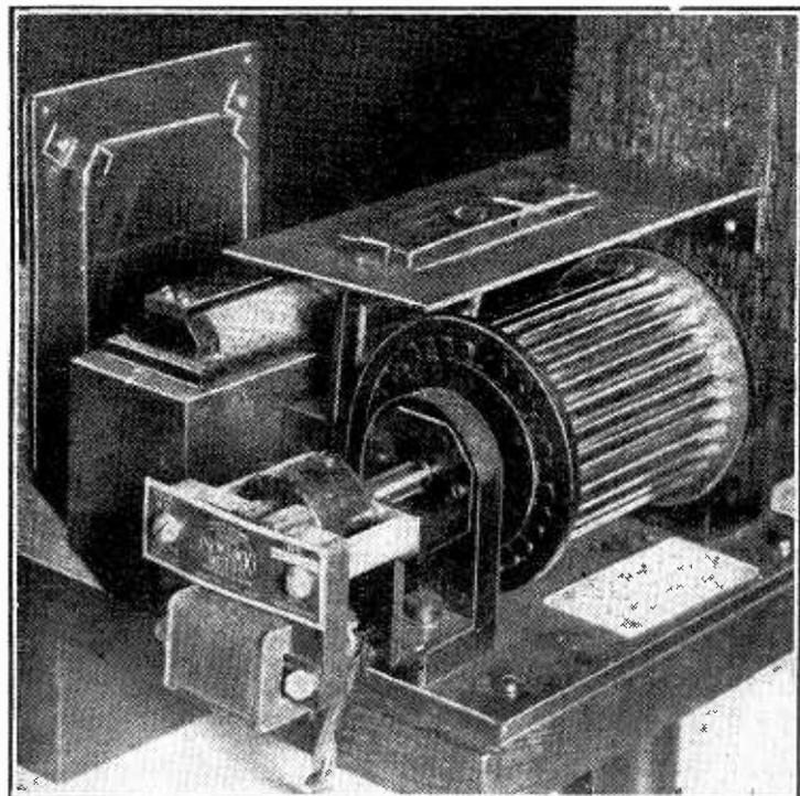
man's head with banks of photo-cells on either side, and in front of it a spot-light mirror-drum scanner. On the other side of the booth is the mirror-drum receiver. Baird have also on view a large cathode-ray tube designed for electromagnetic de-
