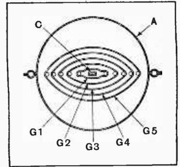
Electrode assembly for a frequency-changing valve.
