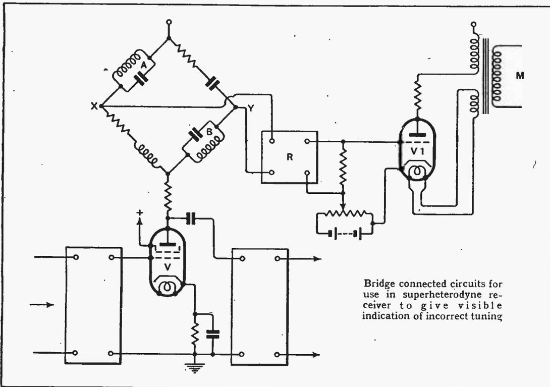
Bridge connected circuits for use in superheterodyne receiver to give visible indication of incorrect tuning
