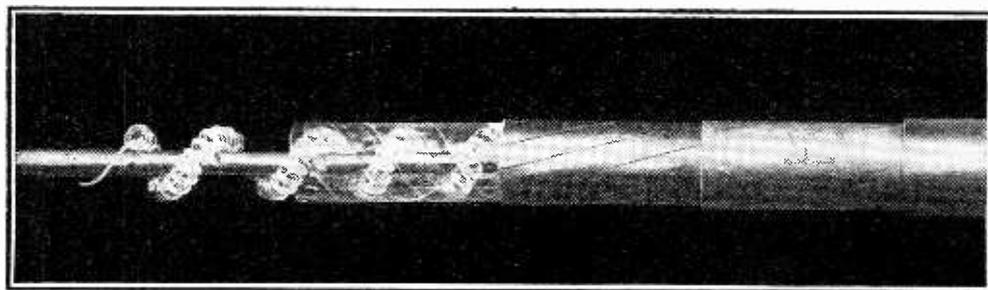
Construction of a Styroflex-insulated high-frequency cable made by the German firm of Felten and Guilleaume.
