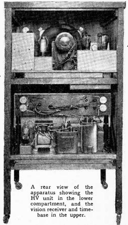
A rear view of the apparatus showing the HV unit in the lower compartment, and the vision receiver and time-base in the upper.
