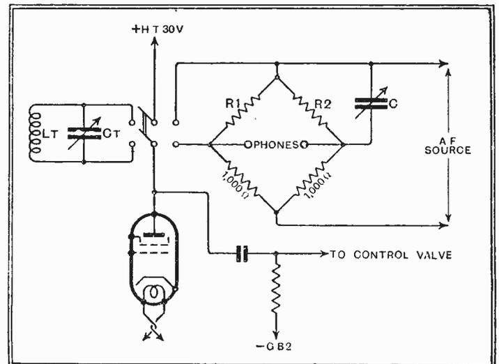
checked in a short space of time. With the switches in the positions shown, it will be seen that the circuit is essentially the same as that of Fig. 2, with the addition of decoupling RF chokes and condensers. With all the switches except S changed over to their alternative positions, the meter is ready to be calibrated. The bias on G<sub>1</sub> is under the control of the potentiometer,
