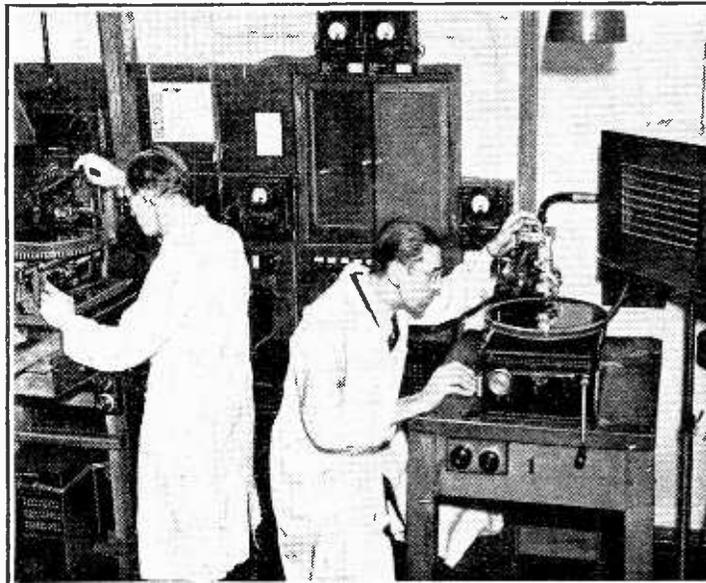
Two of the four machines used by H.M.V. for recording the Coronation ceremony and the King's speech. These were employed in pairs to minimise the chances of a failure, and to insure continuity the second pair came into operation before the first had completed a record.
