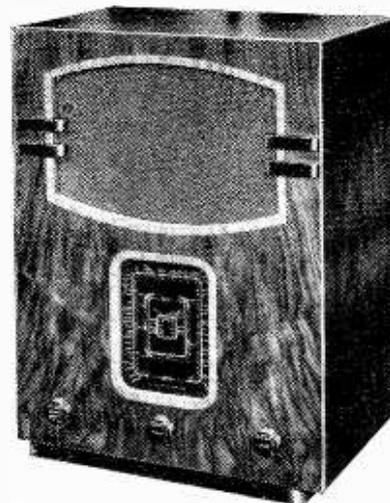
McMICHAEL MODEL 371. Coloured light bands are used as tuning pointers for the three wavebands in this new 10½ guinea McMichael AC superhet. The slow motion drive incorporates a flywheel for quick tuning, and the station names are printed in colour on a black background. Three valves and a rectifier are employed in the circuit of the set, which is available also as an AC/DC model at 11 gns.
