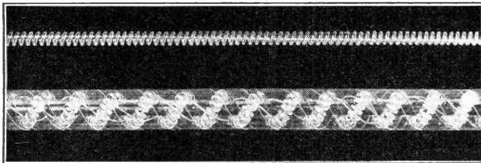
A length of the flexible Styroflex insulating material, and (below) method of winding it round a conductor in such a way as to provide insulation consisting mainly of air.
