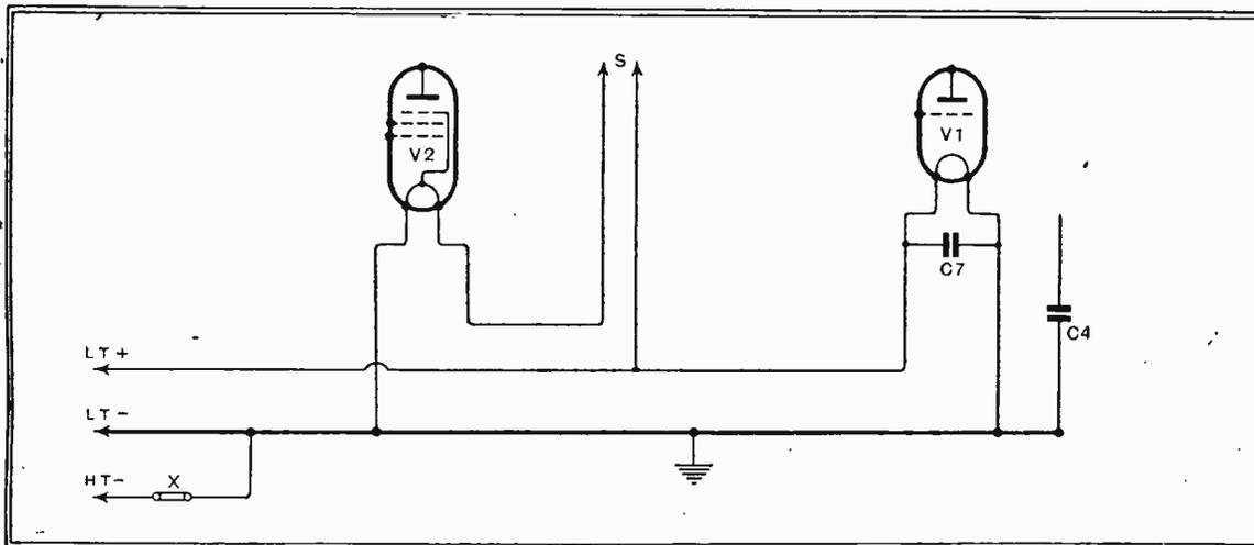
Fig. 2.—Filament wiring for battery valves; other circuit details as in Fig. 1.
