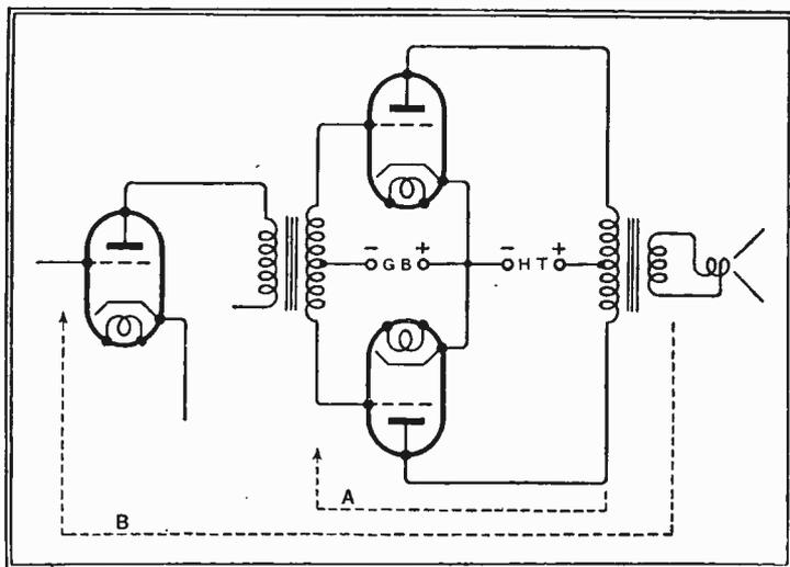
Fig. 1.—Negative feed-back may be applied across the output valves only, as indicated diagrammatically by A. But by extending its scope in both directions, as shown by B, its benefits are applied to the whole amplifier, provided that proper precautions are taken.
