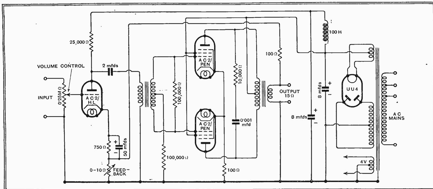
Fig. 3.—Circuit diagram of complete amplifier. With slight modifications a tone control stage giving exceptionally comprehensive adjustment of tone and, if needed, extra gain, can be added. Details will be given later.
