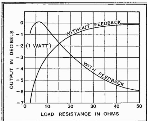
Fig. 6.—The effect of negative feed-back on the output/load resistance characteristic of the amplifier described. These curves do not take account of distortion, which is excluded by running well within the rated output.
