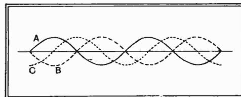
Fig. 2.—If A is a sample of the original signal applied to the amplifier, the amplified voltage fed back is connected in opposition, as shown by B. But at certain frequencies some parts of the amplifier cause a lag, and the fed-back voltage may then be represented by C, which does not have quite the same opposing effect. And if this lag is added to by further stages in the amplifier, the feed-back voltage may actually coincide with A, causing positive feed-back.
