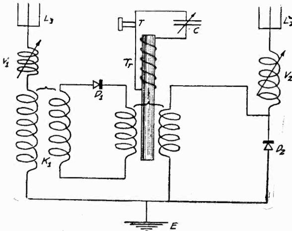
FIG. 6.—COMPENSATION OF PERIODIC STRAYS AT AUDIO FREQUENCIES.
