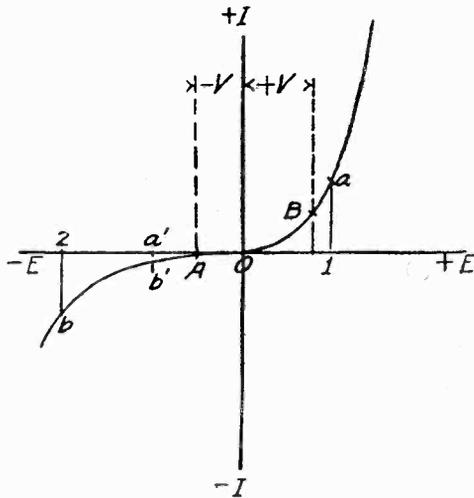
FIG. 5.—CHARACTERISTIC OF A CARBORUNDUM-STEEL DETECTOR.
