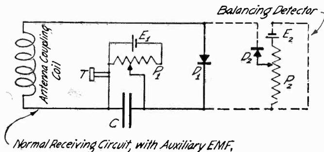
FIG. 3.—MARCONI BALANCED CRYSTAL RECEIVER.
