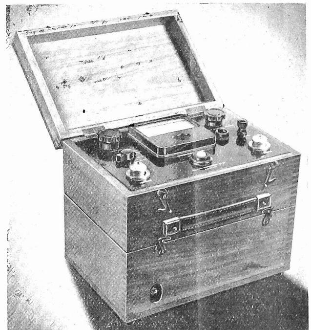
Fig. 5. Radiological type of Baldwin-Farmer electrometer
