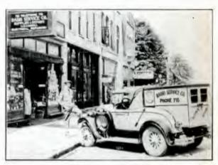
Above: The Radio Service Co., of Cleveland, employs this Chrysler roadster to render speedy service. It is equipped with a rack for carrying spare tubes, all kinds of tools, oscillators and a test set. Right behind the driver's seat an Atwater Kent screen-grid set is installed to be used for demonstration.
