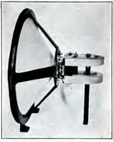
Farrand Dynamic Speaker FARRAND MFG. CO., Long Island City, N. Y. Farrand inductor dynamic speaker available in four standard inpedance values in order to match any output; chassis complete with driving unit and cone is being supplied to set manufacturers and set builders.
