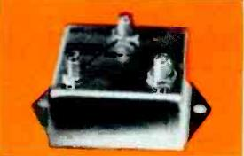
**TWO-WAY SPLITTER** 20 db isolation between outputs. Completely shielded eliminating pick-up. Matched 75 ohm input, two 75 ohm outputs. 3.5 db loss each outlet. Flush mounting waterproof container. MF-61 connectors, with three MF-59 males supplied.
