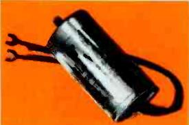
**MATCHING TRANSFORMER** Capacitors provide positive line isolation. Completely shielded eliminating stray pick-up. 72 to 300 ohms. Bandwidth 4 to 300 mcs. 6 db step-up voltage gain MF-61 input connector, spade fittings output, plus MF-59 supplied.
