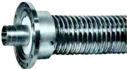
The H9-50 HELIAX is a 50 ohm cable featuring convoluted inner and outer conductors of high conductivity copper, permitting easy bending around obstructions. Type H9 is available in 1,000 foot lengths. Flanged end fittings for Type H9 mate with 6-1/8 inch EIA standard flanges and inner connectors.
