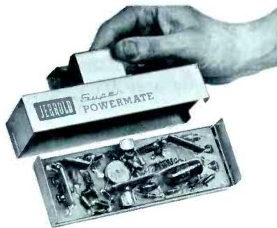
Gain-overload specifications range from 15.5 db with a maximum output of 700,000 microvolts at channel 2 to 11.1 db with a maximum output at channel 7, to 11.3 db with 200,000 microvolts maximum output at channel 13.
