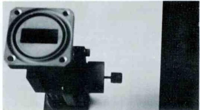
Business end of 12kMc waveguide showing choke joint flange.
