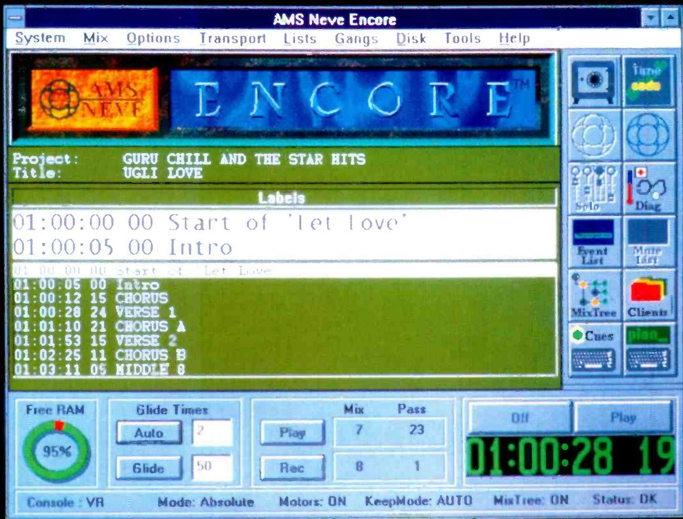
**P**ROBABLY. AMS Neve is introducing ENCORE™, a powerful new automation system. Encore uses a Pentium Processor, runs under Windows NT and combines the best innovations of AMS Neve's automation packages.
