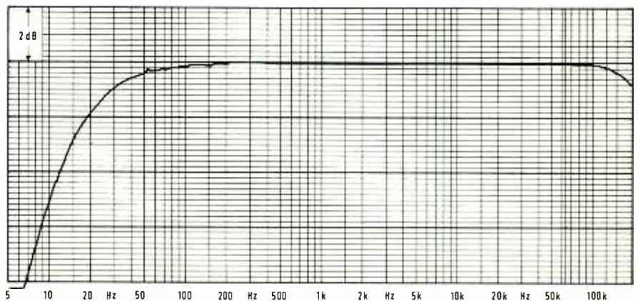
FIG. 2 dbx 902 DE-ESSER FREQUENCY RESPONSE WITH DE-ESSING
