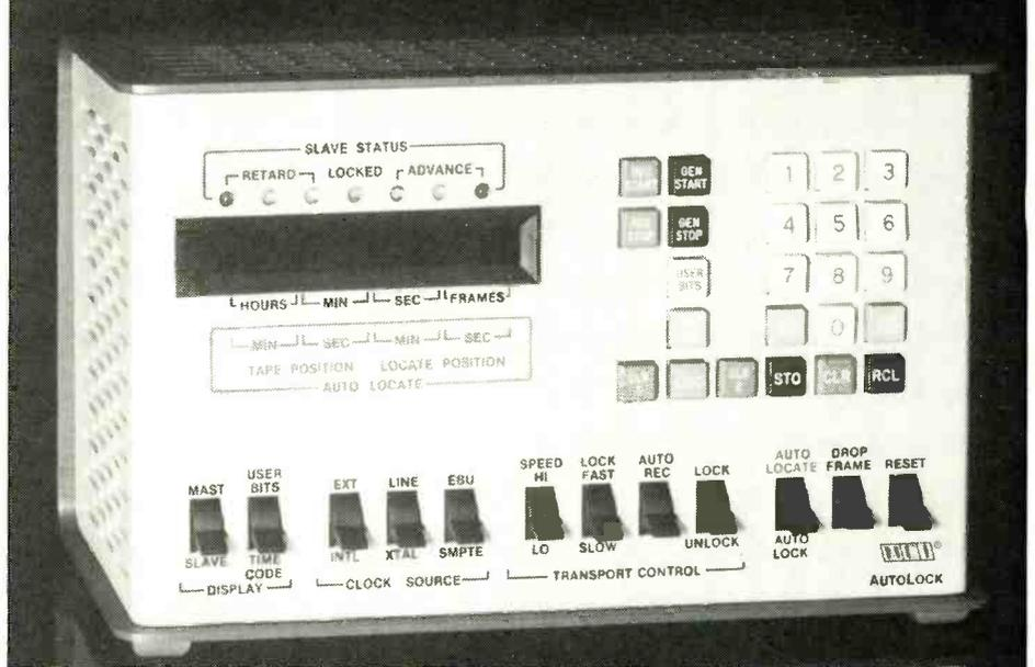
units to video machines for parallel sound editing. Sync interlock, including still, is achieved by the use of VITC recorded on two picture lines and read by the revolving head drum of the video recorder. Other features include automatic changeover to phase locked sync at sound speed and use of CTL pulse from the VTR control track to ensure interlock in the event of poor timecode reading. Interfaces available for JVC and Sony *U-matics* and many tape machines.
