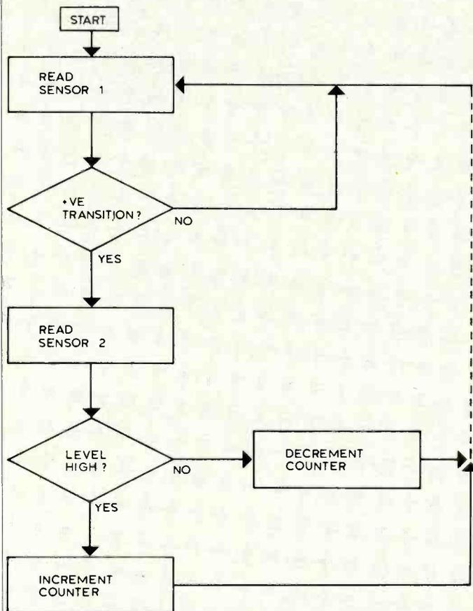
FLOWCHART FOR SOFTWARE DERIVATION OF DIRECTION SENSING
