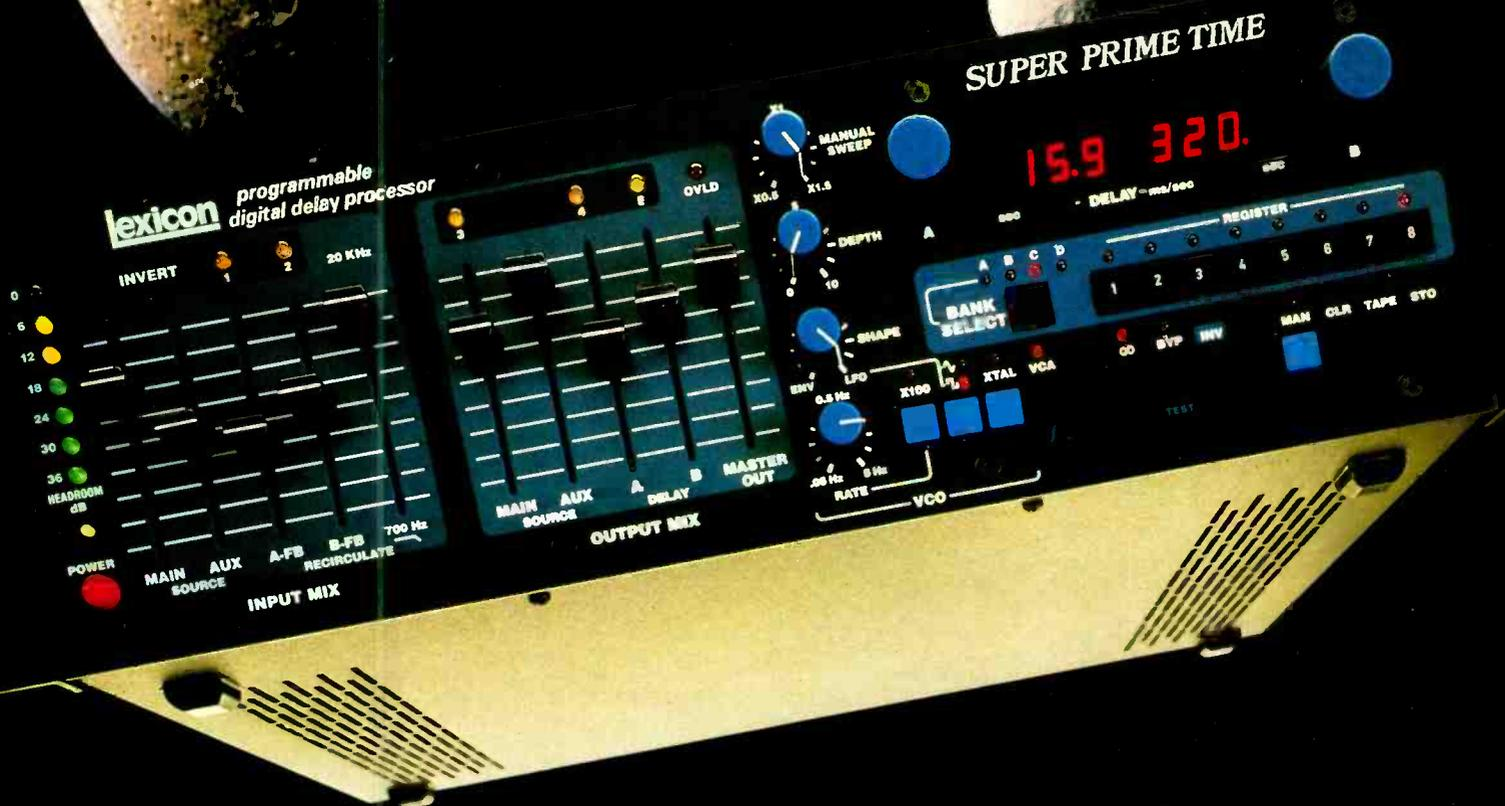
The Super Prime Time is the first micro-processor-based special effects device and audio processor which enables you to create, store and recall effects for any piece of music live or in the studio.
