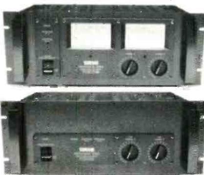
\*The PC2002 is identical to the PC2002M but without the twin Peak Output meters.
