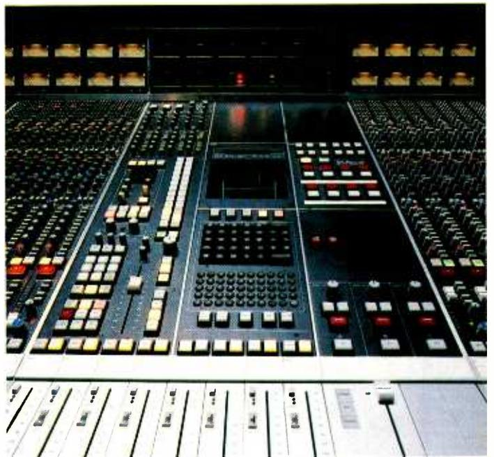
In live production, the SSL Real Time System enables complex sequences of all channel and group fades and cuts to be pre-programmed, and then manually executed with a single set of controls.
