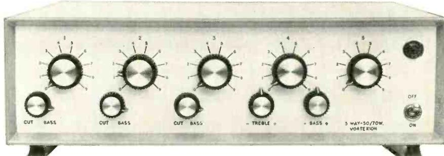
THIS is a high fidelity amplifier with bass cut controls on each of the three low impedance balanced line microphone stages and a high impedance (1·5 meg.) gram stage with bass and treble controls, plus the usual line or tape input. All the input stages are protected against overload by back to back low self capacity diodes and all use F.E.T.s for low noise, low intermodulation distortion and freedom from radio breakthrough.
