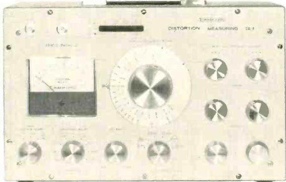
A sensitive instrument for the measurement of total harmonic distortion, designed for speedy and accurate use. Capable of measuring distortion products as low as 0.002%. Direct reading from calibrated meter scale.
