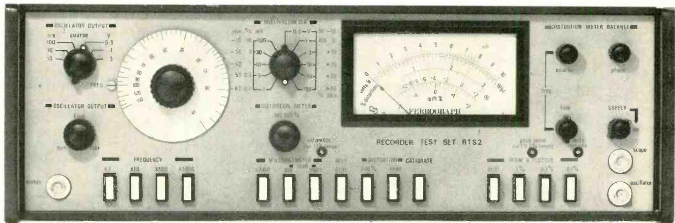
The RTS2 combines a millivoltmeter, distortion meter, peak to peak wow & flutter meter, and audio generator.
