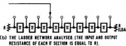
FIG. 8 EQUIVALENT CIRCUIT FOR A 600 OHM LADDER FADER AT MINIMUM ATTENUATION SETTING
