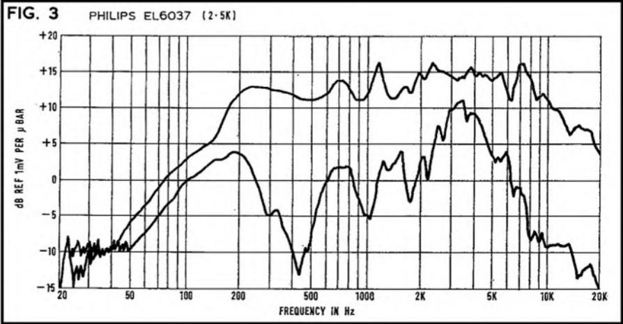
show the free field sensitivities of both these microphones. They are substantially similar, the differences in the back response of the two microphones being due to normal manufacturing tolerances. The response is flat from 200 Hz to 10 kHz, and the usable response is from 100 Hz to 20 kHz.
