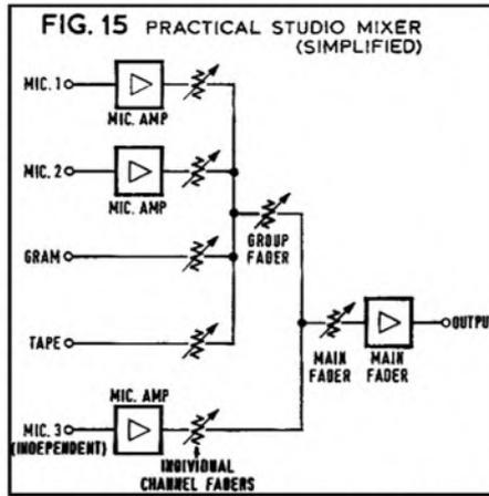
to allow each source to be controlled by any group fader.
