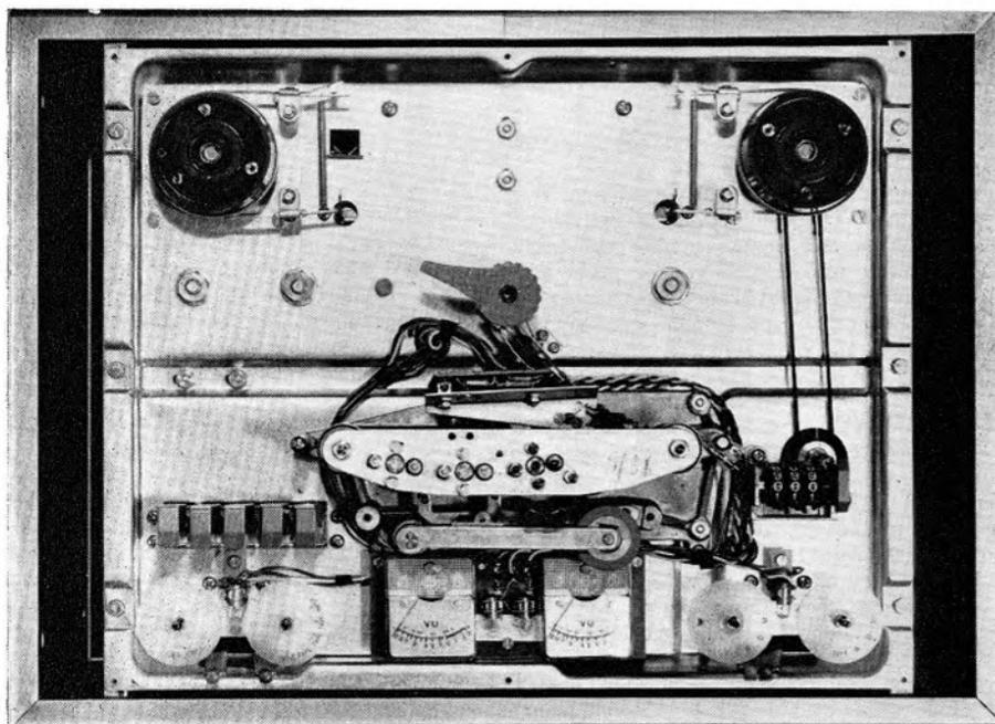
If neglect is the basic cause of trouble, the solenoids may be sluggish, and more than once this has led to replacement when all that was needed was cleaning and thorough lubrication. The slug must slide freely, and can be removed, cleaned with spirit, with the barrel similarly treated, and then reassembled with a smear of Moly slip. As with all lubrication, a little in the right place is the secret, not liberal application.
