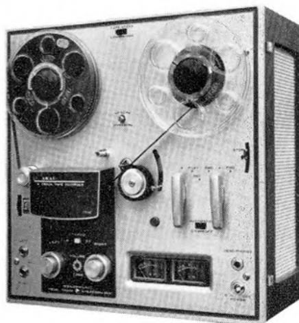
THIS is the standard Akai deck, this time with a switched-pole motor to give a 2:1 change of speed and a slip-on capstan sleeve to provide a further 2:1 increase covering 19, 9.5 and 4.75 cm/s.
