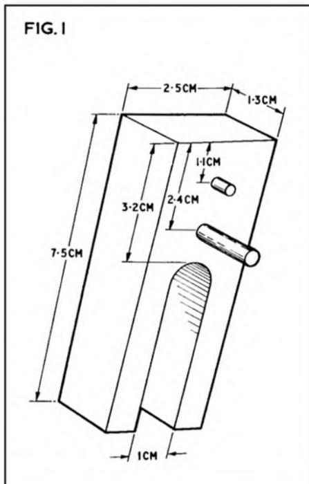
clamps the tape against the spool centre while two turns of the spool are made by using the device as a handle. It is essential while turning the take-up spool also to turn the feed spool in order to keep the tape slack. As the diameter of the steel peg is very small, the threader can easily be removed.
