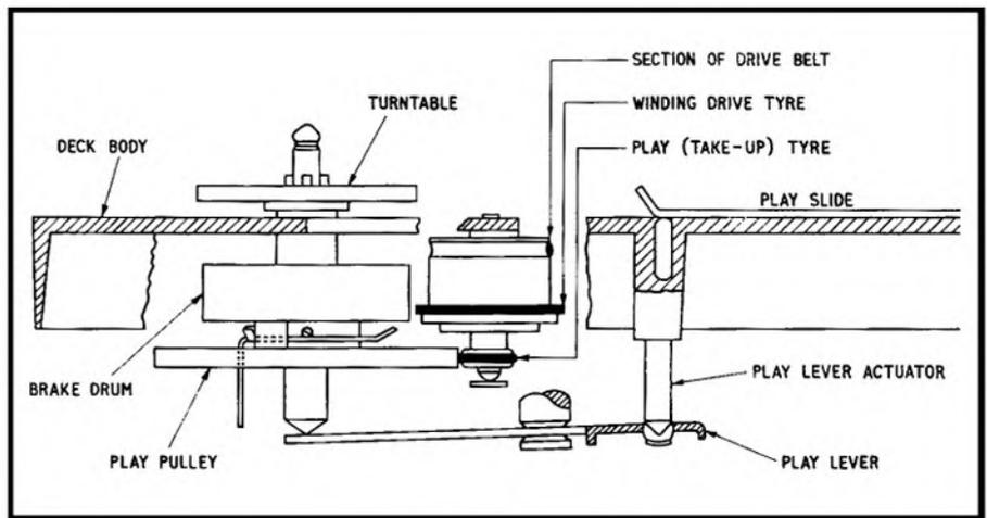
Fig. 8. Ampex 753 arrangement.
