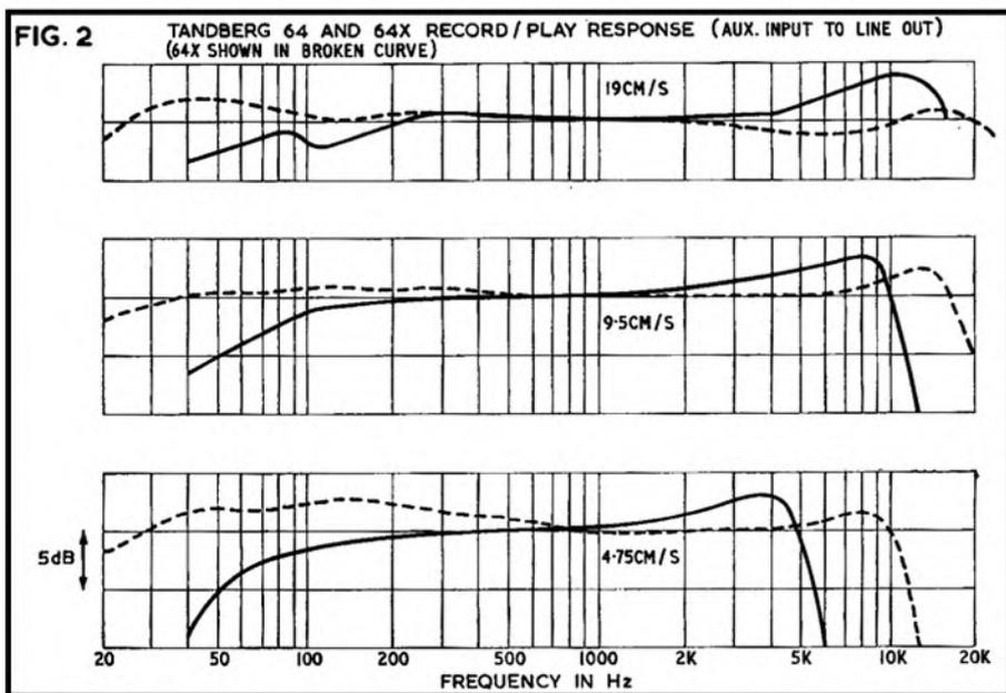
Readers interested in precise figures might care to note the following taken at 15 kHz, 0 dB at 1 kHz being adjusted to suit each tape. BASF LH +7 dB. Philips SP.18 +5 dB. BASF LGS35 +4.5 dB. Zonatape +3.5 dB. Agfa +3 dB. The latter Agfa tape was brand new and measured during its first run. When tested after re-spooling, it rose to +4.5 dB. These 15 kHz figures were all about 3 dB lower on the other channel.
