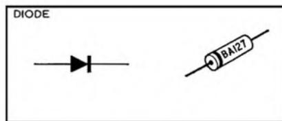
garden stone (don't cut the cat, a true whisker wouldn't really work). Such fiddling is unnecessary today since *germanium diodes* may be purchased quite cheaply with wire and crystal sealed inside a plastic container—similar in *size* and *shape* to a resistor. The diode has certain characteristics in common with the transistor and it is no coincidence that the circuit symbol is similar.
