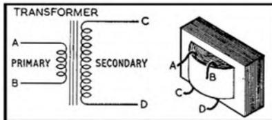
(pendulums once more) electricity inserted at the *primary* cause another current to be *induced* into the *secondary* coil. The process itself is called *electromagnetism*. Transformers are often specified by the ratio of wire turns
