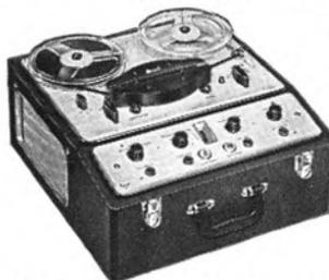
Mono — half track — three heads — recording level meter — separate amplifiers, record and playback heads — frequency response 25-26,000 c/s ± 3dB — power output 2 watts r.m.s.
