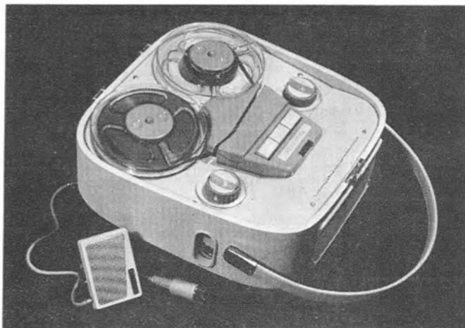
Complete with dual impedance mike 200/50K; 1,200' TP tape; empty  $4\frac{1}{4}$ " spool; Radio lead; batteries; circuit; and instruction book. Headphones/Stet, spare plug, head cleaning kit.
