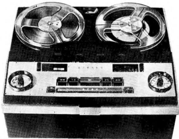
Transistorised input stages allow mixing of microphone (0.1mV. at 200 ohms), radio (10mV. at 100K) and pickup (200mV. at 1 Meg.). The remaining circuitry is valve.
