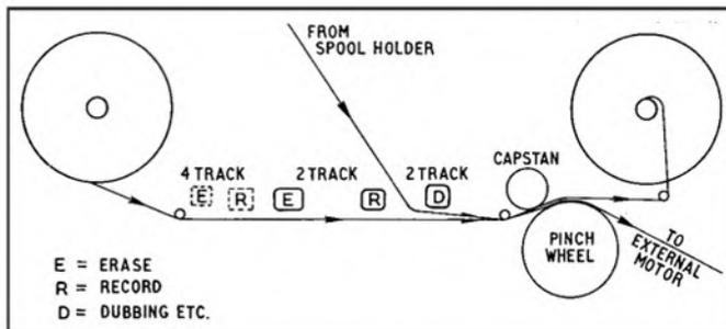
Superimposition: it is necessary to provide an alternative load for the oscillator when disconnecting the erase head. A 1.5 K resistor would be suitable, with a single-pole, double-throw switch to select either the erase head or the shunt resistor.
