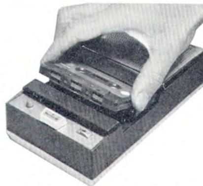
Frequency response: 120 c/s to 6 Kc/s ± 3 dB. Signal-to-noise: better than 40 dB. Rewind time: 70 seconds. Dimensions (in leather carrying case): 8¼ x 6½ x 2½ in. Cabinet Dimensions: 7¼ x 4¼ x 2½ in.
