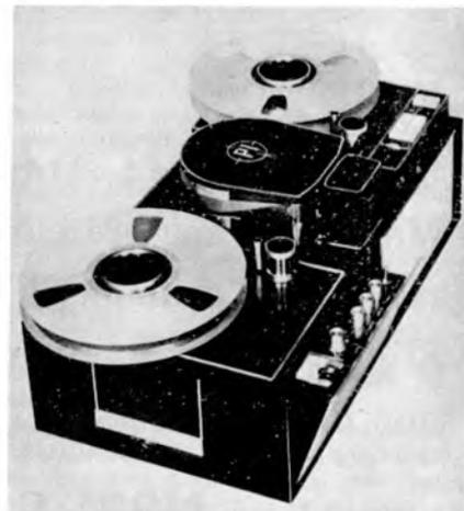
playing time of 115 minutes on a 10½ in. spool of one-inch tape. Tape speed is 6.25 i/s and, weighing only 68 pounds, the recorder is the lightest on the market and can be lifted by one man. *Continued on page 355*
