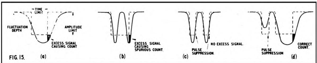
Fig. 15: Operation of discriminator, and effect of pulse suppressor: (a) Normal, correct counting condition. (b) Spurious counting condition caused by double fluctuation with no pulse suppression. (c) Spurious count eliminated by suppression. (d) Correct count allowed, with suppression.
