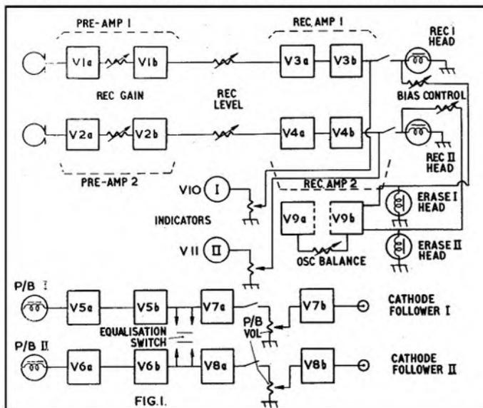
to the recording amplifiers. The two playback amplifiers are three-stage units with switched equalisation, operated by the speed-change control, between second and third stages, a variable level control from each feeding the cathode-followers. Both the Record-Level and the Playback-Volume controls are dual potentiometers.
