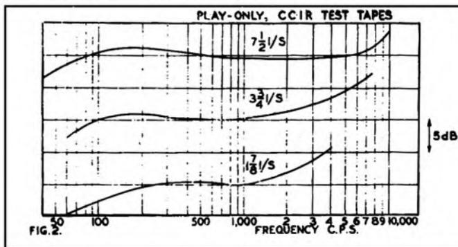
recommendation at  $7\frac{1}{2}$  i/s, but that the high note response is over equalised at the two lower speeds. A high note roll-off will be required in any external power amplifier if C.C.I.R. tapes are to be played on this recorder, and an even more vigorous top cut will be needed to reproduce N.A.R.T.B. recordings satisfactorily.
