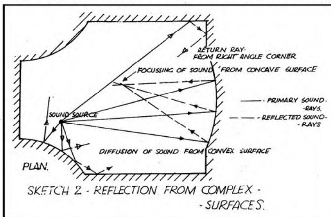
plans and sections, and setting on these drawings a diagram showing the sound source, the listeners, and the various direct and indirect sound paths between them.
