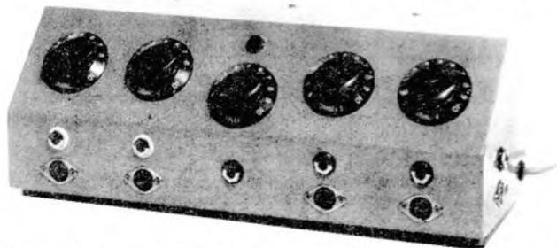
inputs are high impedance, and the output impedance is 600 ohms, up to 200 mV, suitable for gram input of a tape recorder. The model has two high-level and two low-level inputs and built-in power supply. The mixer is manufactured and distributed by Esisolder Iron Company Ltd., 98 Dominion Road, Worthing, Sussex.
