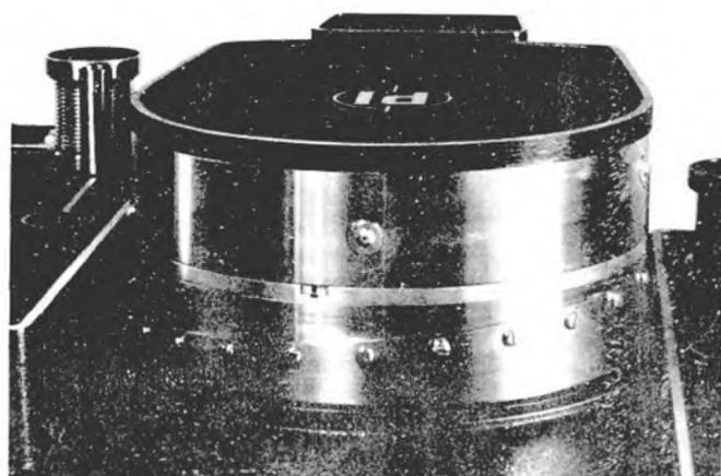
The helical scan head assembly which forms the heart of the PI-3V video recorder
