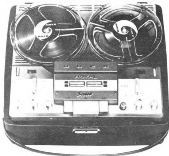
The specification supplied gives the following frequency response figures 50:20,000 c/s, 7½ i/s: 50-16,000 c/s, 3½ i/s: 50-8,000 c/s, 1½ i/s: 50-4,000 c/s, ½ i/s. Wow and flutter figures are claimed to be 0.15% at 7½ i/s. The power output is 2 watts per channel. Dimensions of the Royal Stereo are 15 × 14 × 7 in. Price £141. 15s. **Distributors are Bosch Ltd., 205 Great Portland Street, London, W.1.**
