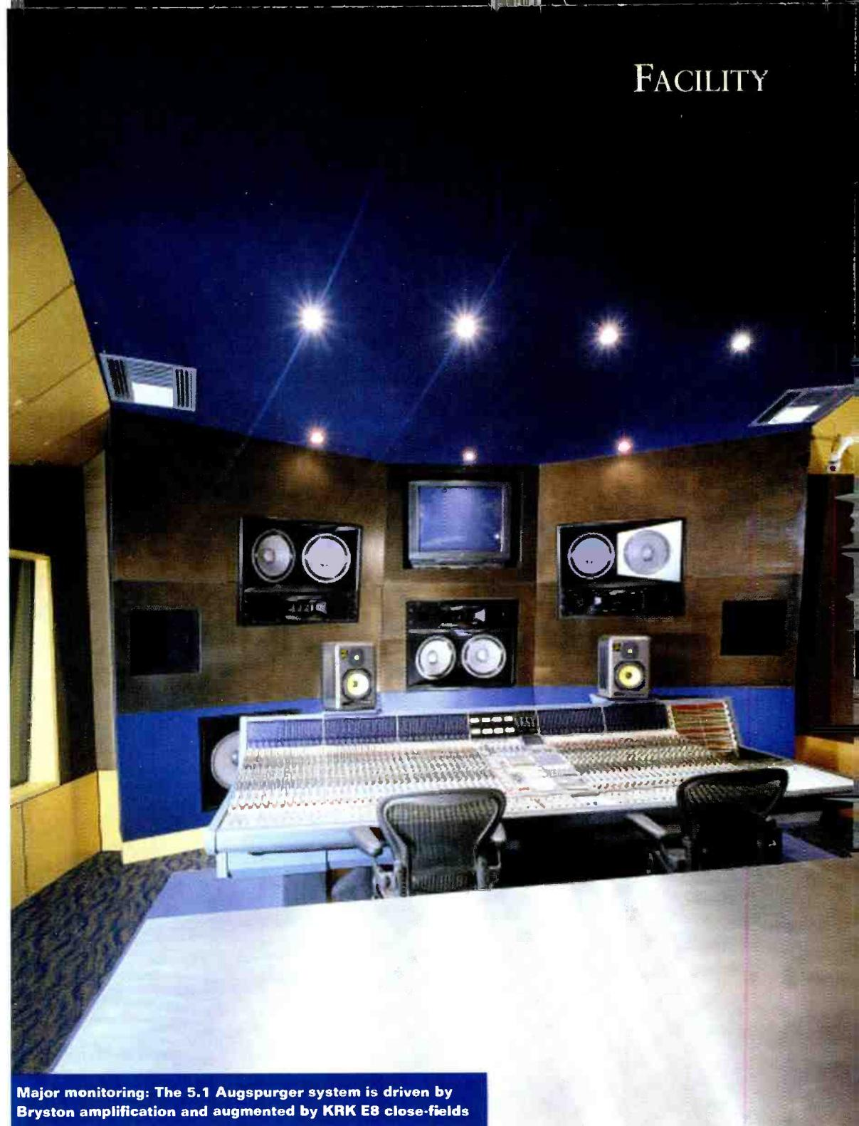
**Major monitoring:** The 5.1 Augspurger system is driven by Bryston amplification and augmented by KRK E8 close-fields
