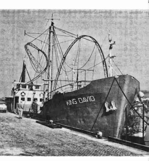
The Capital Radio ship back in Ijmuiden Harbour with a hopelessly twisted antenna damaged during the lowering operation at sea.
