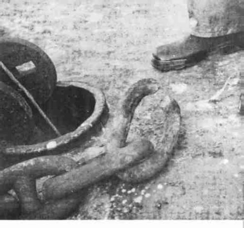
The link that broke . . . in the 'new' anchor chain.
