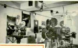
Newsreels and other short movie subjects also make excellent television program material. Sound film is run through these projectors. Pictures are projected onto the "Iconoscope" of the cameras in the next room for transmission.
