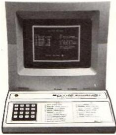
automatically determine both the baud rate and polarity of the received signal. The combination of automatic decoding and simplified tuning make this system particularly attractive to the newcomer. If the letters I receive are a fair reflection of the problems experienced by new listeners, the EasyReader's Smartlock should prove extremely popular.
