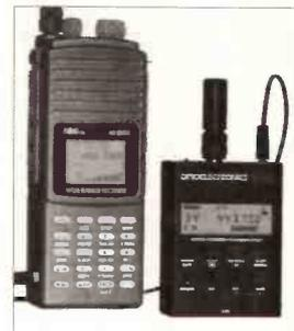
The most innovative product for scanners of 1995? Connect this little frequency counter up to your AR-8000 and see it make the scanner jump onto a
