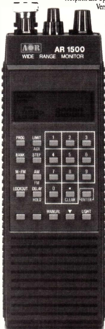
Versatility is excellent. The AR1500 may be powered from its internal NiCad pack, spare dry batteries may be carried for extended operation and used with the dry battery case, the set may also be plugged directly into the cigar lighter socket of a motor vehicle (external input range 11 - 18V DC).
