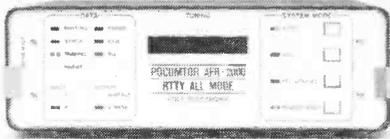
**THE POCOMTOR AFR-2000 CW-RTTY ALL MODE DECODER** allows the simple and easy decoding of CW — RTTY — ARQ — FEC & ASCII (including 200 baud press services), FEC Collective & Selective modes.
