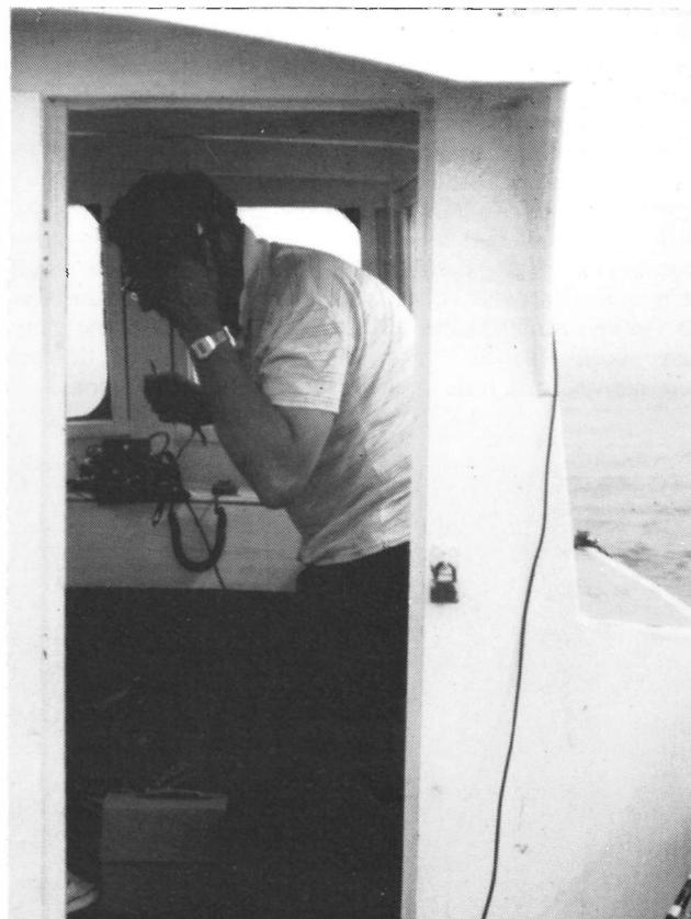
Bernard Atkinson operating G6EBH/MM in the wheelhouse of his diesel vessel *Prospect*. The transceiver is a Yaesu FT-290R with muTek front end. A Daiwa 30w amplifier is used with an HB9CV antenna for SSB and a 1/4-wave vertical for FM/repeaters. The boat is 22ft. long and 8' -6" beam with a 12 1/2 h.p. main engine and a 7 1/2 h.p. auxiliary. Listen for G6EBH/MM on summer weekends and sometimes on Wednesday afternoons from AO square on 2m.
