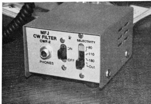
The MFJ Filter with a mini-LED between the two top screws on the front panel.
